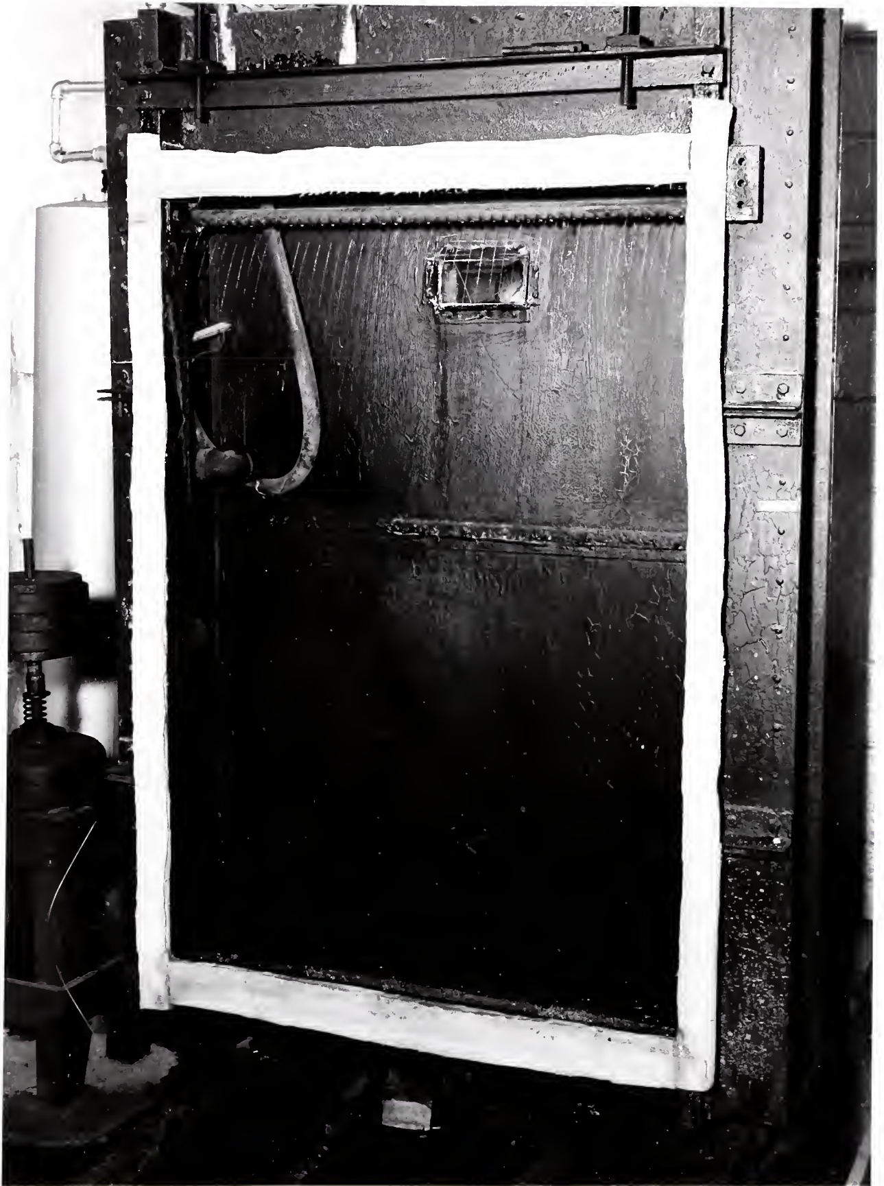
Fig. 3 - Permeability test chamber, showing method of applying water to the wall face.
