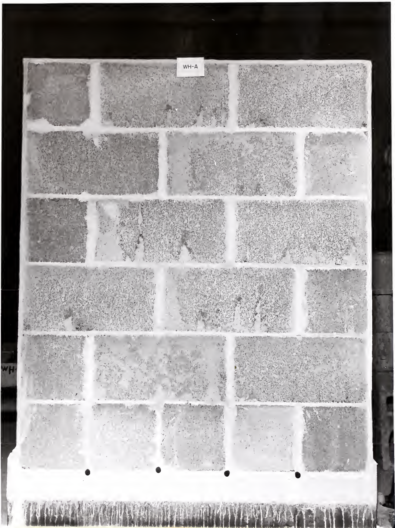
Fig. 2 - Front elevation (exposed face) of wall A, showing weep holes.
