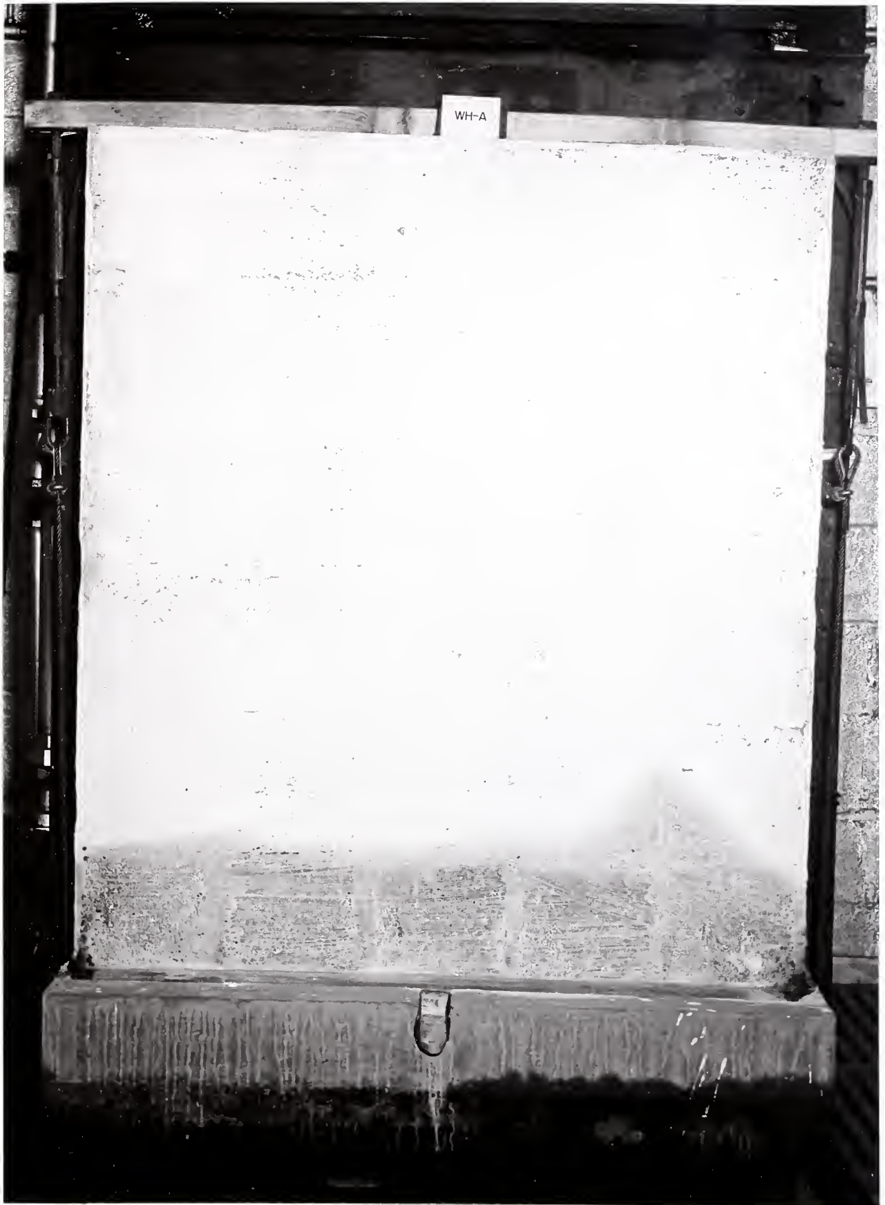
Fig. 7. - Wall A after test A-7, pressure head of 3-in.
