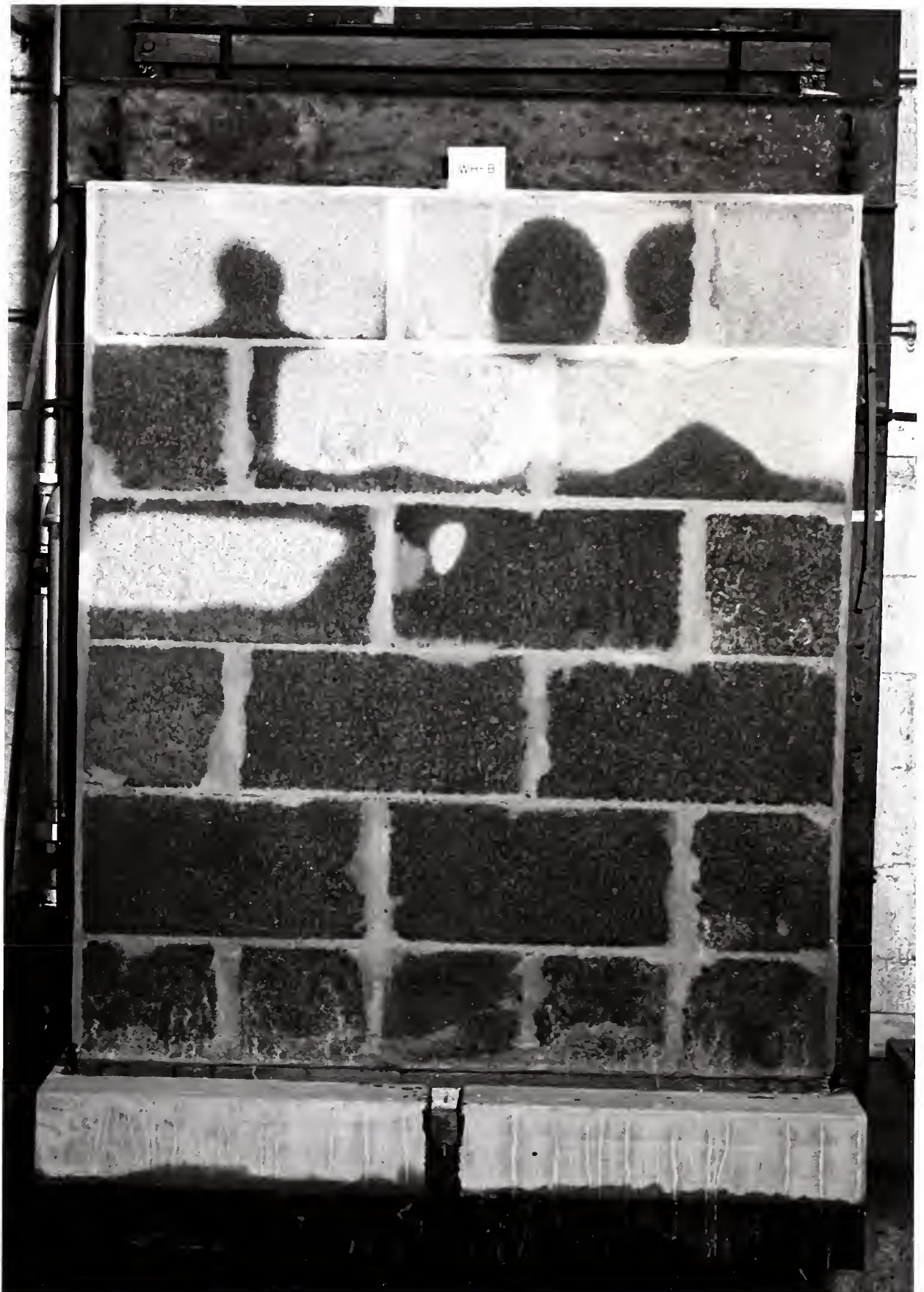
Fig. 4 - Back of wall B after test B-2; exposed face not painted, weep holes open, pressure head of 3-in.
