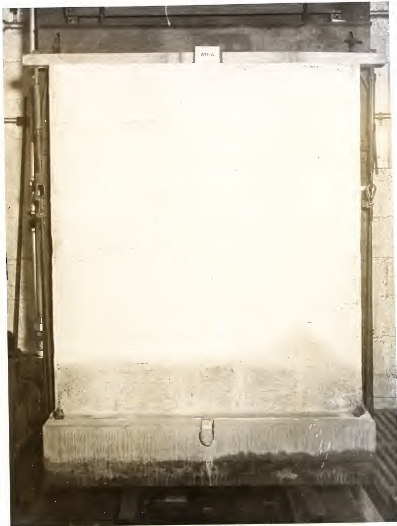
Fig. 6 - Wall A after test A-6; pressure head of 2-in.
