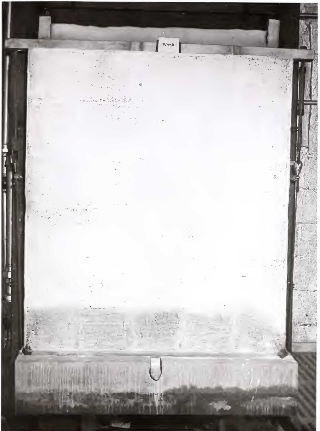
Fig. 5 - Back of wall A after test A-5; face painted, back whitewashed, weep holes open and pressure head of 1-in.
