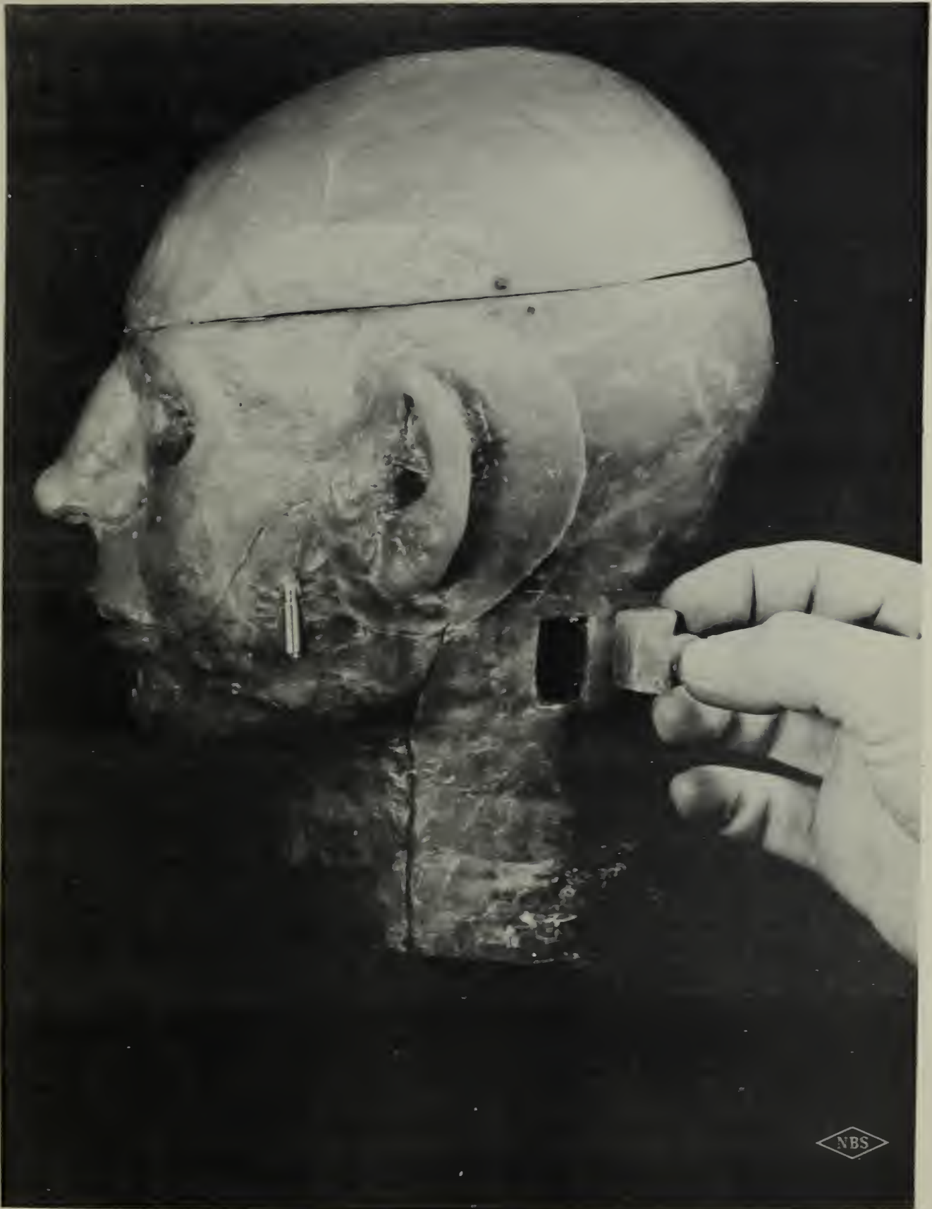
Figure 3. Wax phantom showing placement of ionization chamber at skin of cheek and recessed location for measurements in region of neck lymphatics.
