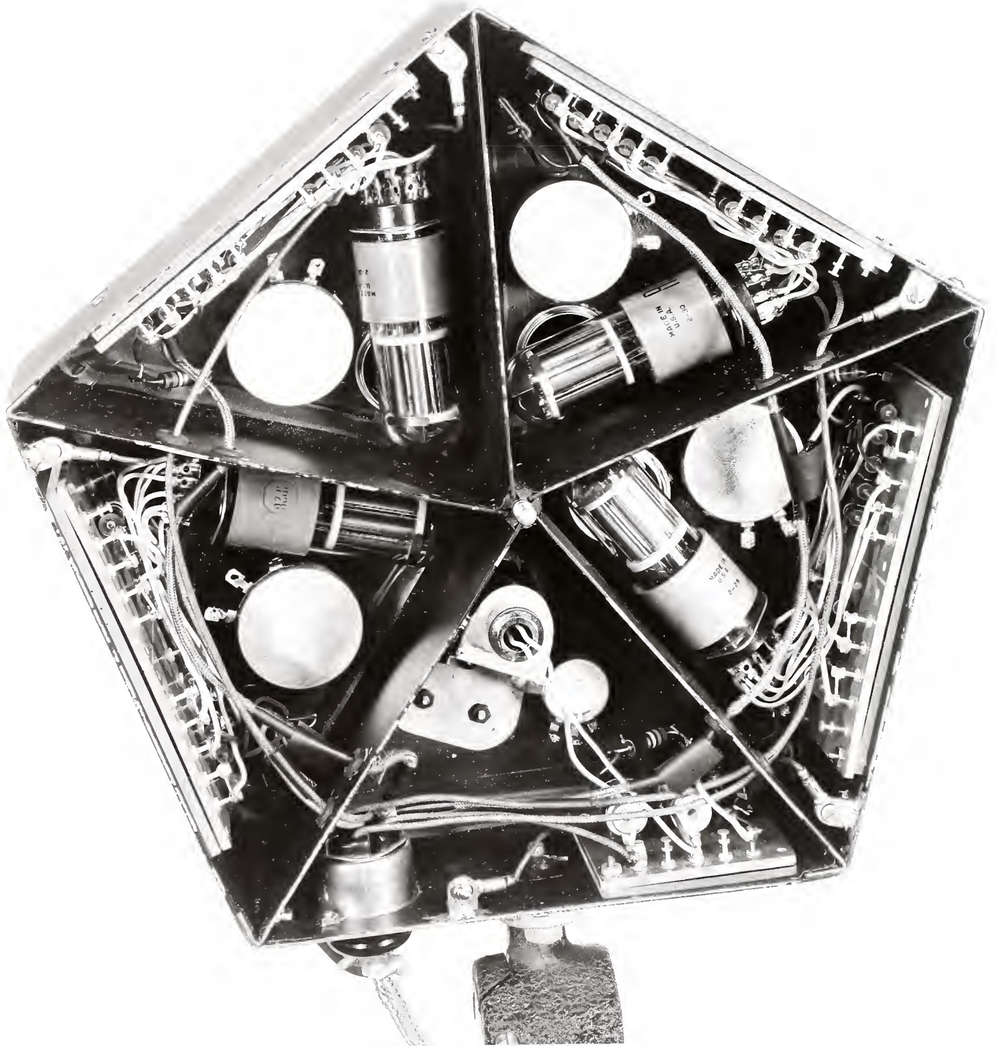
FIG. 6 SPECTRORADIOMETER RECEIVER, REAR VIEW OF INTERIOR
