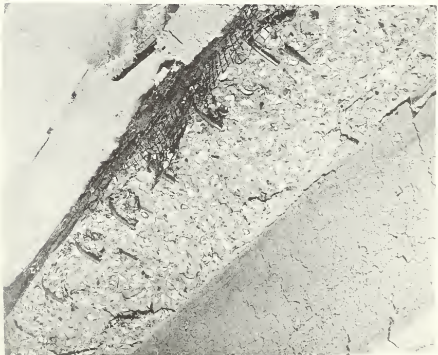
FIG. 15 REPRESENTATIVE SPALLED AREA (SLAB) FROM TEST OF A: \frac{4}{5} :1 BEAM
