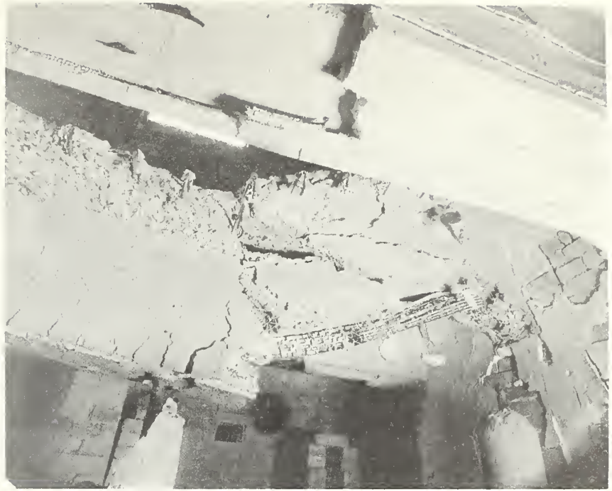
FIG. 16 NORTH HALF OF A:4/5:1 BEAM AFTER FIRE TEST 334 AND RELOADING TEST
