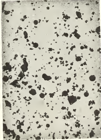
LOW CARBON FLY ASH X 80
