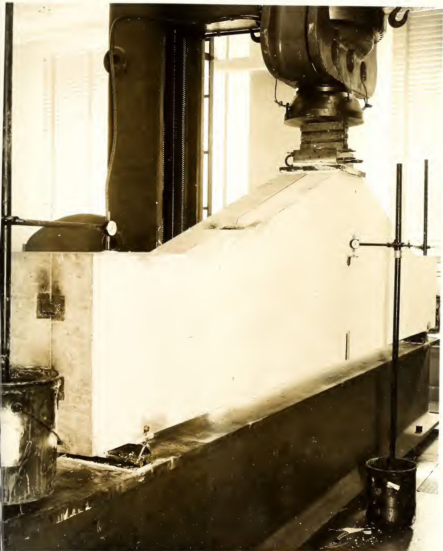
Fig. 6. View of Tee-Head in testing machine.
