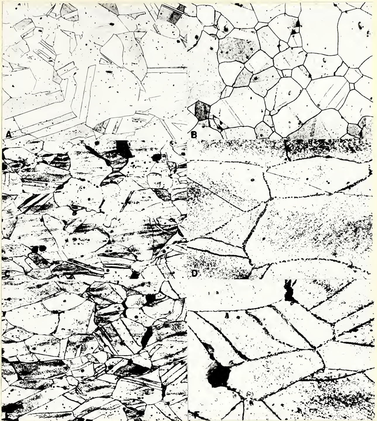
Figure 1. Structure of the steel as annealed and after testing at 1350°F to rupture. Longitudinal sections. Etched in 5 parts HCl (conc.) and 2 parts chromic acid (10%).
