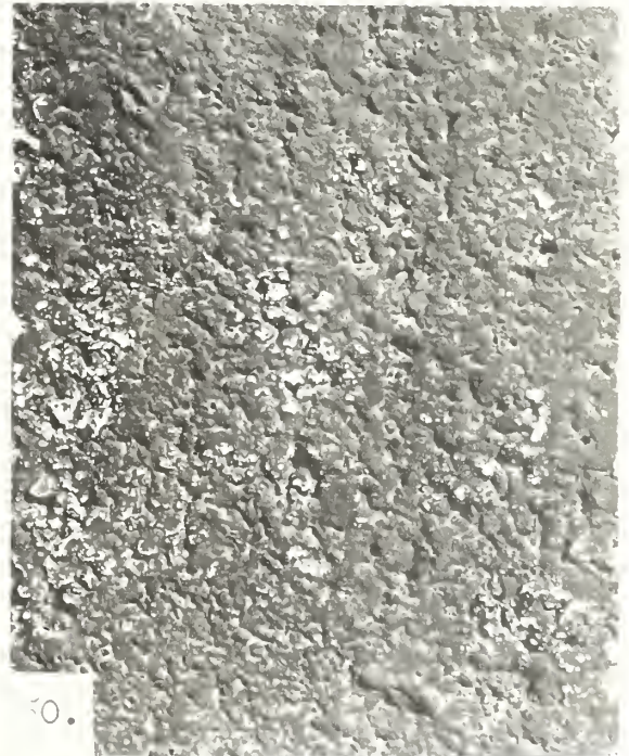
Figure 7. Class I coatings on cinder block - 2 years outdoor exposure.
