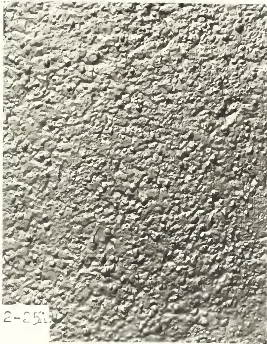
Figure 12. Aluminum paint (coating no. 23) applied to various base coats on cinder block - 2 years outdoor exposure.
