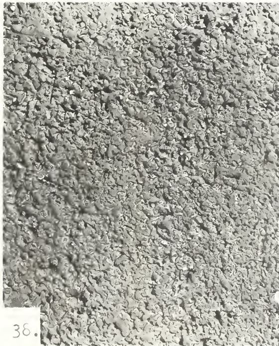
Figure 11. Class III coatings on cinder block - 2 years outdoor exposure.
