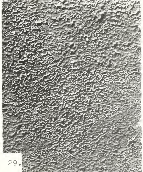
Figure 6. Class I coatings on cinder block - 2 years outdoor exposure.
