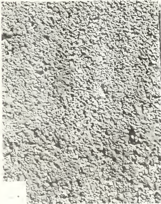
Figure 3. Class I coatings on cinder block - 2 years outdoor exposure.
