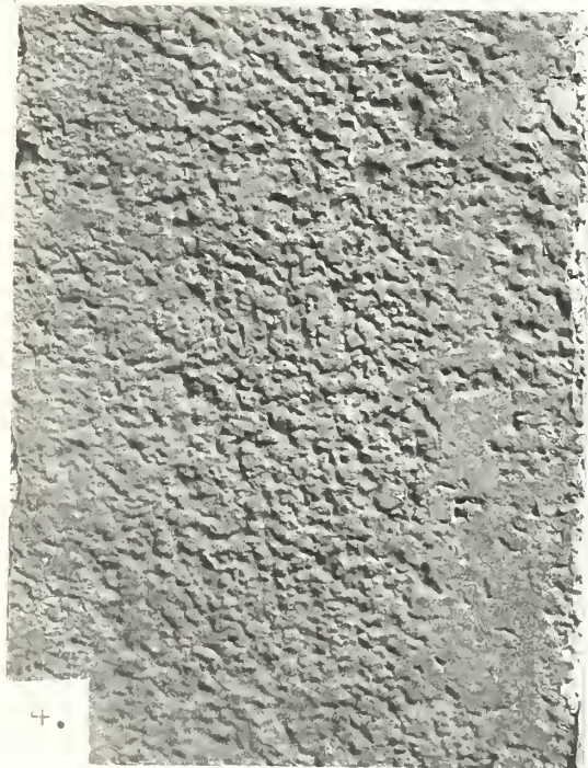
Figure 9. Coatings on cinder block - 2 years outdoor exposure. 56 & 59, Class I coatings; 4 & 5, Class III coatings.
