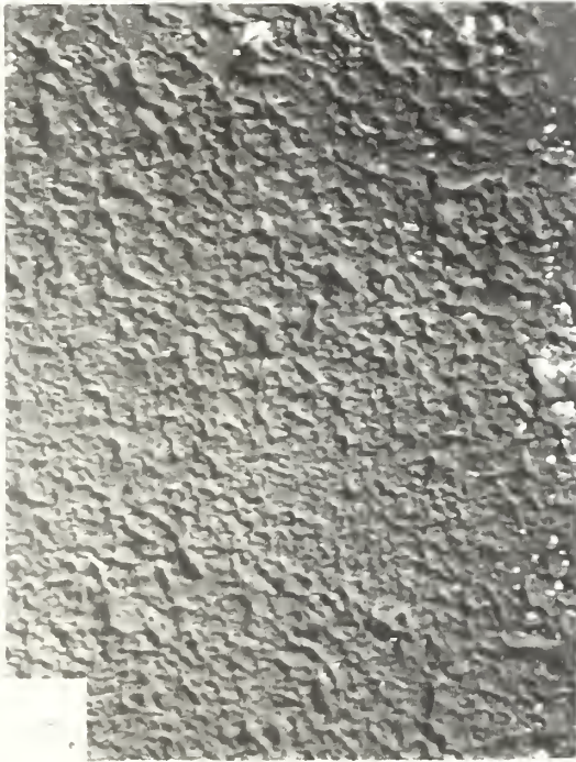
Figure 10. Class III coatings on cinder block - 0, 10, 20, 25 years outdoor exposure.
