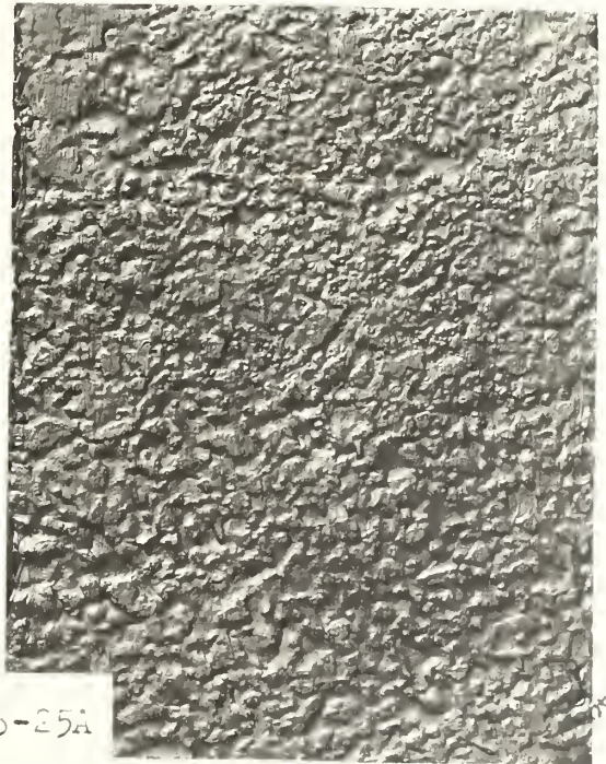
Figure 12. Aluminum paint (coating no. 23) applied to various base coats on cinder block - 2 years outdoor exposure.
