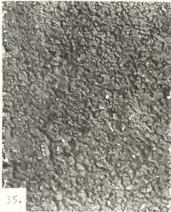
Figure 7. Class I coatings on cinder block - 2 years outdoor exposure.
