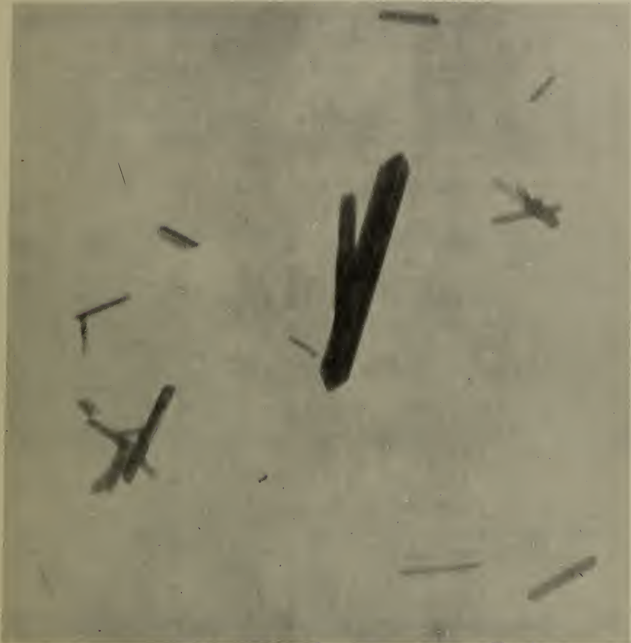
Fig. 4. Electron micrograph of tricalcium phosphate hydrate treated for seven days at 300° C in a hydrothermal bomb. Magnification 25,000 diameters.
