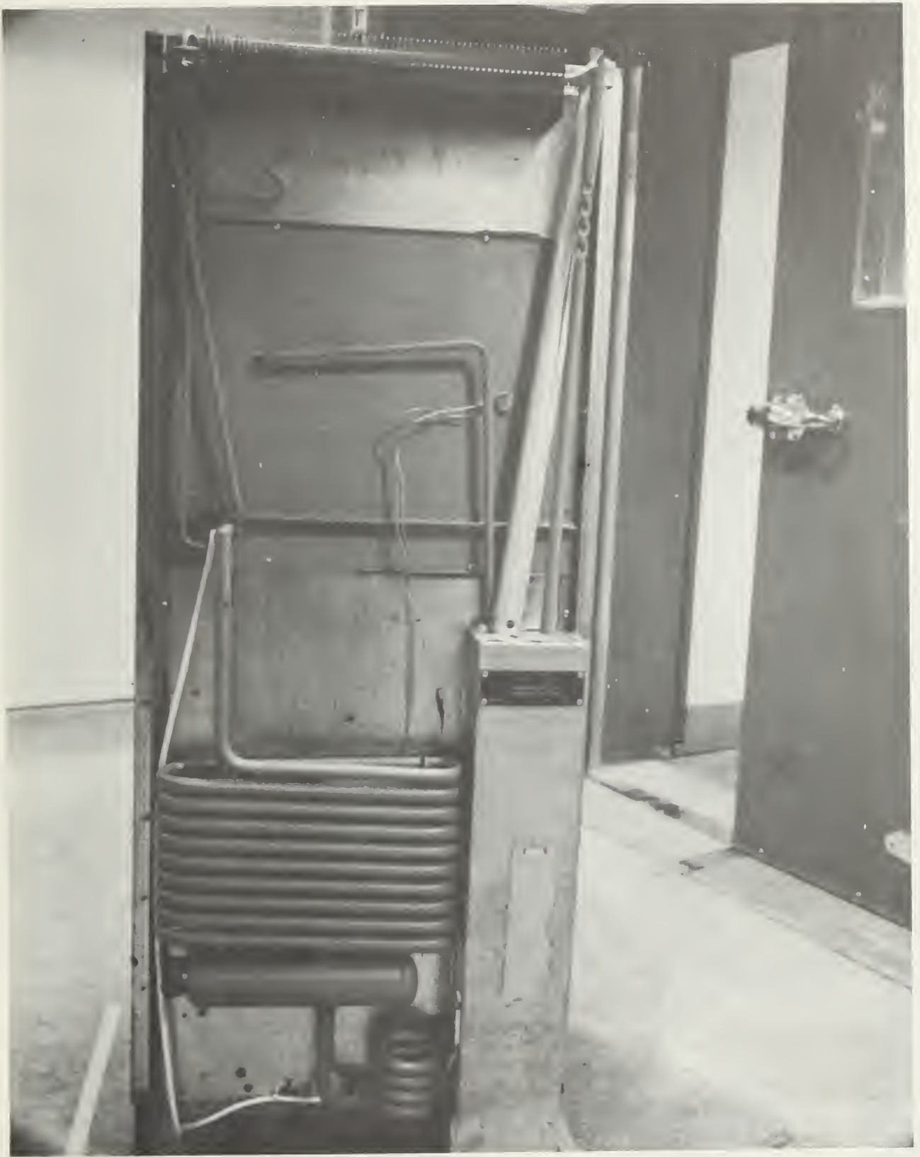
Figure 2 Absorption cooling system, back view of S & S refrigerator.
