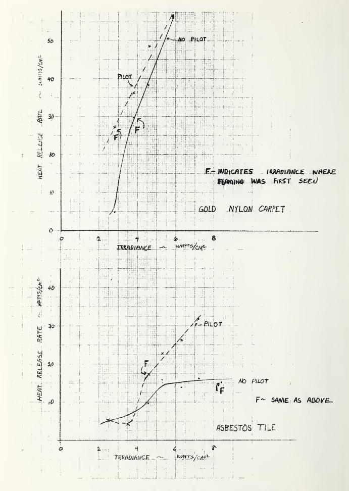
FIGURE 4 - HEAT RELEASE RATES FOR NYLON CARPET AND ASBESTOS TILE
