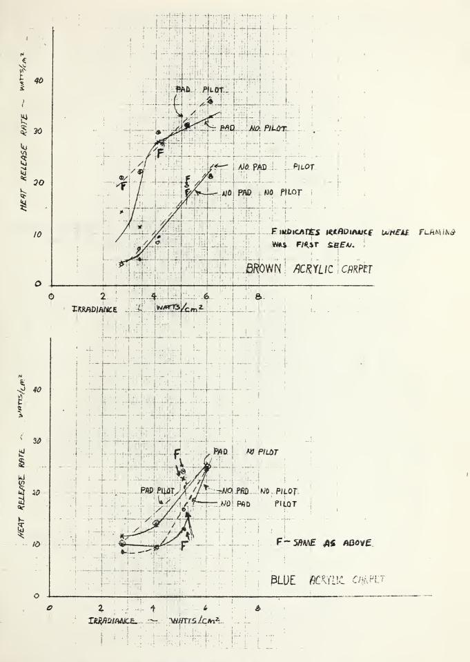
FIGURE 3 - HEAT RELEASE RATES FOR ACRYLIC CARPETS
