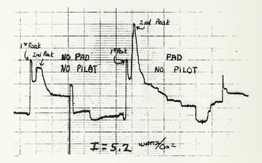
FIGURE 2 - HEAT RELEASE RATE CURVES FOR BROWN ACRYLIC CARPET
