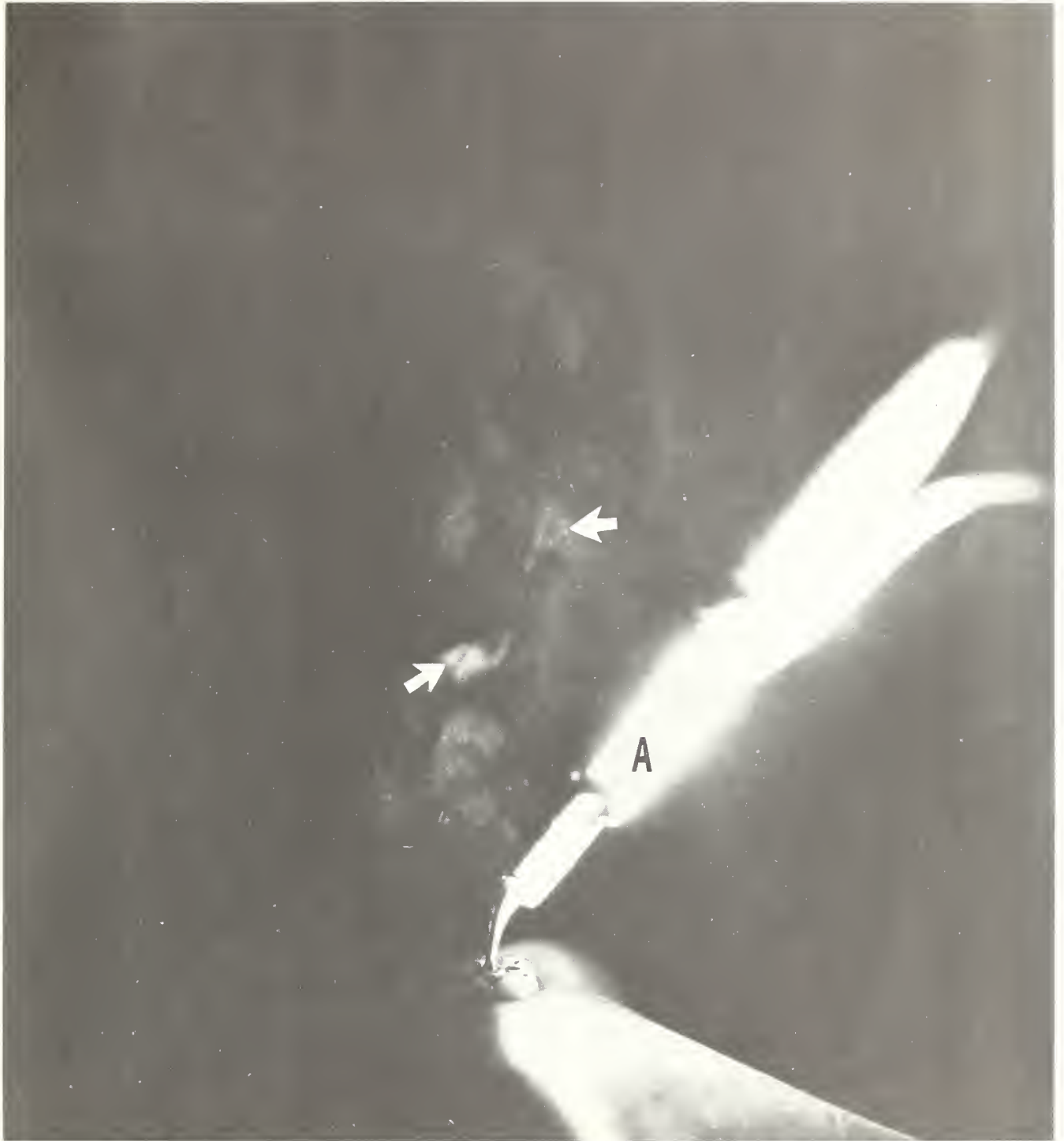
Fig. 1. A cloud of material, arrows, is being emitted from the amalgam at the tip of an ultrasonic amalgam condensing instrument. The particles, also shown in Fig. 3, settle on the instrument handle, A, and may be responsible for some of the haze surrounding the handle.
