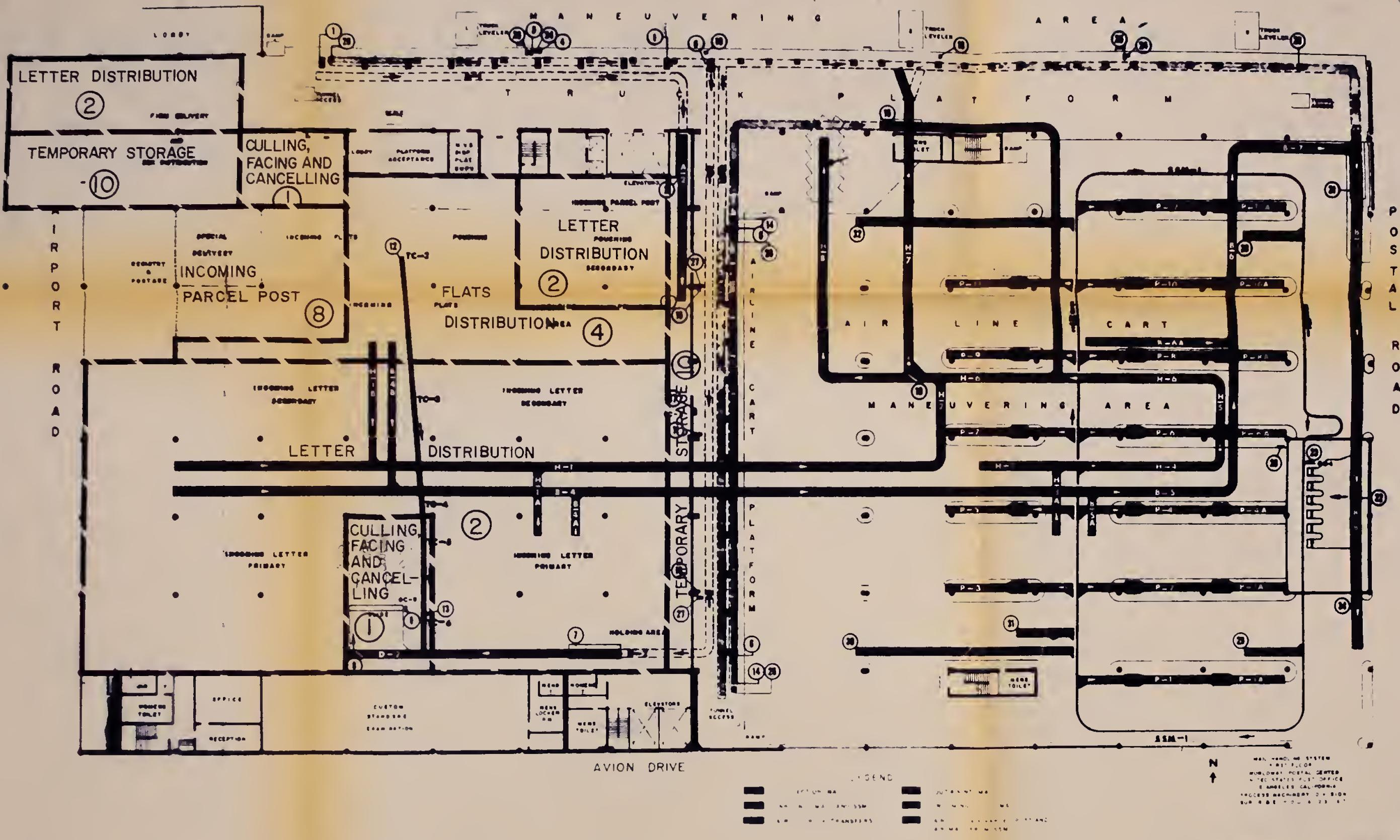
FIG. 5 - LOS ANGELES POST OFFICE FIRST-FLOOR PLAN SHOWING DESIGNATED WORK AREAS
