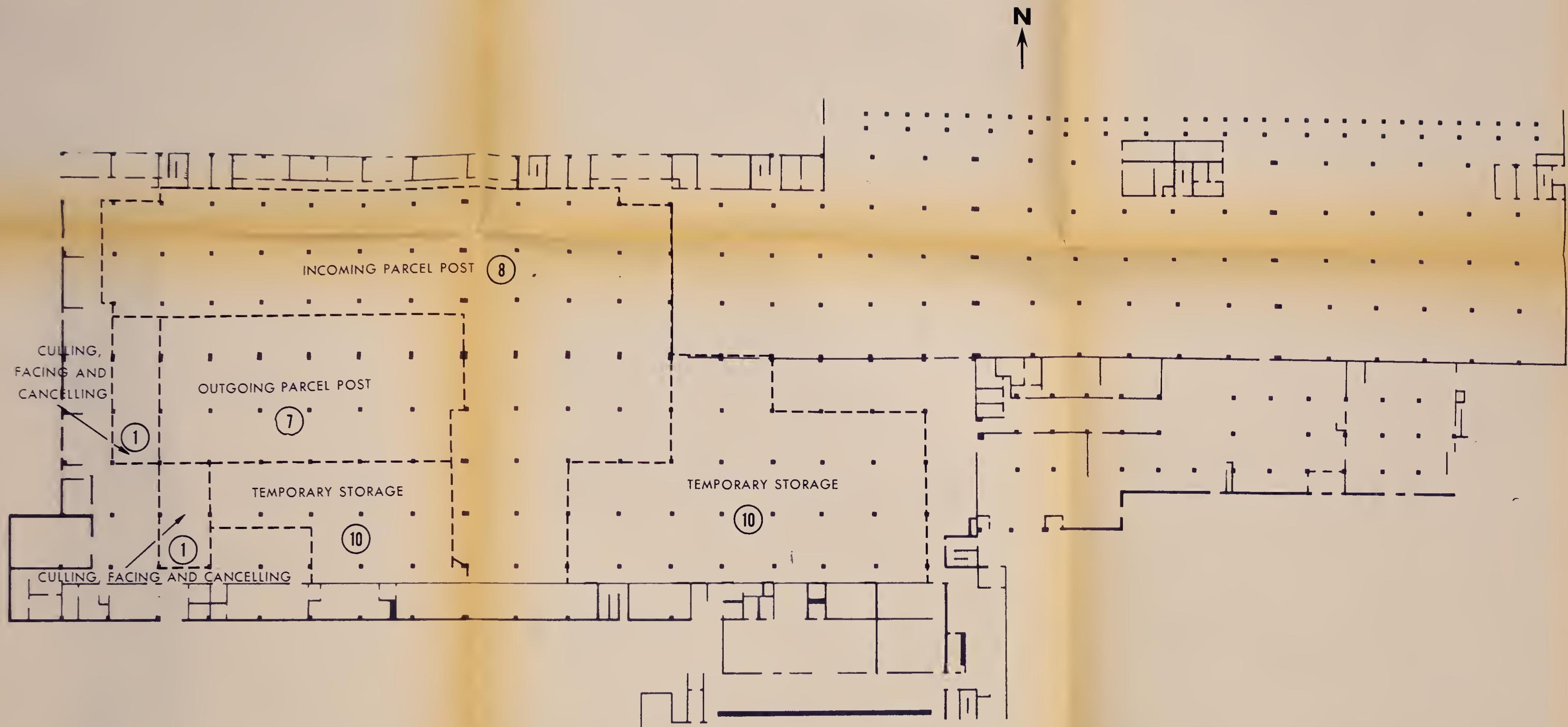
FIG. 1 - HOUSTON POST OFFICE FIRST-FLOOR PLAN SHOWING DESIGNATED WORK AREAS
