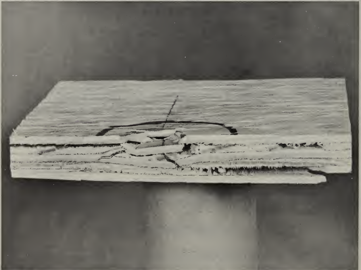
FIGURE 6.9 TYPICAL FAILURE MODE OF FLOOR SYSTEM B LOADED OVER A 5/8 in DIAMETER AREA
