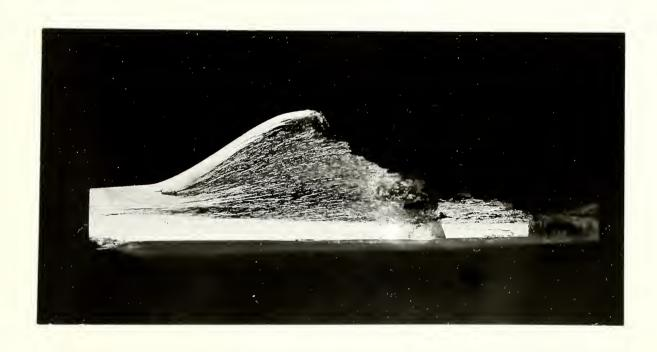
Figure 1. Cross-section of exfoliated 2024-T4
