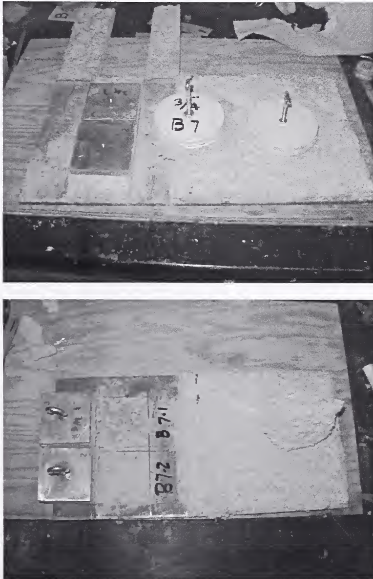
Figure 7-25. Comparative testing: current method versus ASTM E 736 method: (top) locations of two screw cap tests; (bottom) after completion of tests.
