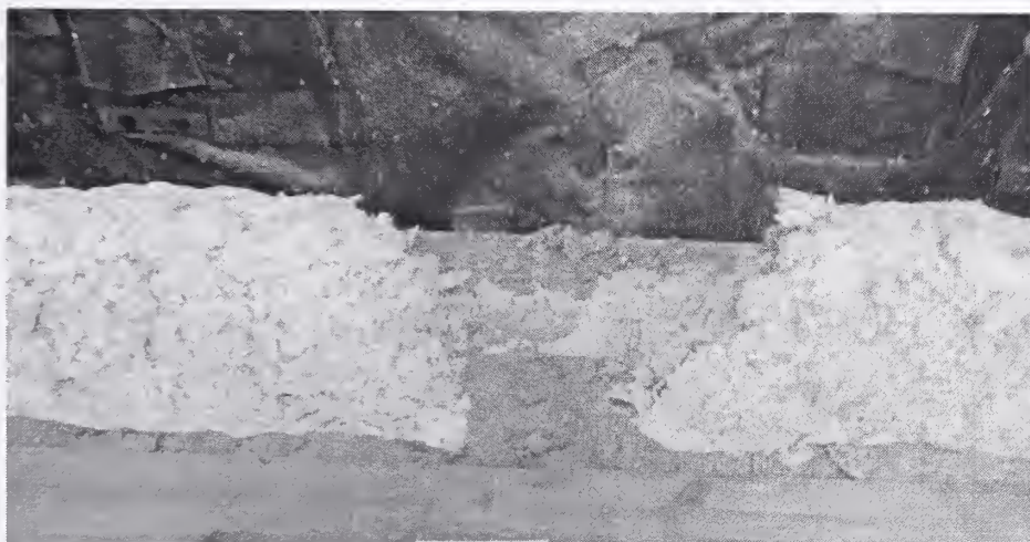
Figure C-11. Photograph showing damage to the SFRM on unprimed steel bar (BAR04) after a debris impact at 0 degree using the large universal receiver.
