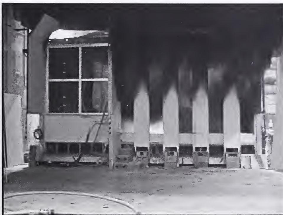
Figure 3-10. View external to the compartment 30 s after ignition of the spray burner in Test 6.
