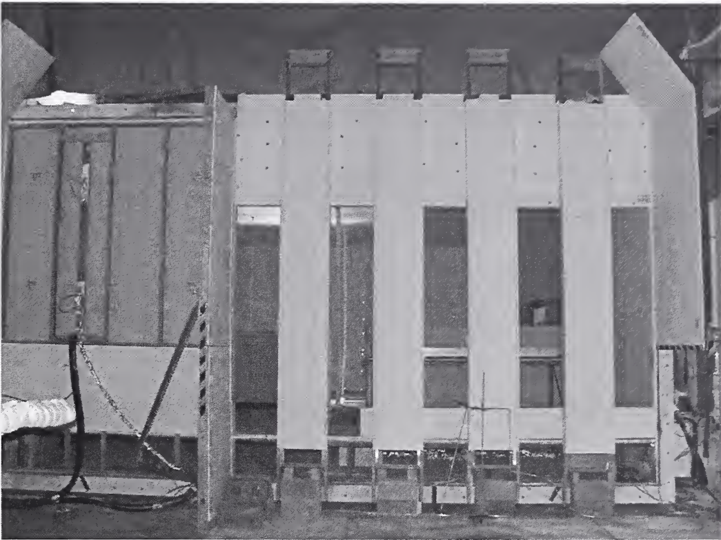
Figure 2–3. West side of experimental enclosure. Five ventilation openings are present. The knee wall was removed for access to instrumentation.
