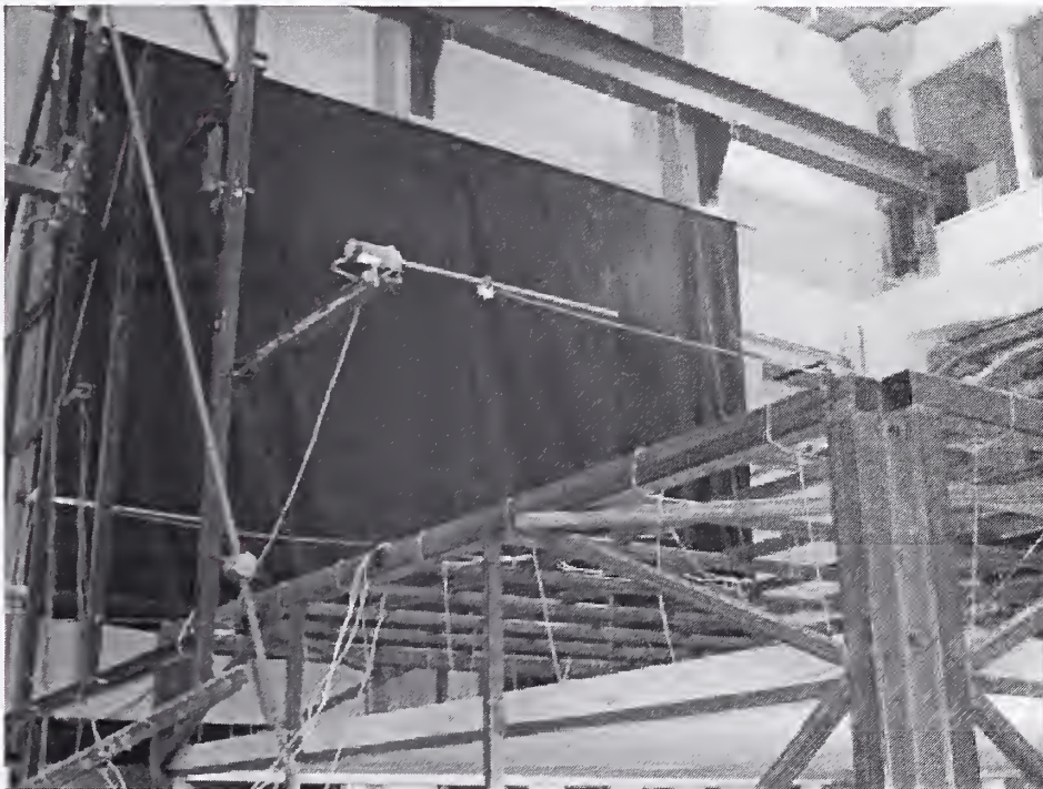
Figure 2-14b. Displacement transducers mounted on the top of the testing frame.
