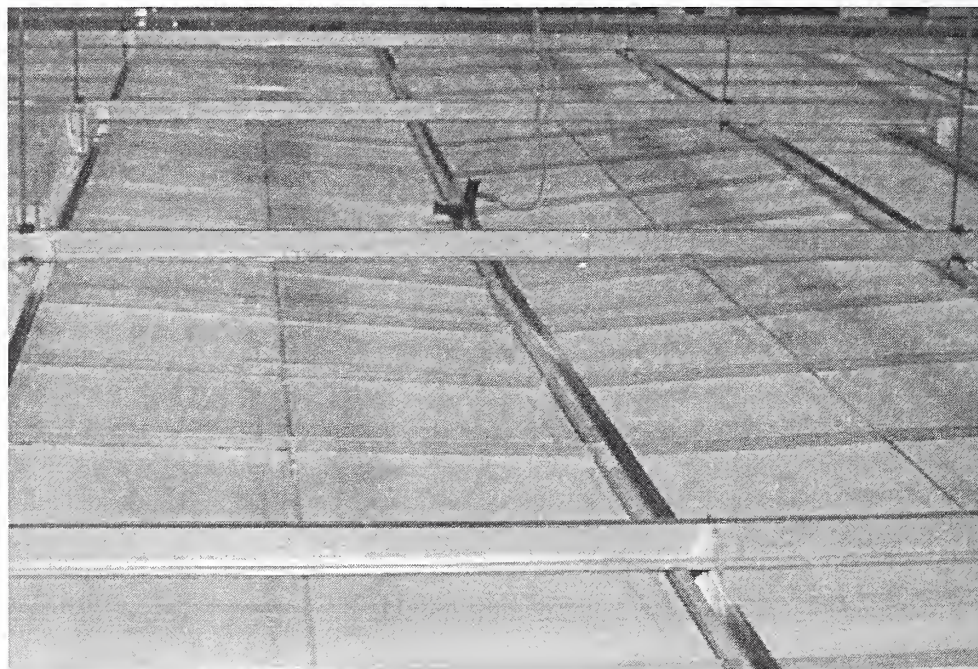
Figure 3–9. Damage to the center of ceiling system CS3 following Test 20.
