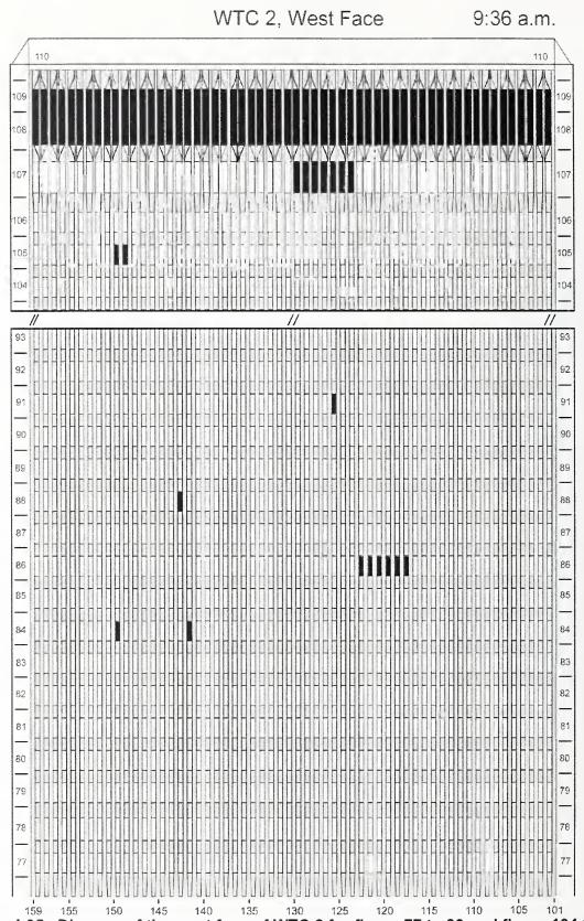
Figure J-35. Diagram of the west face of WTC 2 for floors 77 to 93 and floors 104 to 110 at 9:36 a.m. showing the condition of windows and locations of fires.
