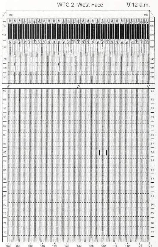
Figure J-11. Diagram of the west face of WTC 2 for floors 77 to 93 and floors 104 to 110 at 9:12 a.m. showing the condition of windows and locations of fires.
