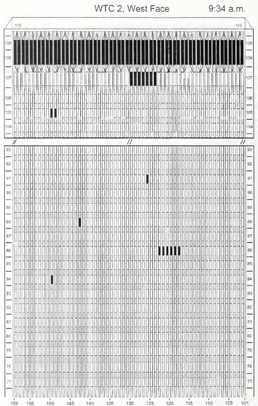
Figure J-33. Diagram of the west face of WTC 2 for floors 77 to 93 and floors 104 to 110 at 9:34 a.m. showing the condition of windows and locations of fires.
