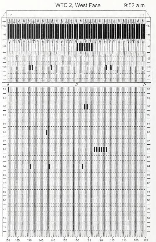
Figure J-51. Diagram of the west face of WTC 2 for floors 77 to 93 and floors 104 to 110 at 9:52 a.m. showing the condition of windows and locations of fires.
