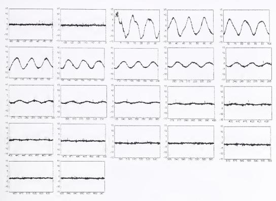
Figure K-16. Division of displacement data into subsets of 1000 points (33.37 s). Data displayed using a common displacement scale.
