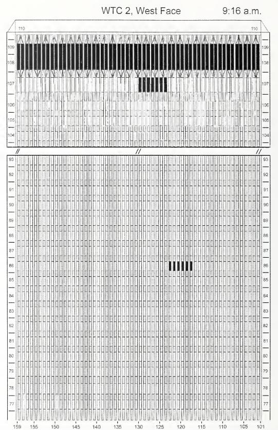
Figure J-15. Diagram of the west face of WTC 2 for floors 77 to 93 and floors 104 to 110 at 9:16 a.m. showing the condition of windows and locations of fires.
