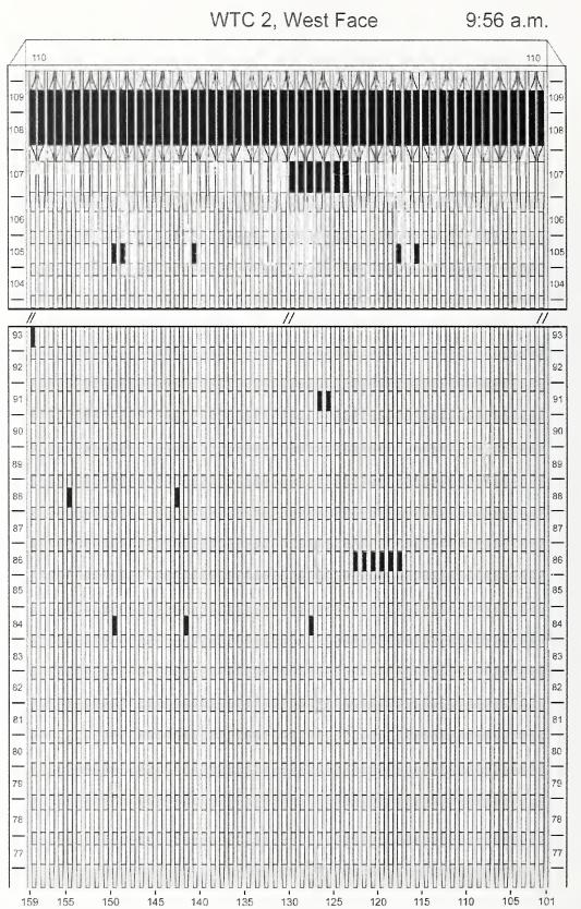
Figure J-55. Diagram of the west face of WTC 2 for floors 77 to 93 and floors 104 to 110 at 9:56 a.m. showing the condition of windows and locations of fires.
