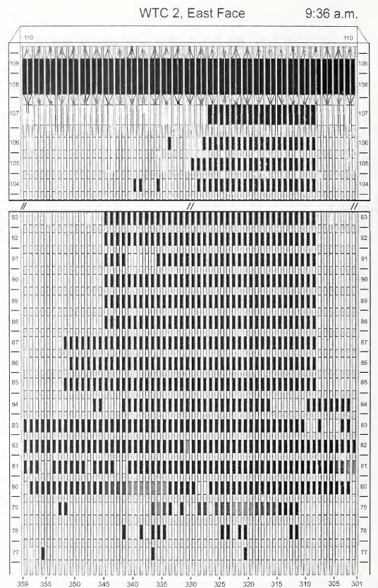
Figure H-35. Diagram of the east face of WTC 2 for floors 77 to 93 and floors 104 to 110 at 9:36 a.m. showing the condition of windows and locations of fires.
