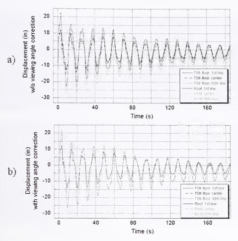
Figure K-25. WTC 2 displacement at 70th floor and extrapolation to displacement at roof (a) before and (b) after correction for camera viewing angle. Oscillations in the angle increment variable  $\Delta\theta$  have been removed.
