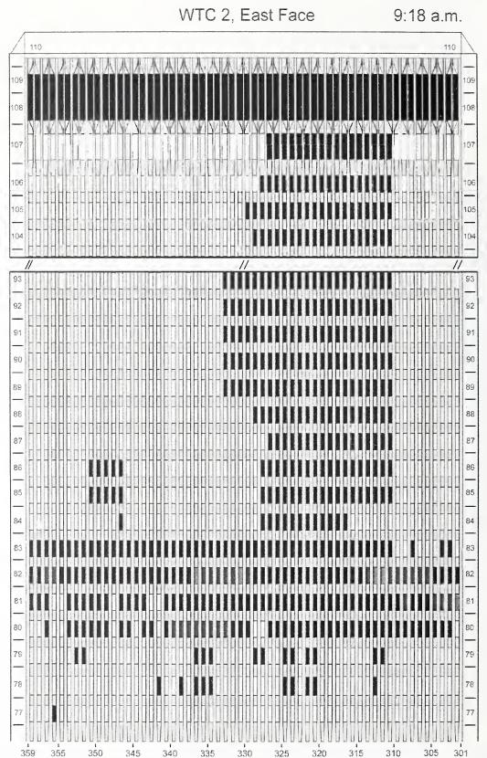
Figure H-17. Diagram of the east face of WTC 2 for floors 77 to 93 and floors 104 to 110 at 9:18 a.m. showing the condition of windows and locations of fires.
