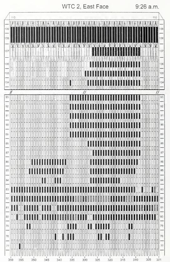
Figure H-25. Diagram of the east face of WTC 2 for floors 77 to 93 and floors 104 to 110 at 9:26 a.m. showing the condition of windows and locations of fires.
