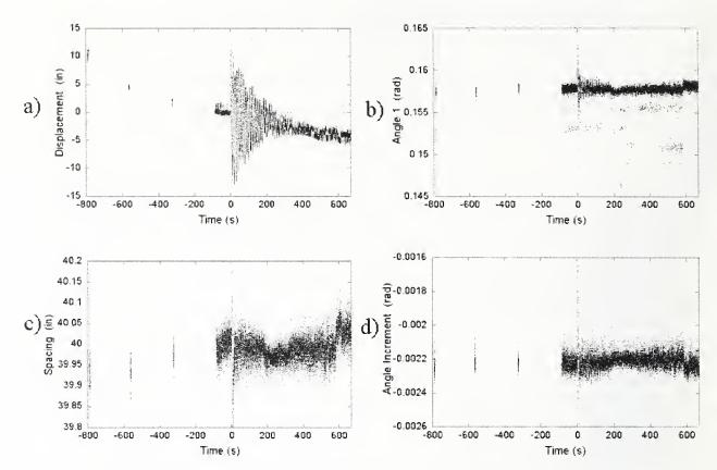
Figure K-7. Plots of WTC 2 analysis results over the entire duration of the uninterrupted video for a) displacement of the first window line  $d_1$ , b) angle of the first line  $\theta_1$ , c) window spacing p, and d) angle increment  $\Delta\theta$ .
