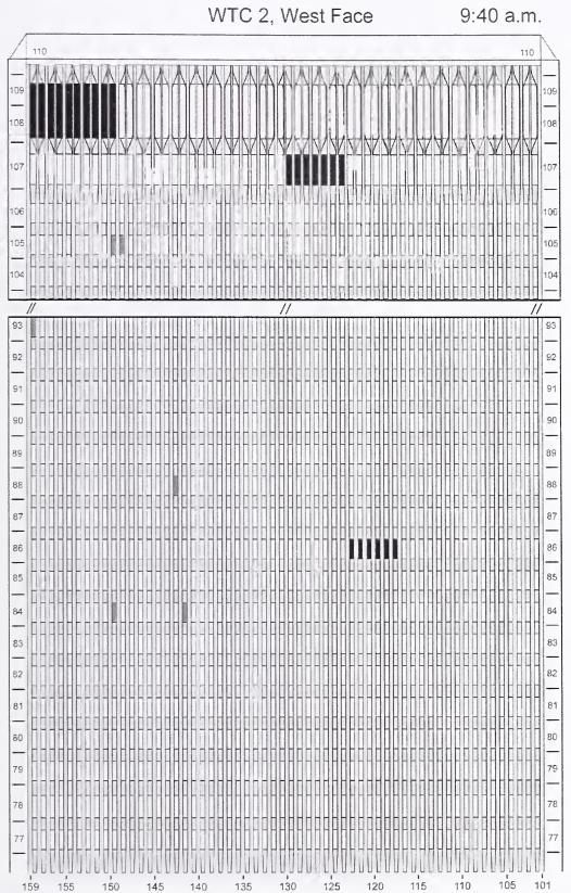
Figure J-40. Diagram of the west face of WTC 2 for floors 77 to 93 and floors 104 to 110 at 9:40 a.m. showing windows where smoke was observed and those hidden from view.
