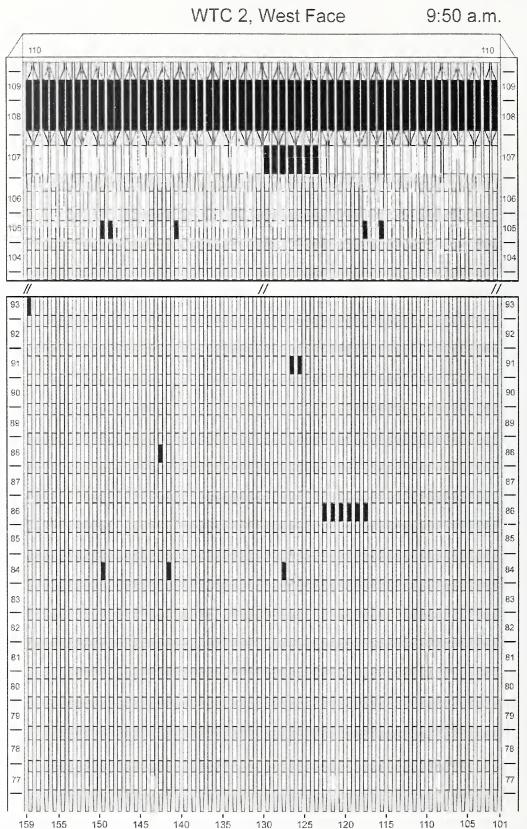
Figure J-49. Diagram of the west face of WTC 2 for floors 77 to 93 and floors 104 to 110 at 9:50 a.m. showing the condition of windows and locations of fires.
