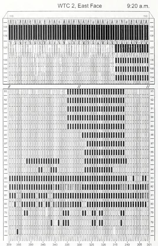
Figure H-19. Diagram of the east face of WTC 2 for floors 77 to 93 and floors 104 to 110 at 9:20 a.m. showing the condition of windows and locations of fires.
