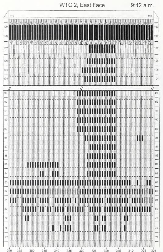
Figure H-11. Diagram of the east face of WTC 2 for floors 77 to 93 and floors 104 to 110 at 9:12 a.m. showing the condition of windows and locations of fires.
