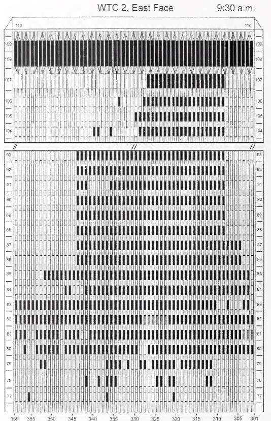
Figure H-29. Diagram of the east face of WTC 2 for floors 77 to 93 and floors 104 to 110 at 9:30 a.m. showing the condition of windows and locations of fires.
