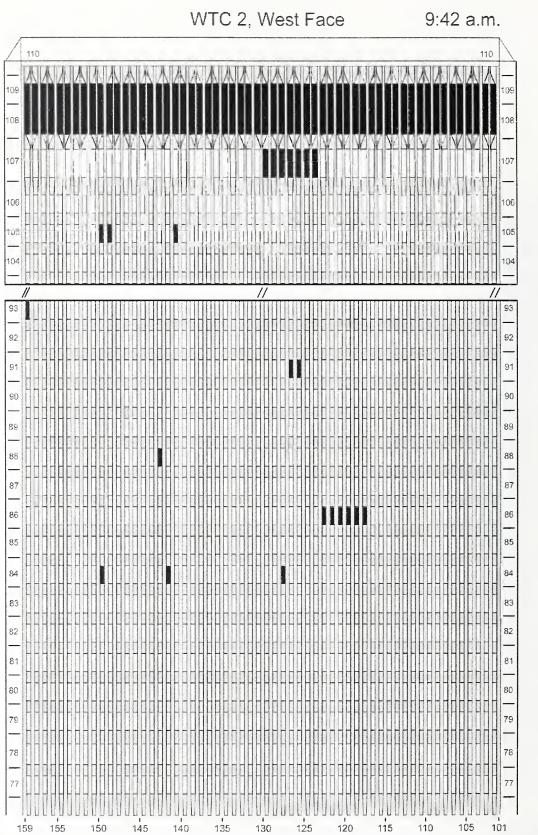
Figure J-41. Diagram of the west face of WTC 2 for floors 77 to 93 and floors 104 to 110 at 9:42 a.m. showing the condition of windows and locations of fires.
