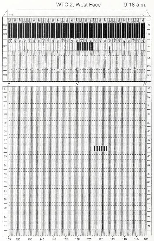
Figure J-17. Diagram of the west face of WTC 2 for floors 77 to 93 and floors 104 to 110 at 9:18 a.m. showing the condition of windows and locations of fires.
