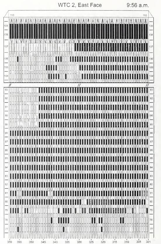
Figure H-55. Diagram of the east face of WTC 2 for floors 77 to 93 and floors 104 to 110 at 9:56 a.m. showing the condition of windows and locations of fires.
