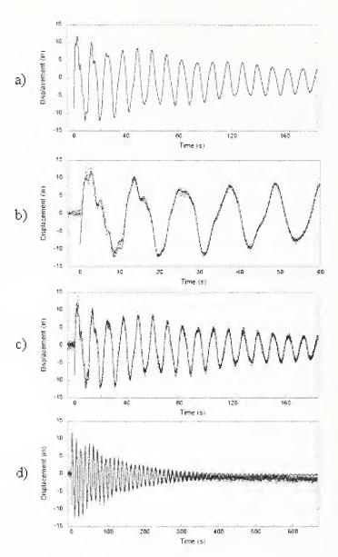
Figure K-15. Sum of four modes and a comparison with displacement data.
