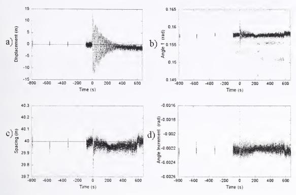
Figure K-11. Plots of corrected WTC 2 analysis results over the entire duration of the uninterrupted video for a) building displacement of the first window line at the 70th floor  $d_1$ , b) angle of the first line  $\theta_1$ , c) window spacing p, and d) angle increment  $\Delta\theta$ .
