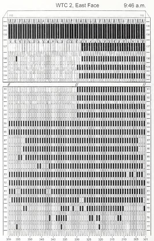
Figure H-45. Diagram of the east face of WTC 2 for floors 77 to 93 and floors 104 to 110 at 9:46 a.m. showing the condition of windows and locations of fires.
