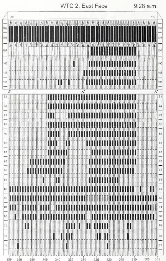
Figure H-27. Diagram of the east face of WTC 2 for floors 77 to 93 and floors 104 to 110 at 9:28 a.m. showing the condition of windows and locations of fires.
