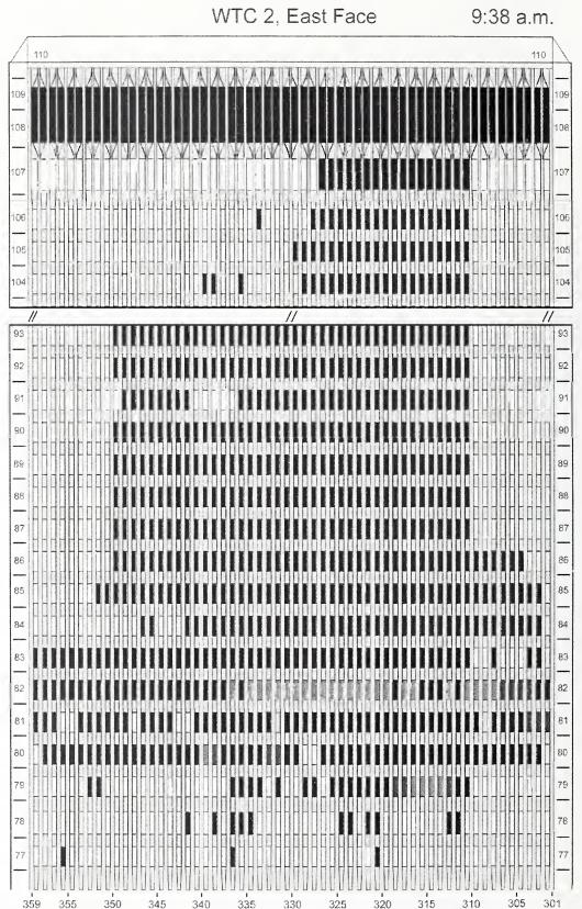
Figure H-37. Diagram of the east face of WTC 2 for floors 77 to 93 and floors 104 to 110 at 9:38 a.m. showing the condition of windows and locations of fires.
