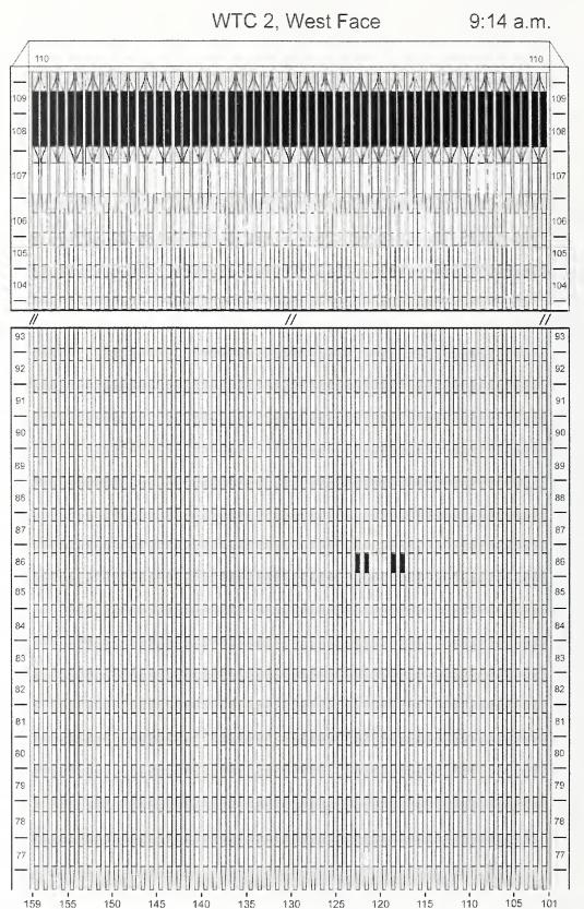
Figure J-13. Diagram of the west face of WTC 2 for floors 77 to 93 and floors 104 to 110 at 9:14 a.m. showing the condition of windows and locations of fires.
