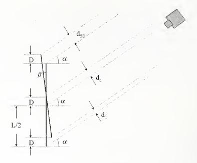
Figure K-23. Viewing angle geometry at first extremum of sway, with building displacement to north and counter-clockwise rotation.
