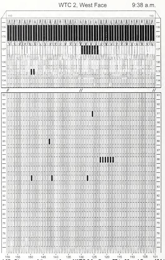
Figure J-37. Diagram of the west face of WTC 2 for floors 77 to 93 and floors 104 to 110 at 9:38 a.m. showing the condition of windows and locations of fires.
