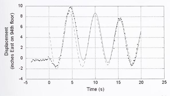
Figure K-29. Comparison of data (blue dots) to modes from nonlinear analyses of data starting at 0 s (dashed red line) and 2 s (solid red line).
