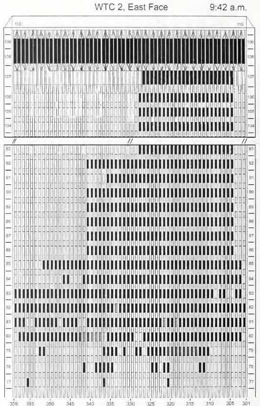
Figure H-41. Diagram of the east face of WTC 2 for floors 77 to 93 and floors 104 to 110 at 9:42 a.m. showing the condition of windows and locations of fires.
