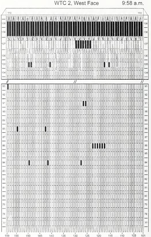
Figure J-57. Diagram of the west face of WTC 2 for floors 77 to 93 and floors 104 to 110 at 9:58 a.m. showing the condition of windows and locations of fires.
