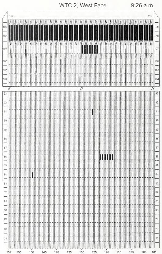
Figure J-25. Diagram of the west face of WTC 2 for floors 77 to 93 and floors 104 to 110 at 9:26 a.m. showing the condition of windows and locations of fires.
