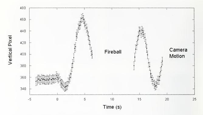
Figure K–28. Vertical displacement of index point measuring east-west motion of WTC 2 just before and after aircraft impact. Higher values indicate motion to the east. Red error bars indicate uncertainty.
