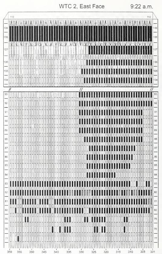
Figure H-21. Diagram of the east face of WTC 2 for floors 77 to 93 and floors 104 to 110 at 9:22 a.m. showing the condition of windows and locations of fires.
