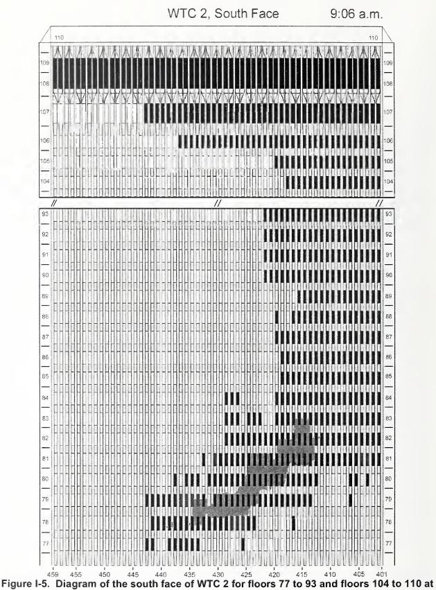
Figure I-5. Diagram of the south face of WTC 2 for floors 77 to 93 and floors 104 to 110 at 9:06 a.m. showing the condition of windows and locations of fires.
