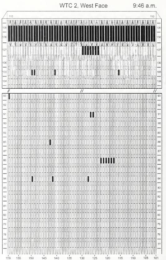
Figure J-45. Diagram of the west face of WTC 2 for floors 77 to 93 and floors 104 to 110 at 9:46 a.m. showing the condition of windows and locations of fires.
