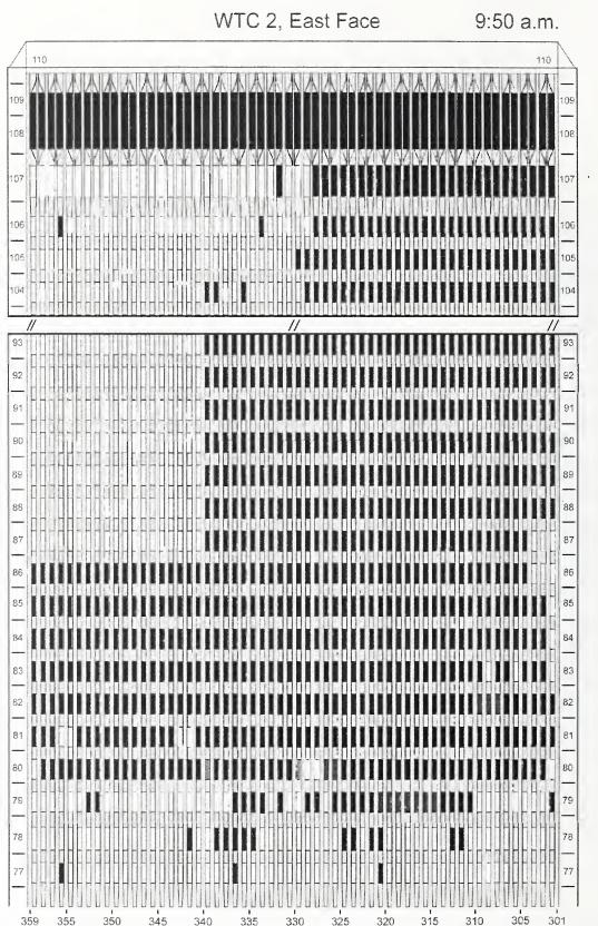
Figure H-49. Diagram of the east face of WTC 2 for floors 77 to 93 and floors 104 to 110 at 9:50 a.m. showing the condition of windows and locations of fires.
