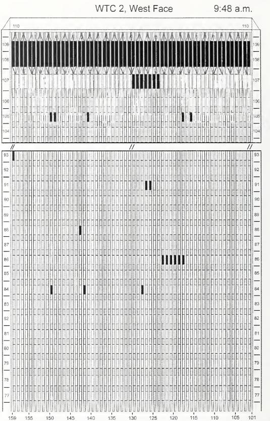
Figure J-47. Diagram of the west face of WTC 2 for floors 77 to 93 and floors 104 to 110 at 9:48 a.m. showing the condition of windows and locations of fires.
