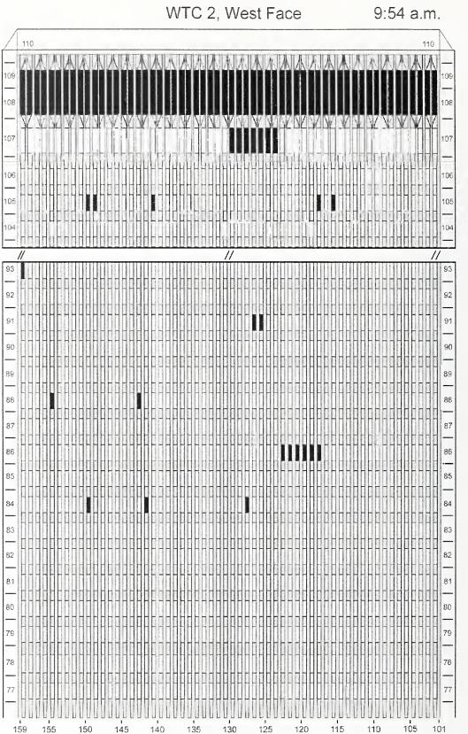
Figure J-53. Diagram of the west face of WTC 2 for floors 77 to 93 and floors 104 to 110 at 9:54 a.m. showing the condition of windows and locations of fires.
