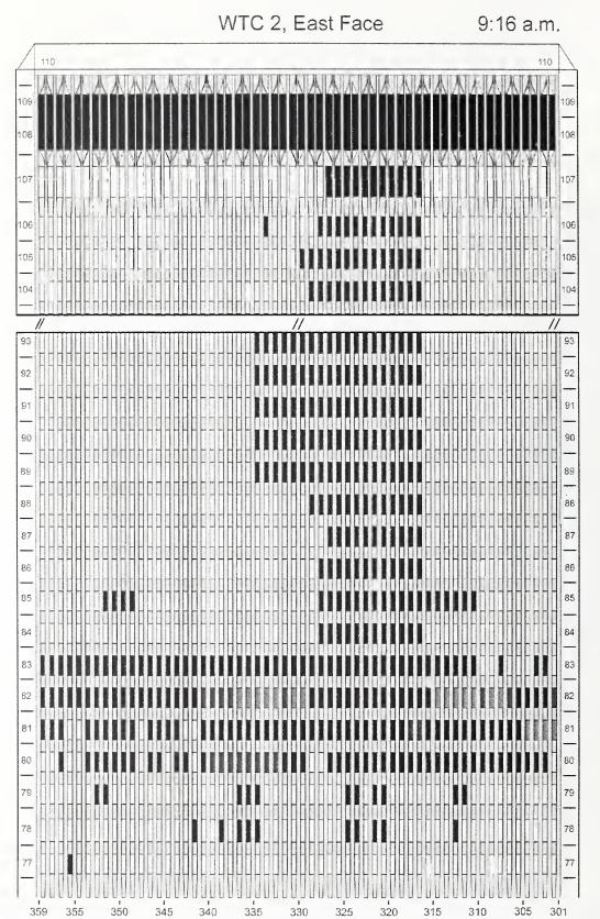
Figure H-15. Diagram of the east face of WTC 2 for floors 77 to 93 and floors 104 to 110 at 9:16 a.m. showing the condition of windows and locations of fires.
