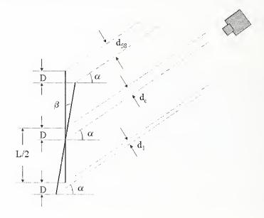
Figure K-24. Viewing angle geometry at second extremum of sway, with building displacement to south and clockwise rotation. Values of D and  $\beta$  are negative in this configuration.
