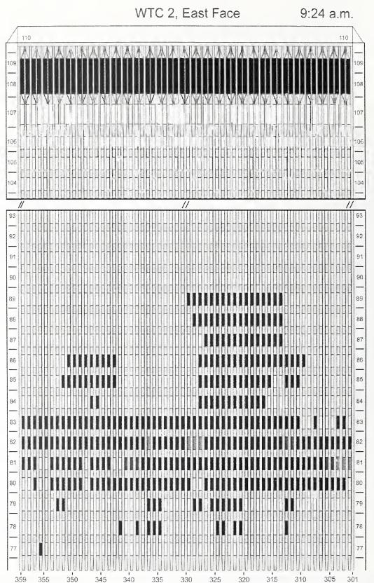
Figure H-23. Diagram of the east face of WTC 2 for floors 77 to 93 and floors 104 to 110 at 9:24 a.m. showing the condition of windows and locations of fires.
