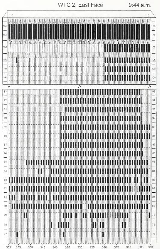
Figure H-43. Diagram of the east face of WTC 2 for floors 77 to 93 and floors 104 to 110 at 9:44 a.m. showing the condition of windows and locations of fires.
