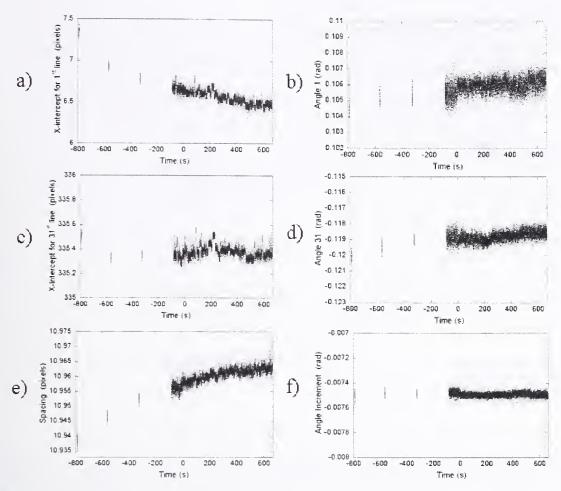
Figure K–9. Plots of fixed building analysis results over the entire duration of the unadjusted video for a) x-intercept of the first line  $s_1$  in horizontal pixels, b) angle of the first line  $\phi_1$ , c) x-intercept of the 31st line  $s_3$ , d) angle of the 31st line  $\phi_3$ , e) line spacing  $\Delta s = (s_1 - s_3) / 30$ , and f) angle increment  $\Delta \phi = (\phi_1 - \phi_3) / 30$ .
