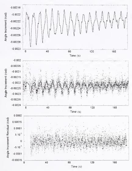
Figure K-22. Angle increment modes: a) sum of four modes, b) comparison to data, c) residual after subtraction of sum of modes from data.
