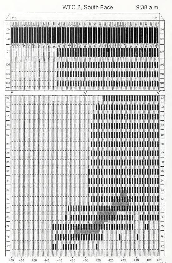
Figure I-37. Diagram of the south face of WTC 2 for floors 77 to 93 and floors 104 to 110 at 9:38 a.m. showing the condition of windows and locations of fires.
