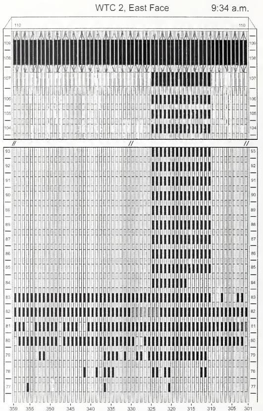
Figure H-33. Diagram of the east face of WTC 2 for floors 77 to 93 and floors 104 to 110 at 9:34 a.m. showing the condition of windows and locations of fires.
