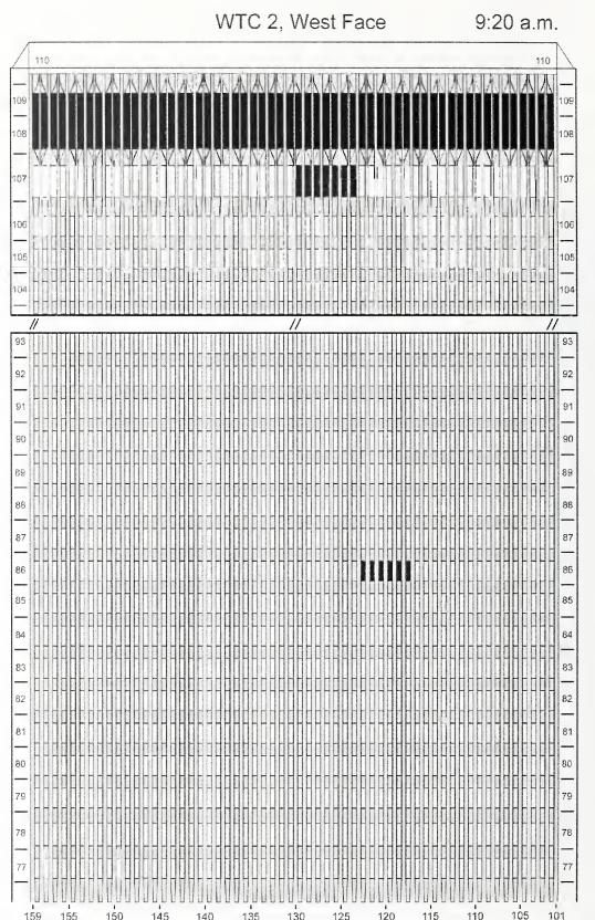
Figure J-19. Diagram of the west face of WTC 2 for floors 77 to 93 and floors 104 to 110 at 9:20 a.m. showing the condition of windows and locations of fires.
