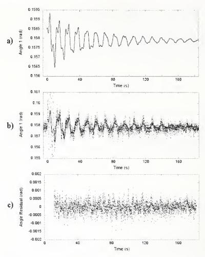
Figure K-21. Angle modes: a) sum of four modes, b) comparison to data, c) residual after subtraction of sum of modes from data.
