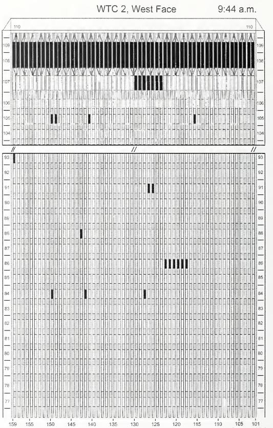
Figure J-43. Diagram of the west face of WTC 2 for floors 77 to 93 and floors 104 to 110 at 9:44 a.m. showing the condition of windows and locations of fires.
