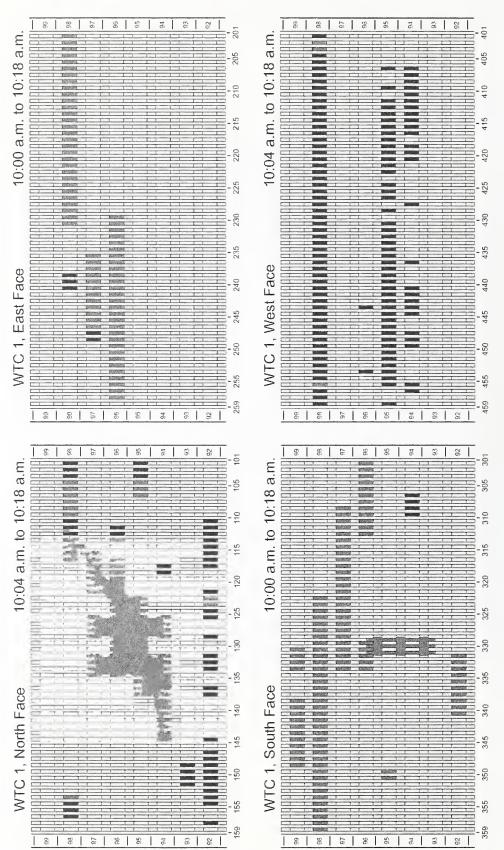
Figure 8-93. Maps of integrated fire observations between 10:00 a.m. and 10:18 a.m. are shown for the four faces of WTC 1. Colors represent the highest intensity fire observed in a window using the color scale defined in Figure 5-1.
