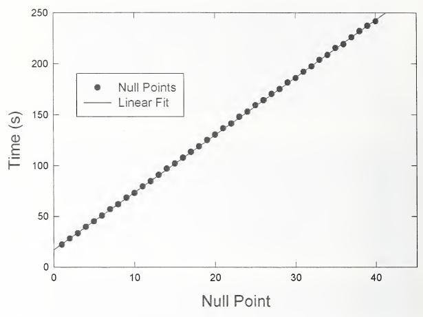
Figure 7-15. The time when null points are observed in the difference video of WTC 2 are plotted versus the null point number. The points fall on a straight line having a slope of  $5.647 \text{ s} \pm 0.008 \text{ s}$ .
