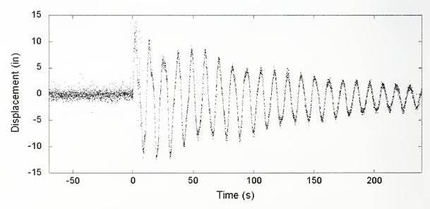
Figure 7-18. The displacement of the first (left-most) window line on the 70th floor of WTC 2 determined using moiré analysis is shown as a function of time.
