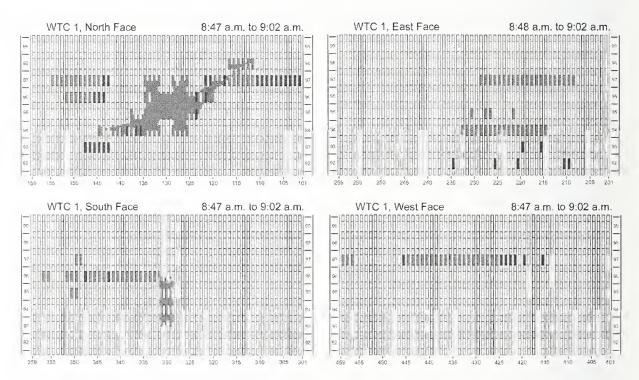
Figure E-4. Maps of integrated fire observations between 8:47 a.m. and 9:03 a.m. are shown for the four faces of WTC 1.
