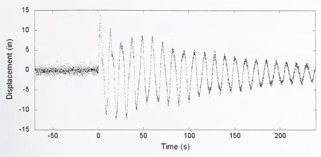
Figure E-2. The displacement of the first (left-most) window line on the 70th floor of WTC 2 determined using moiré analysis is shown as a function of time.
