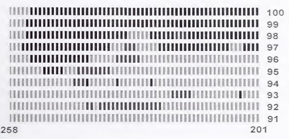
Figure 5-3. A representation of fires for floors 91 to 100 on the east face of WTC 1 around 9:42 a.m. is shown. Results are taken from the Excel spreadsheet shown in Figure 5-2.
