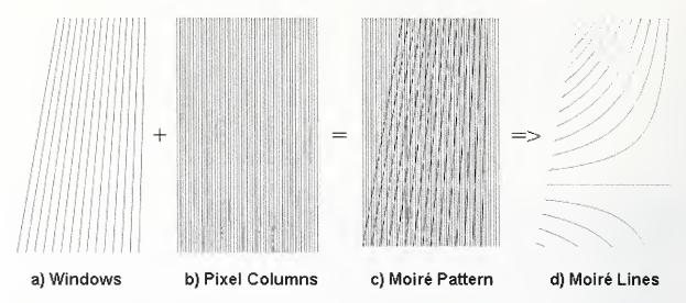
Figure 7-17. Drawings demonstrate the formation of a moiré fringe pattern (c and d) by the superposition of the lines on a tower façade (a) with the vertical columns of picture elements (pixels) of a digital camera.
