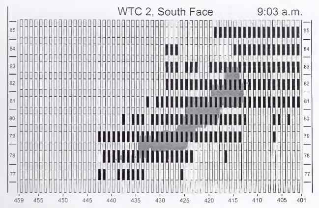
Figure 7-27. A schematic of observed window conditions on the south face of WTC 2 immediately following the aircraft impact is shown. Window and floor numbers are indicated. The colors represent • window broken open, • glass in place, and • not visible.
