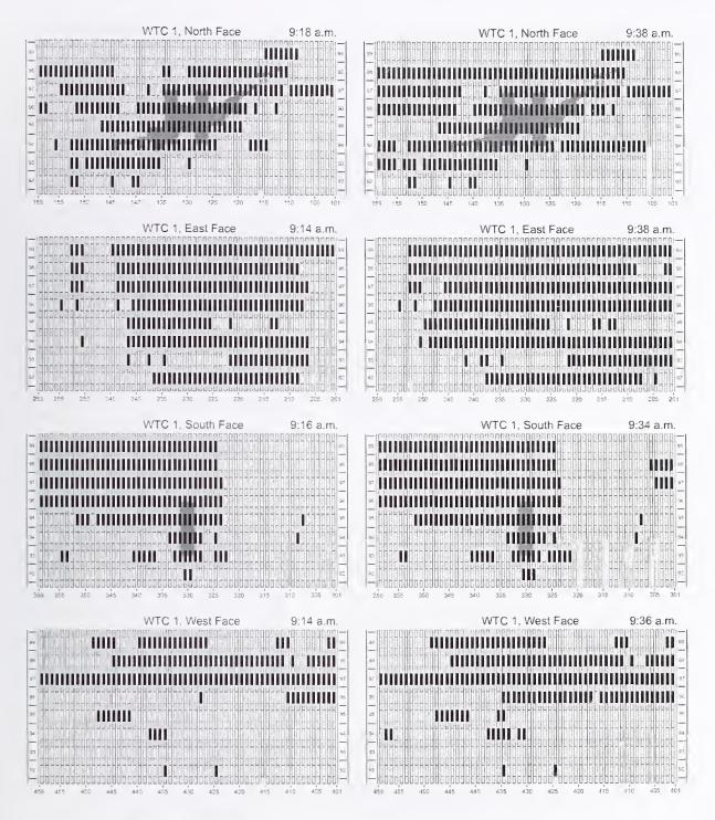
Figure 8-50. Maps for the 92nd through the 99th floors compare missing window glass for the four faces of WTC 1 at two times, around 9:18 a.m. and roughly 17 minutes later.
