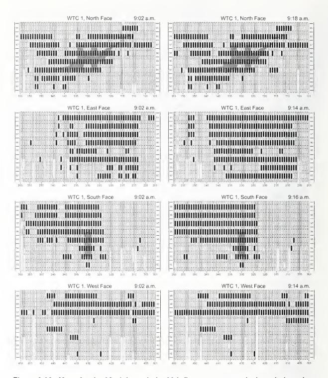
Figure 8-32. Maps for the 92nd through the 99th floors compare missing window glass for the four faces of WTC 1 at two times, around 9:02 a.m. and roughly 15 minutes later.
