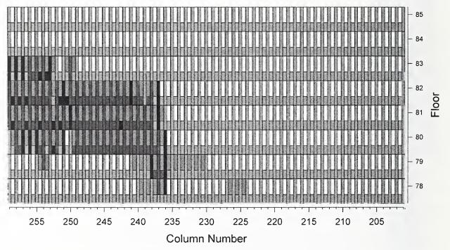
Figure 7-33. A color-coded visualization of initial damage to the north face of WTC 2 is shown. Information concerning damage to the aluminum on the curtain wall ( - undisturbed, - disturbed but still in place, and - aluminum facing missing) and windows ( - glass missing and - glass in place) are combined.
