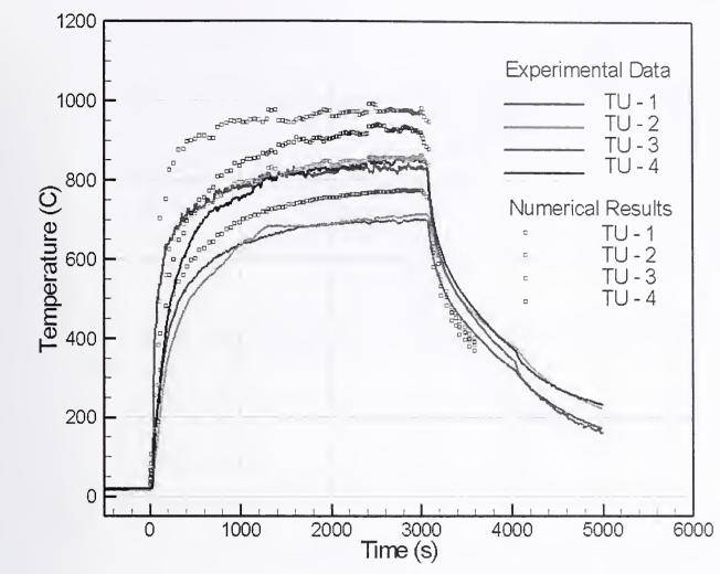
Figure 5–18. Comparison of numerical simulations with measurements for the temperature of the SFRM surface at four locations 3.70 m above the floor on the north truss in Test 5.
