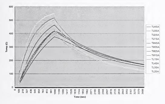
Figure 3–12. Temperature-time history for truss A in Test 3.
