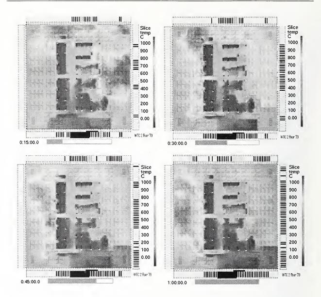
Figure 6–19. Simulated upper layer temperatures on floor 79 of WTC 2, Case C.
