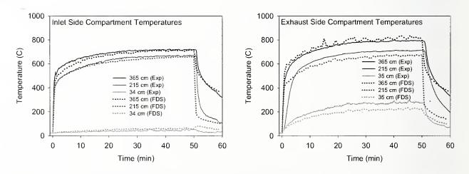
Figure 4–2. Comparison of predicted and measured gas temperatures at various heights above the floor, Test 5.
