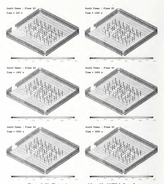
Figure 6-58. Thermal response of floor 83 of WTC 2, Case C.
