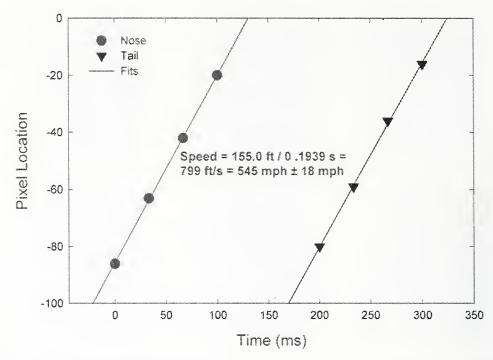
Figure 2–8. Plots of pixel locations for the nose and tail of the aircraft that struck WTC 2 as a function of time taken from the images shown in Figure 2–7.
