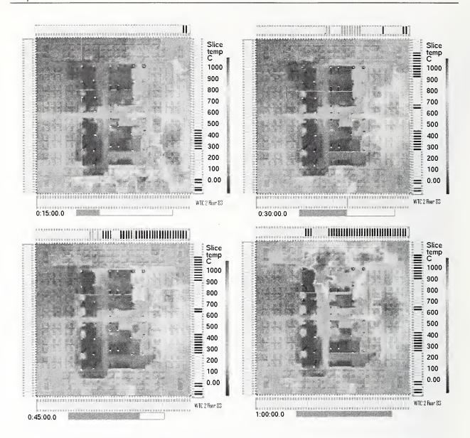
Figure 6-27. Simulated upper layer temperatures on floor 83 of WTC 2, Case C.
