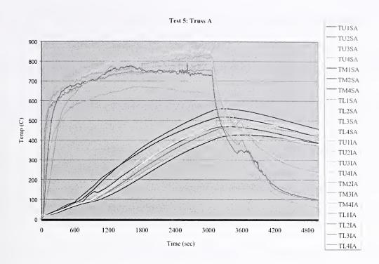
Figure 3-11. Temperature-time history for truss A in Test 5.
