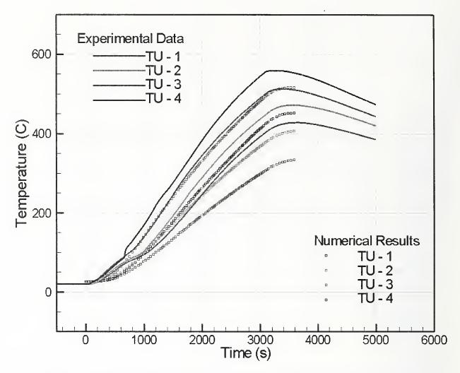
Figure 5–19. Comparison of numerical simulations with measurements for the temperature of the steel surface at four locations 3.70 m above the floor on the north truss in Test 5.
