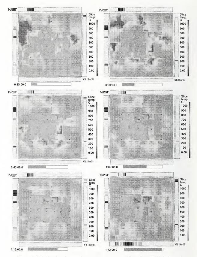
Figure 6–15. Simulated upper layer temperatures on floor 99 of WTC 1, Case A.
