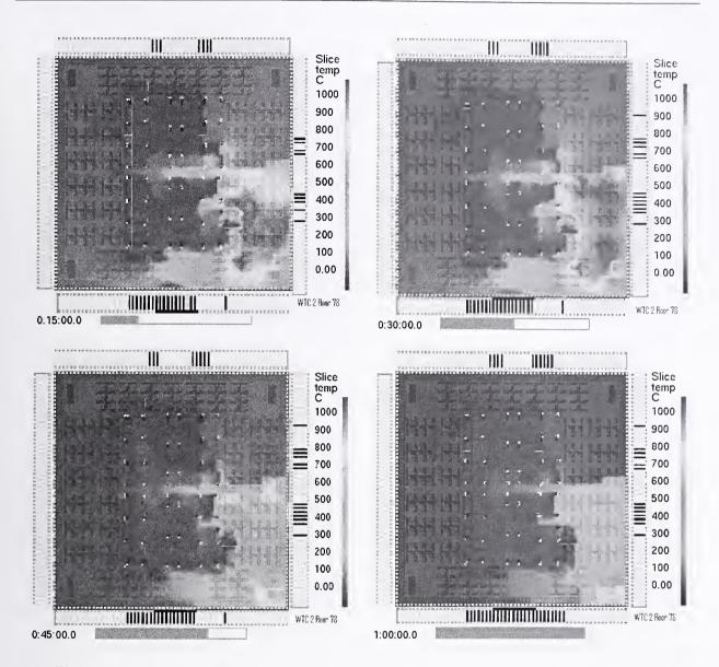
Figure 6-18. Simulated upper layer temperatures on floor 78 of WTC 2, Case D.
