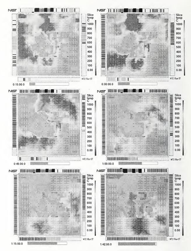
Figure 6–11. Simulated upper layer temperatures on floor 97 of WTC 1, Case A.
