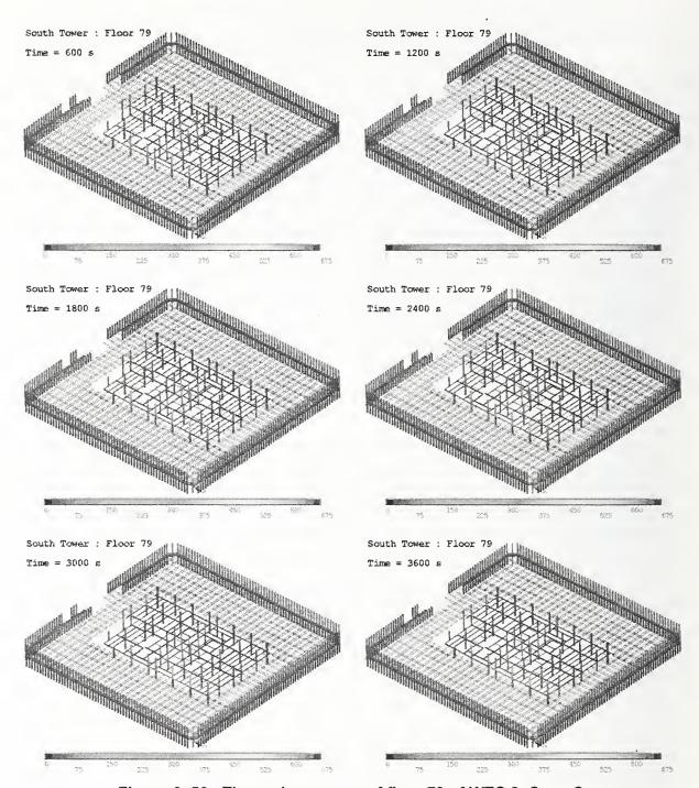
Figure 6-50. Thermal response of floor 79 of WTC 2, Case C.
