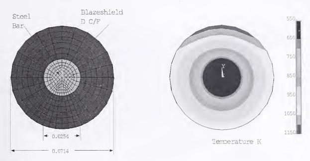
Figure 5–4. FSI grid structure of insulated steel rod (with dimensions in meters) showing the elements used to model the steel (in blue) and the SFRM (in violet), and the temperature contours after 2,000 s in Test 5.
