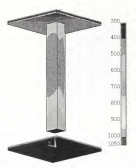
Figure 5–6. Temperature (in K) contours on the outer surface of the SFRM and the ceiling after 2,000 s in Test 5.
