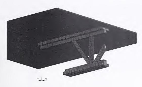
Figure 5–8. Finite element representation of the insulated steel truss (blue), the SFRM (violet), and the ceiling (red) used in the thermal analysis of Test 5.
