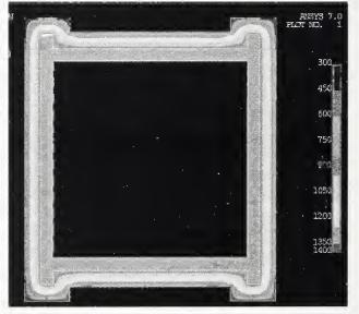
Figure 5–1. Finite element model of light box shape core column and temperature contours (Kelvin) at one instant in time.
