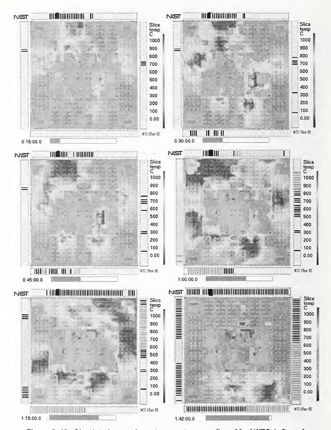
Figure 6-13. Simulated upper layer temperatures on floor 98 of WTC 1, Case A.
