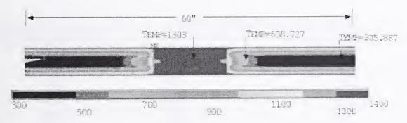
Figure 5–2. Temperature rise (K) in a plate with a 12 in. gap in the thermal insulation.
