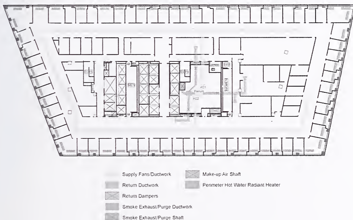
Figure 4-11. Air distribution system, 24th floor, WTC 7.
