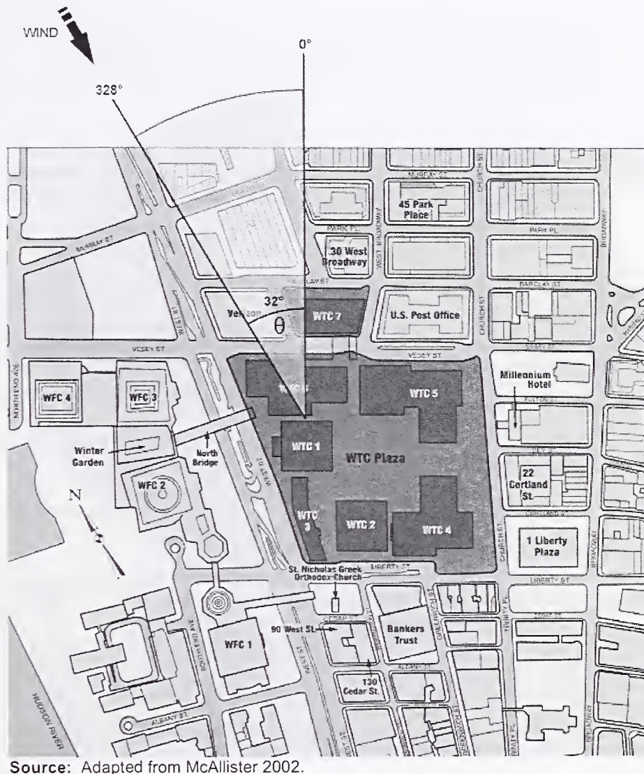
Figure B-2. Illustration of a northerly wind modeled in CONTAM at 328 degrees.
