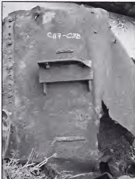
Figure B-16. Floor truss connectors found on recovered panel C-117 (building and column line unknown, floors 101-104). Connectors are shown on the unknown column at different floor levels (cont.).
