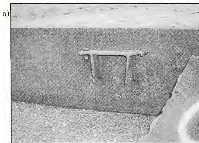
Seat 1: One hole intact with bolt, other ripped out
