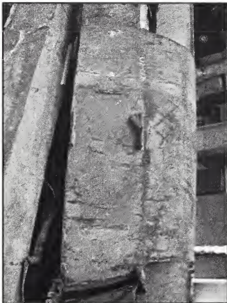
Figure B-6. Floor truss connectors found on recovered panel C-22 (A157: 93-96) from WTC 1. Shown are connectors found on column 157 at different floor levels (cont.).
