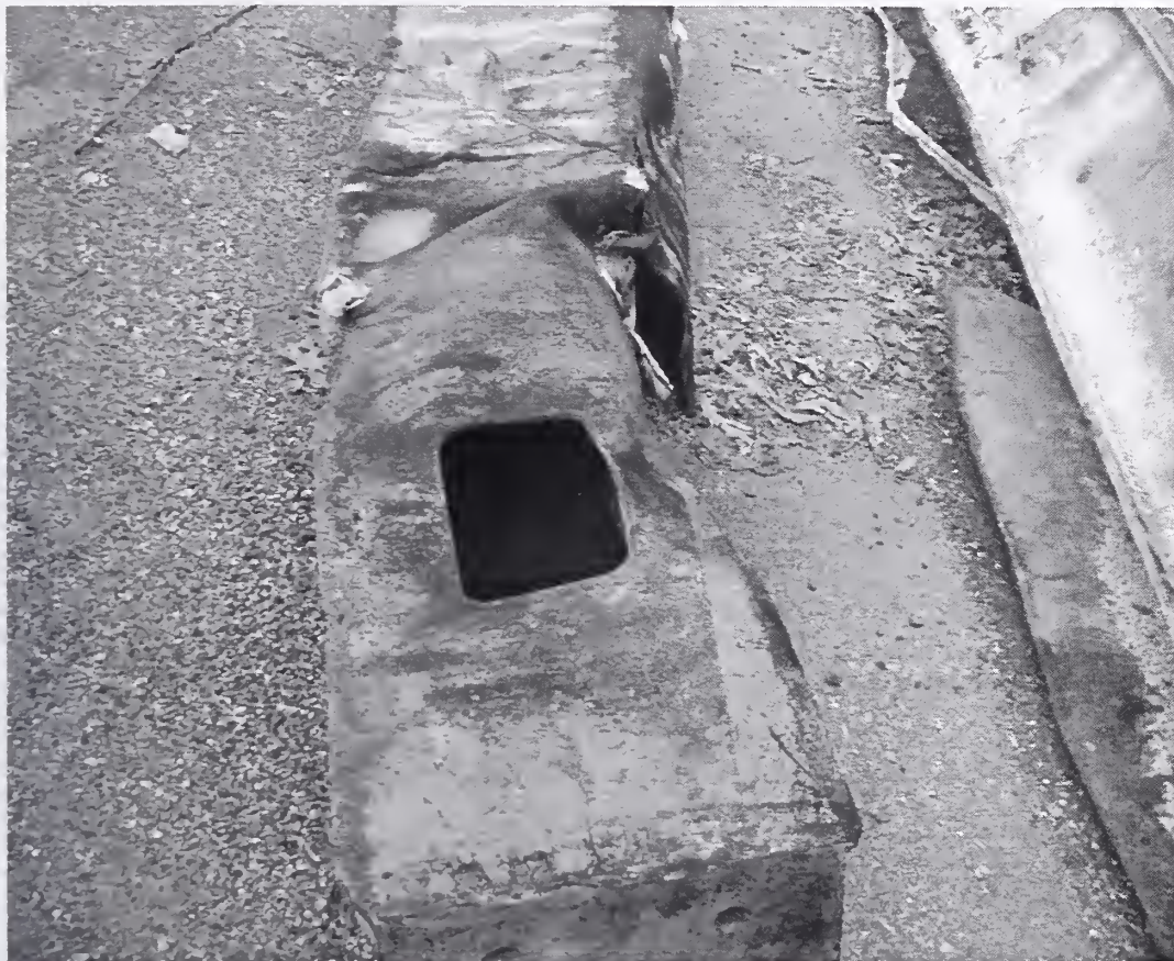
Figure 17. Possible fire effects on lower end of Piece K-2
