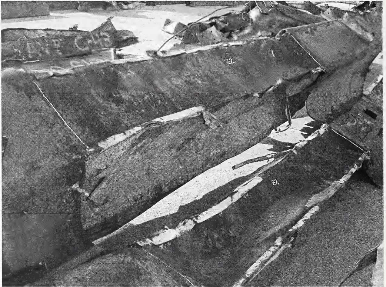
Figure 16. Pattern of presence and absence of possible fire effects on column elements of Piece M-4. Zones marked Z2 at middle are possible fire-affected areas at window openings. Spandrel plates above and below window openings appear unaffected by fire.
