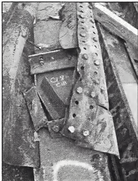
Figure B-5. Floor truss connectors found on recovered panel C-18 (B230: 93-96) from WTC 2. Shown are connectors found on column 231 at different floor levels.
