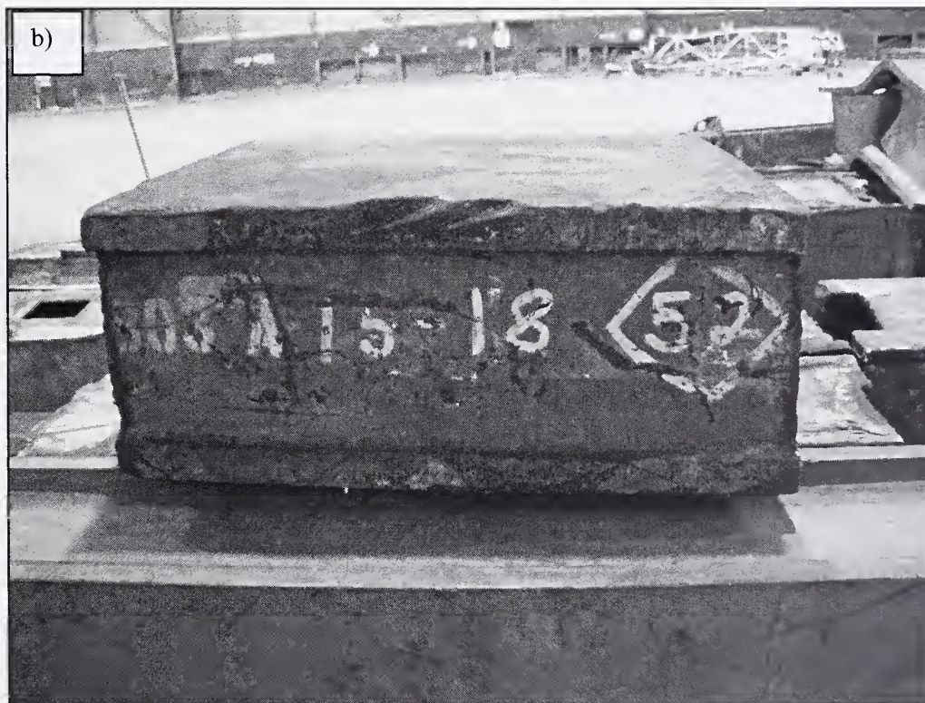
Figure 3–12. Core columns recovered from WTC 1. a) B-1011 (508A: 51–54), lower 2 ft to 3 ft of built-up box column, b) B-6152-1 (803A: 15–18), lower 3 ft of built-up box column.
