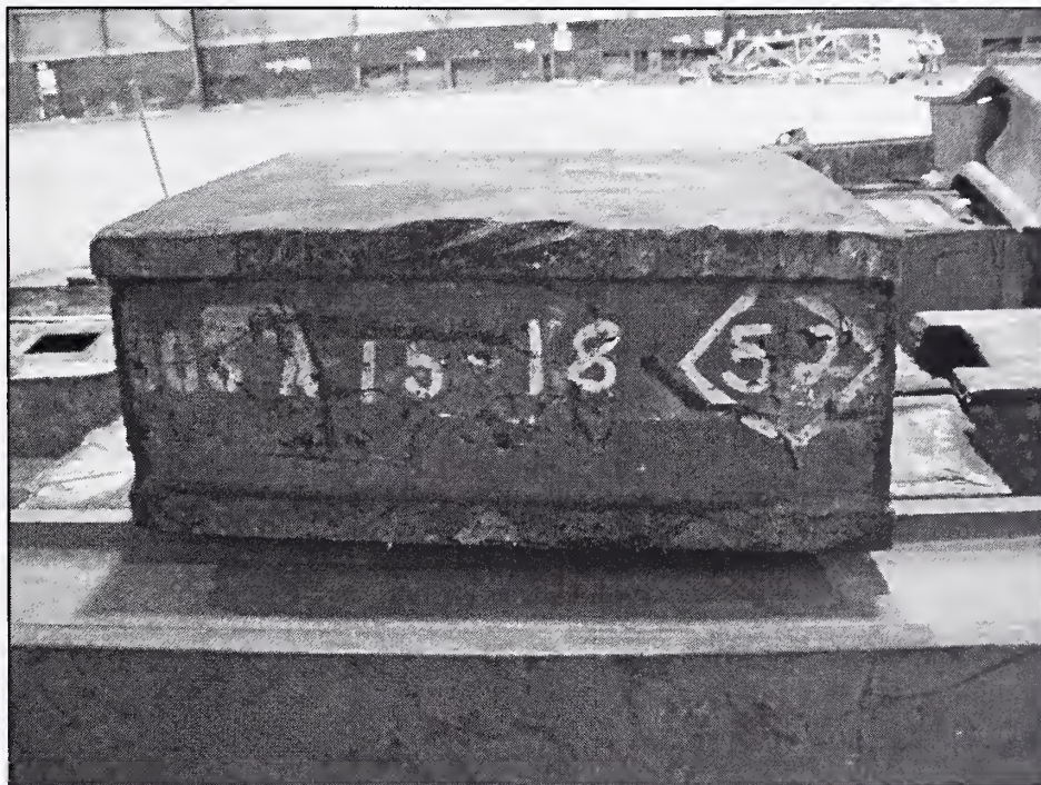
Figure 3–6. (a) Characteristic stenciling found on the lower portions of the exterior column panels for sample C-14. (b) Characteristic stenciling found on an interior core column for sample B-6152.
