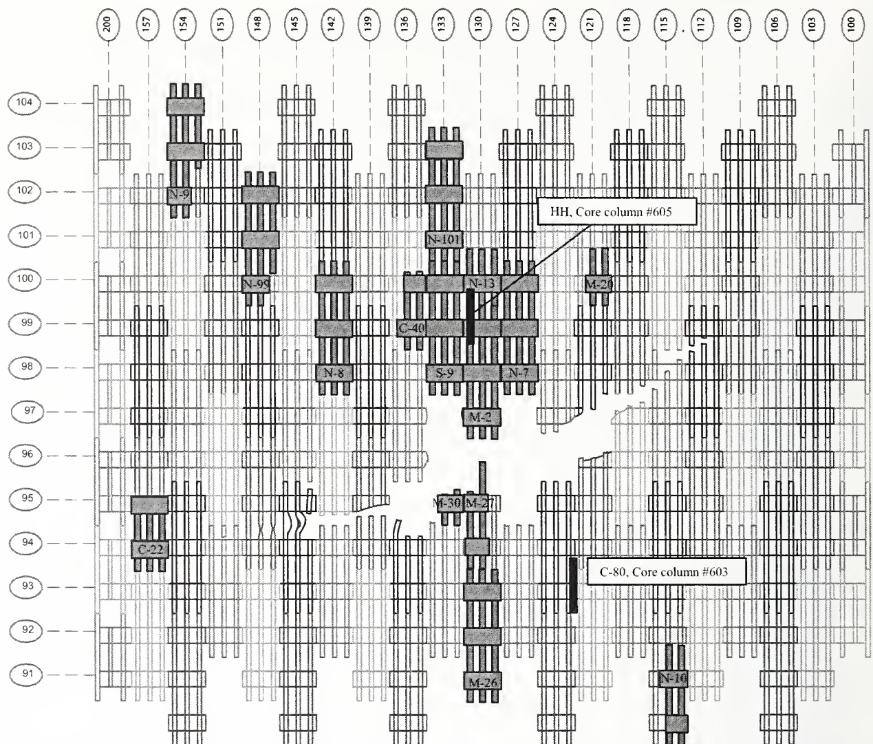
Figure 4–1. Interpreted column damage, from photographic evidence, to WTC 1, with overlay of samples in NIST’s possession. Samples shown represent recovered portions. Core columns 603 and 605 are in the second row from the north face of WTC 1.
