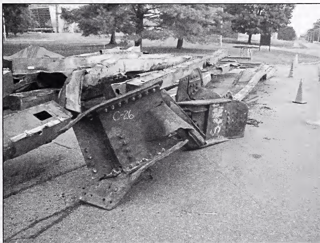
Figure 3–14. Structural element composed of three wide flange sections bolted together. The component was found to be from the framed floor area outside of the core on the 107th floor of WTC 1 (sample was C-26).
