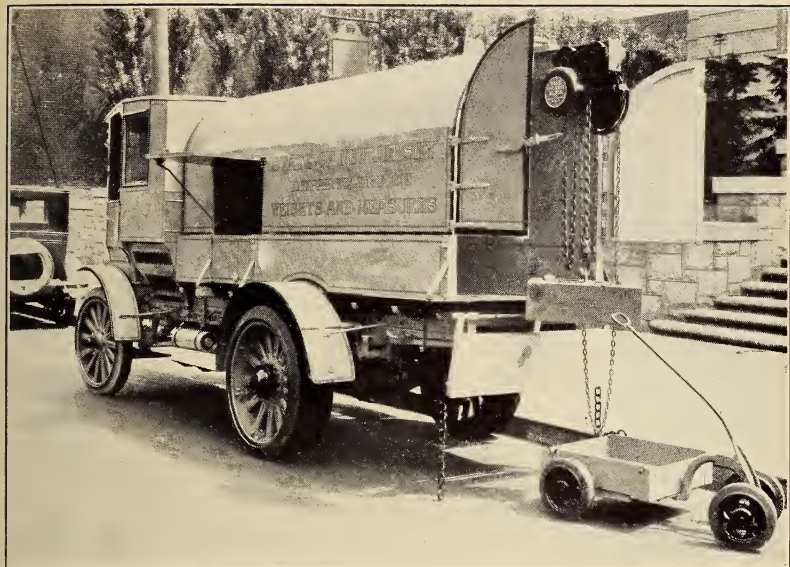
FIG. 2.—New Jersey equipment for testing large-capacity scales
