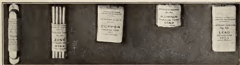
FIG. 29.— Standards for temperature fixed points (Freezing points)
