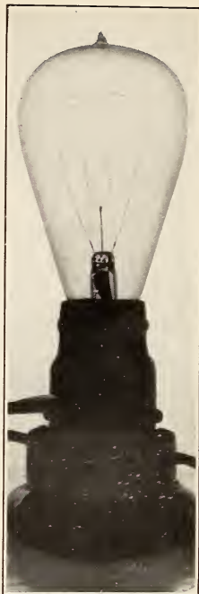
FIG. 31.— Standard of total radiation (Radiant energy)
