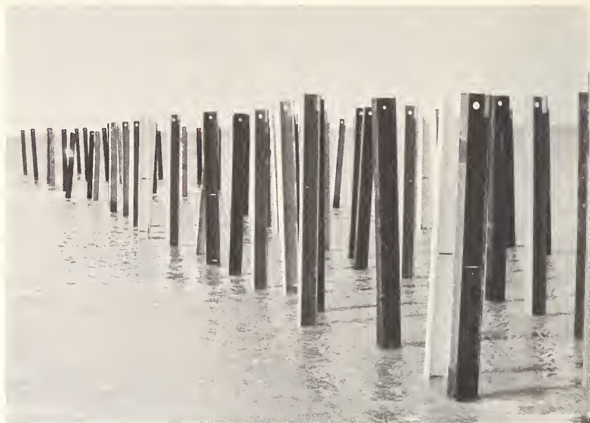
These steel piles with protective coatings were driven into the Atlantic Ocean floor to study the best means of protecting pilings in seawater.
