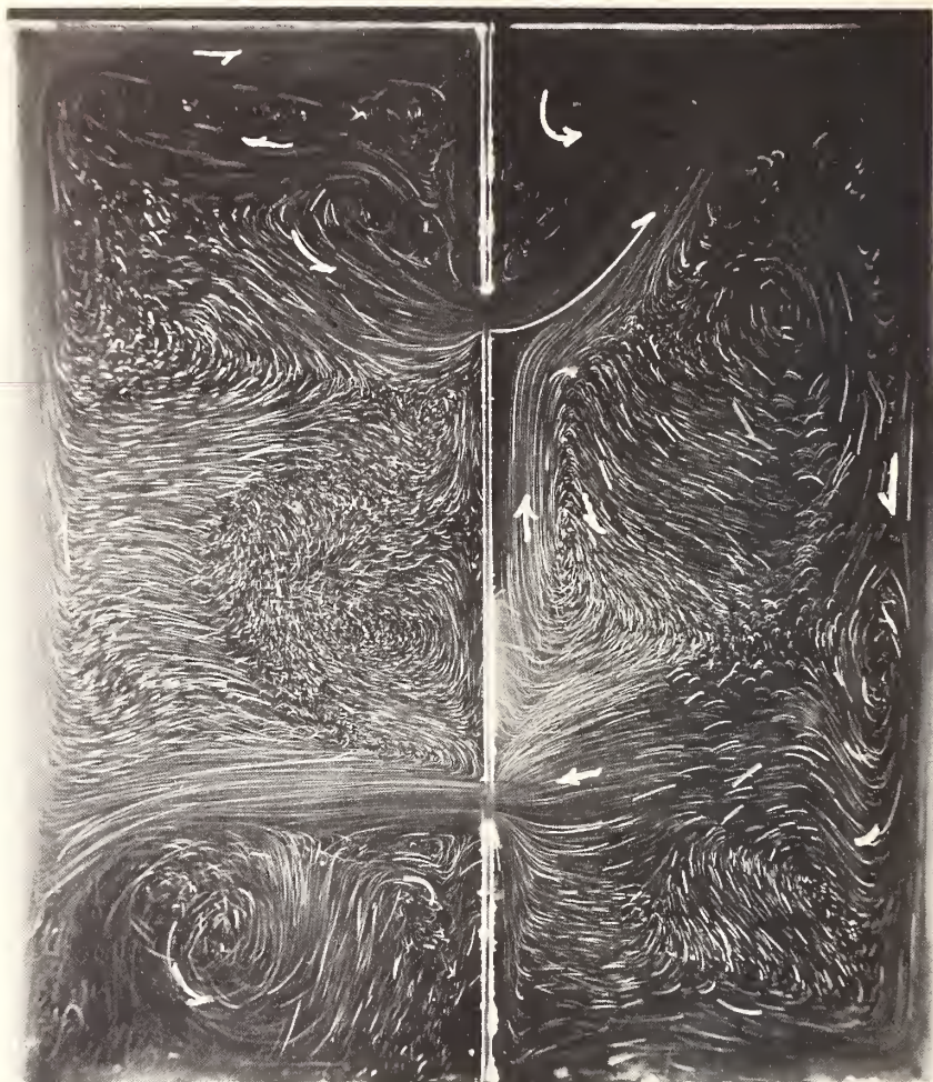
To study the flow of air within and between adjoining rooms, lightweight dust is introduced into a model room and patterns of motion are photographed. The pattern above shows airflow through two narrow openings in a partition. The wall to the far left is heated; that to the far right, cooled.
