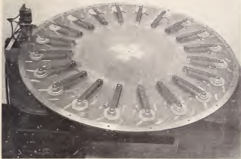
Automatic changer for the calibration of twenty gamma-ray point sources.
