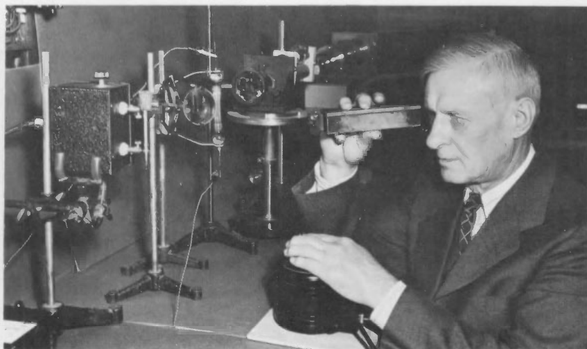
Dr. Meggers observing the spectral line of the mercury isotope of mass 198, a potential basis for an atomic standard of length.
