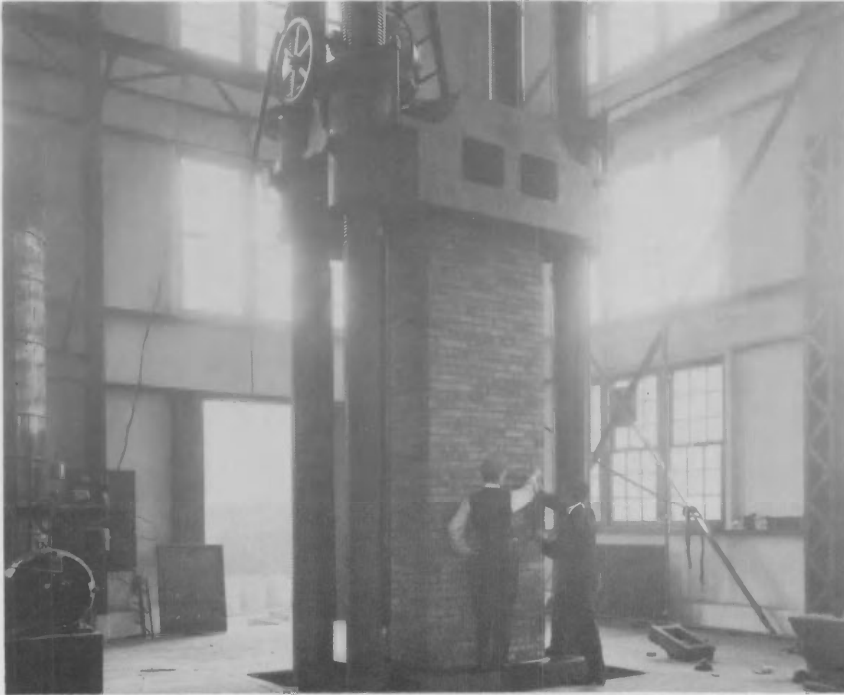
The 2,300,000-pound Emery testing machine in Washington, for making exhaustion tests of beams, girders, and other large metal structural components. A similar compression-to-exhaustion giant, the Olsen machine, was at the Pittsburgh laboratories, for destruction tests of piers and other masonry columns.
