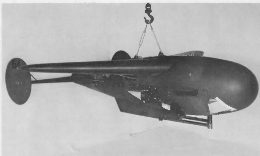
The "Pelican," developed with the cooperation of the Navy Bureau of Ordnance and the MIT Radiation Laboratory. Here it is rigged with instrumentation for flight tests, the 16 mm gunsight aiming point camera directly beneath the wing pointing at a panel of signal lamps indicating radar controls being applied, and the 16 mm camera, slightly lower and forward, pointing at the ground ahead of the glider.
