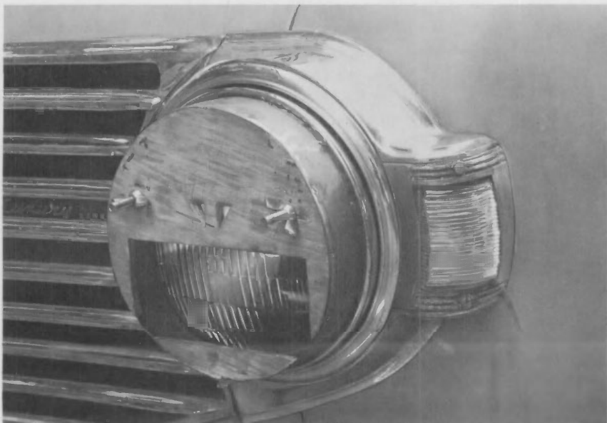
A mockup mask devised at the Bureau for cutting the upward glare of sealed beam headlights, one of dozens of such blackout or brownout devices to reduce skyglow over the coastal cities in the first years of the war.
