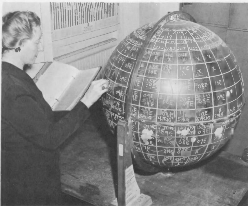
Recording radio-weather forecasting data as a preliminary to preparing monthly predictions of ionospheric and radio conditions. Systematic measurement of the height and density of the ionospheric layers, the highly electrified region of the upper atmosphere produced by solar radiation and greatly influenced by high-speed particles discharged from the sun, is basic in the predicting of radio weather.
