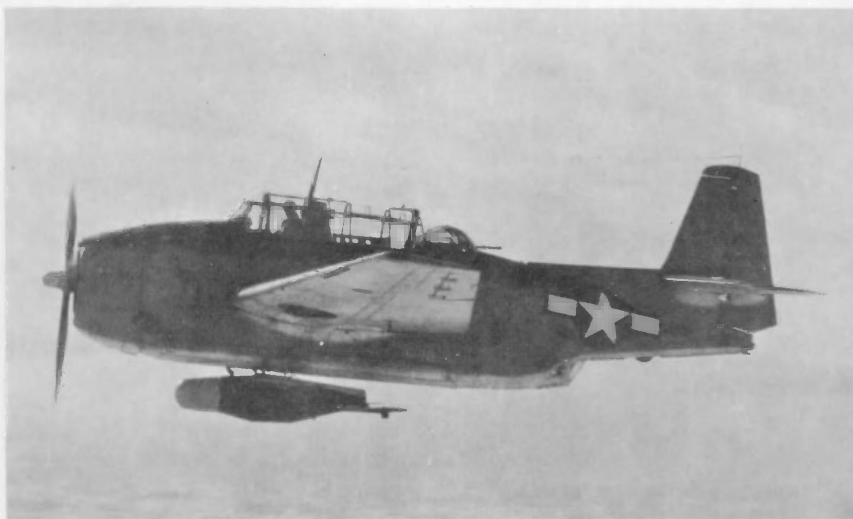
The "Bat," borne by a Navy torpedo bomber, rides with folded tail fins until, upon release, they open into proper flight position.
