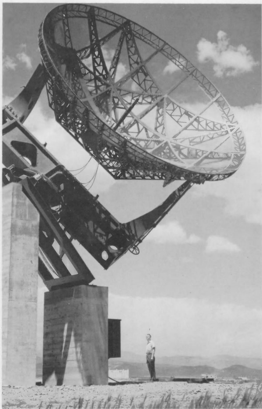
One of the three giant Wurtsburg antennas at the Bureau's Gun Barrel Hill, Colorado, field station. Used in radio propagation research, a dipole at the focal point of the paraboloid reflector receives radio energy from the sun.
