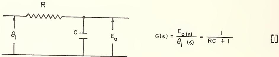
Fig. 8 An Electrical R-C Filter Circuit
