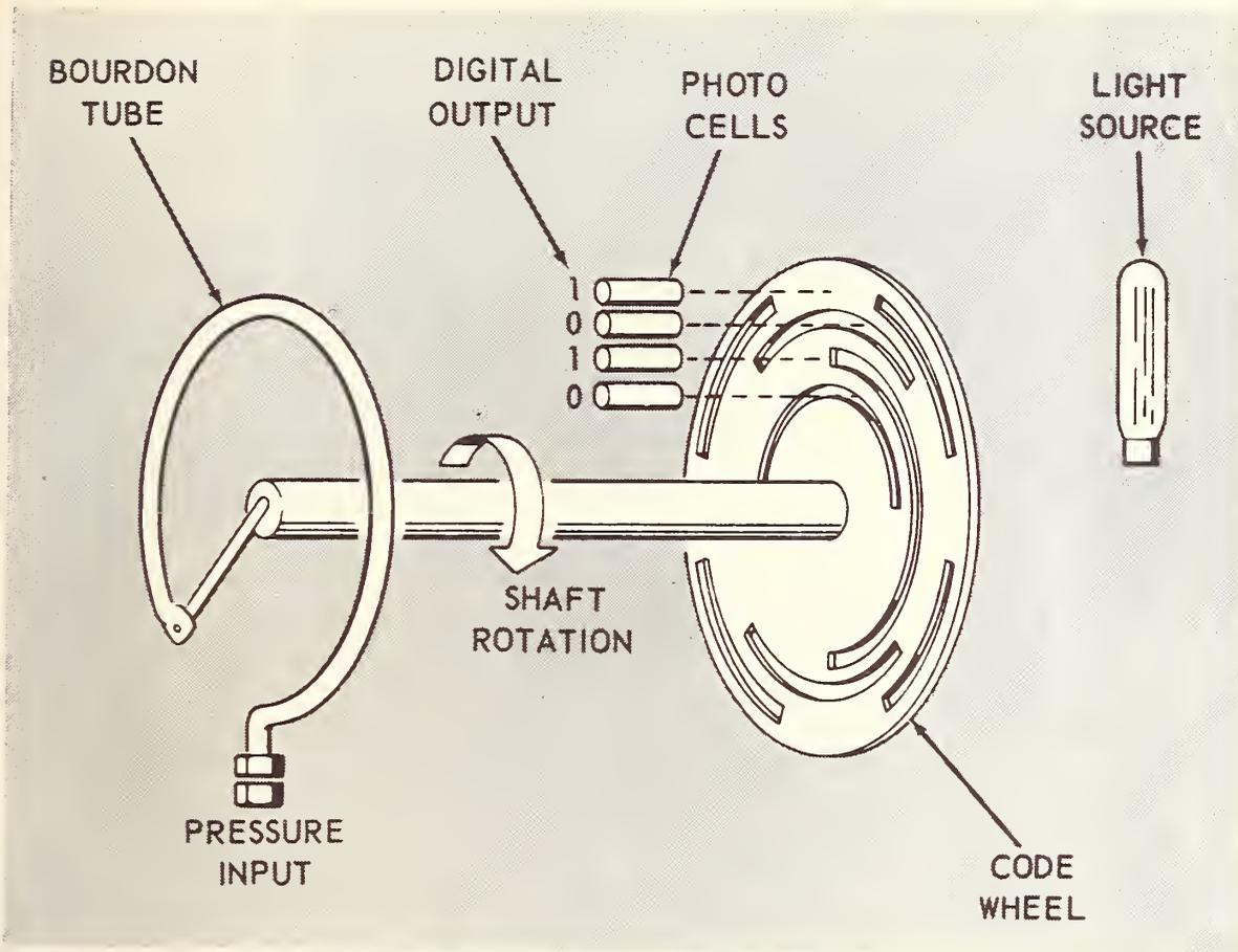
Figure 5. Transducer/Encoder Mechanism
