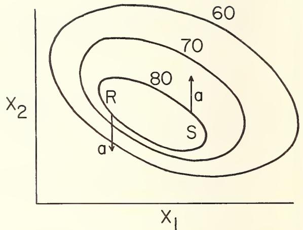
Figure 2. Contours of equal response in a two variable plane.
