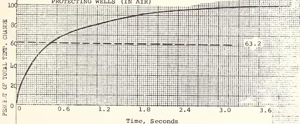
FIG. 10 SPEED OF RESPONSE OF A RADIATION DETECTOR
