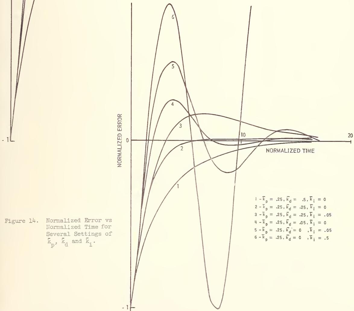
Figure 14. Normalized Error vs Normalized Time for Several Settings of  $\bar{k}_p$ ,  $\bar{k}_d$  and  $\bar{k}_i$ .
