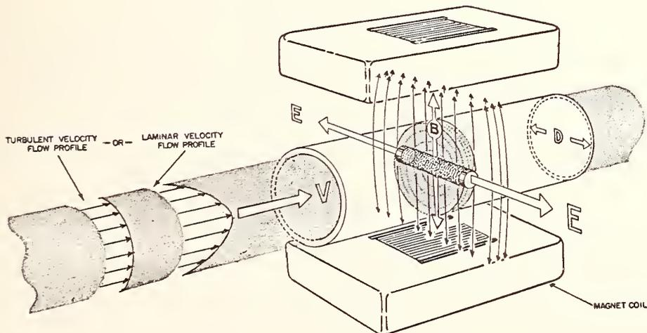
Fig. 33 Principle of Magnetic Flow Meter
