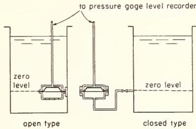
Fig. 36 Liquid Level Measurement by Diaphragm Method
