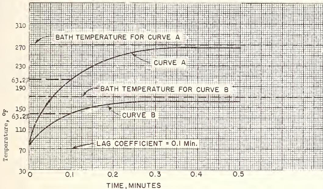
Fig. 2 Speed of Response of Thermometer Bulb
