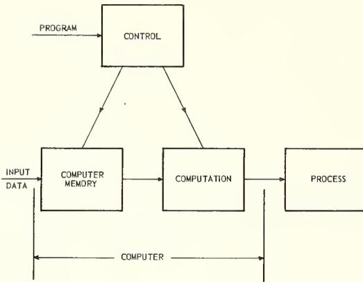
Figure 15. Block Diagram Showing Open Loop Computer Operation.
