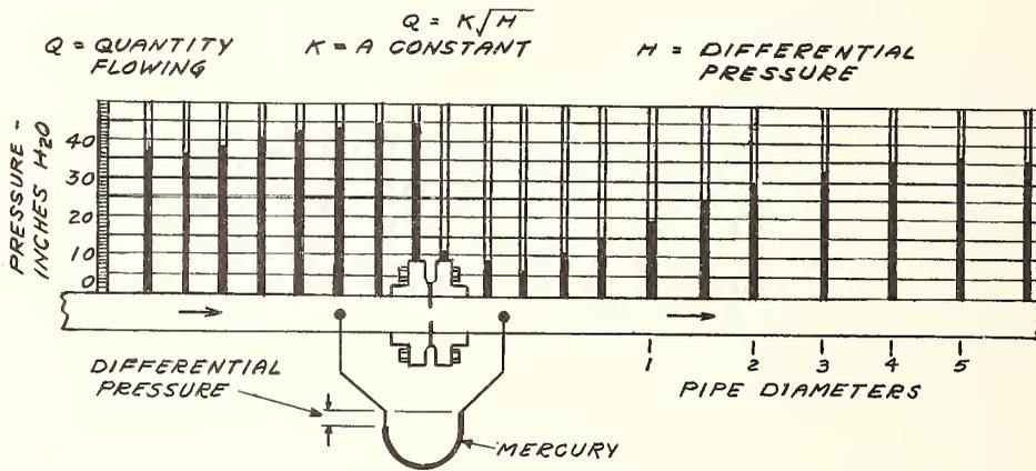
Fig. 24 Differential Pressure Across an Orifice
