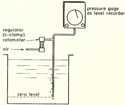
Fig. 39 Liquid Level Measurement by Air Purge Method
