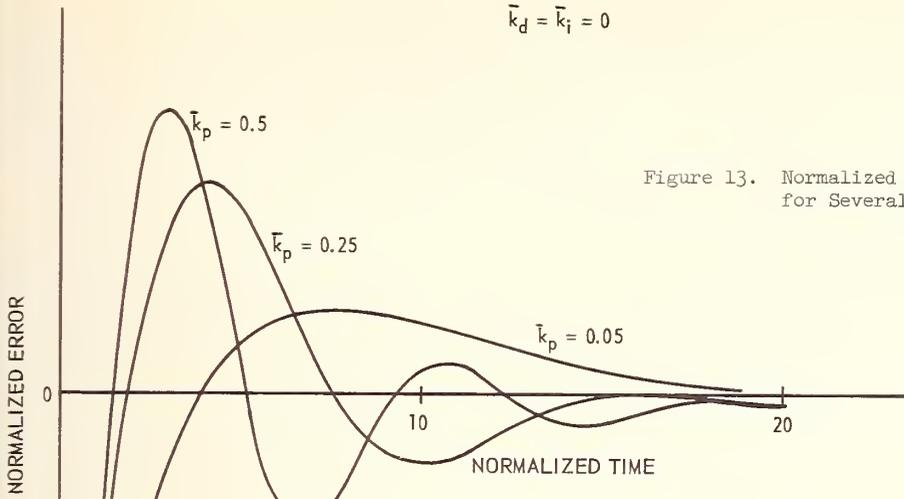
Figure 13. Normalized Error vs Normalized Time for Several Gain Settings.
