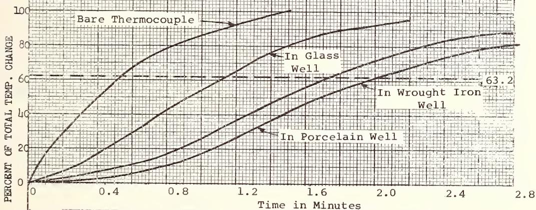
FIG. 9 SPEED OF RESPONSE OF THERMOCOUPLE, WITH & WITHOUT PROTECTING WELLS (IN AIR)
