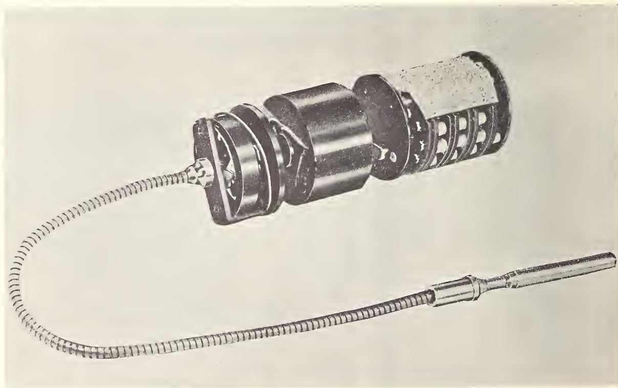
Figure 4. Temperature Transducer/Encoder
