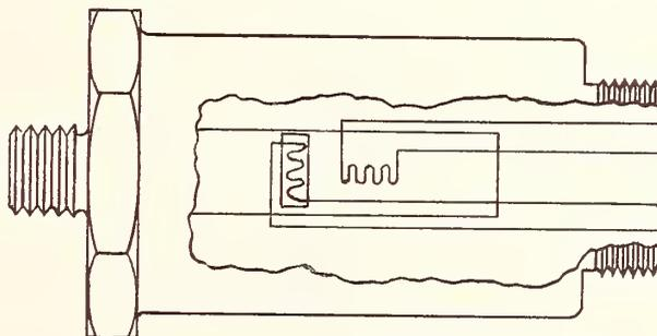
Fig. 19 An Electrical Pressure Transducer
