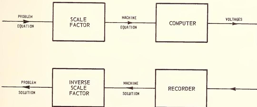
Figure 1. Basic Steps in Using an Analog Computer.
