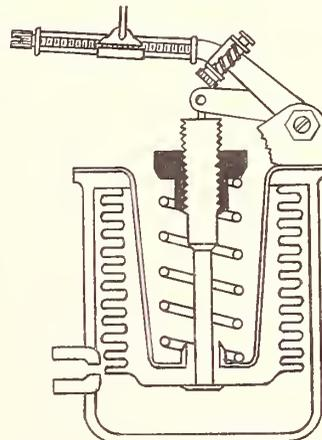
Fig. 15 Spring and Bellows Assembly for Vacuum Measurement
