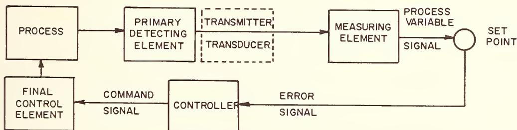
Fig. 1 Block Diagram of Closed Loop Control System
