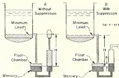
Fig. 37 Liquid Level System with and without Suppression
