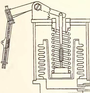
Fig. 14 Spring and Bellows Assembly for Pressure Measurement
