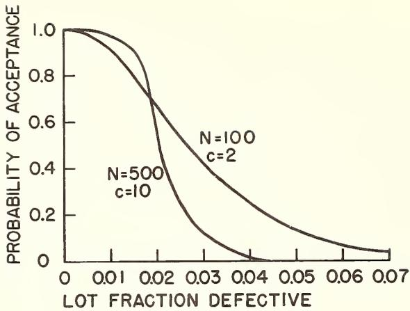
Figure 9. Operating characteristic curves for different sample sizes.
