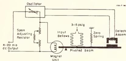
Fig. 45 Method of Operation P/1 Transducer
