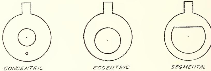
Fig. 20 Orifice Plates
