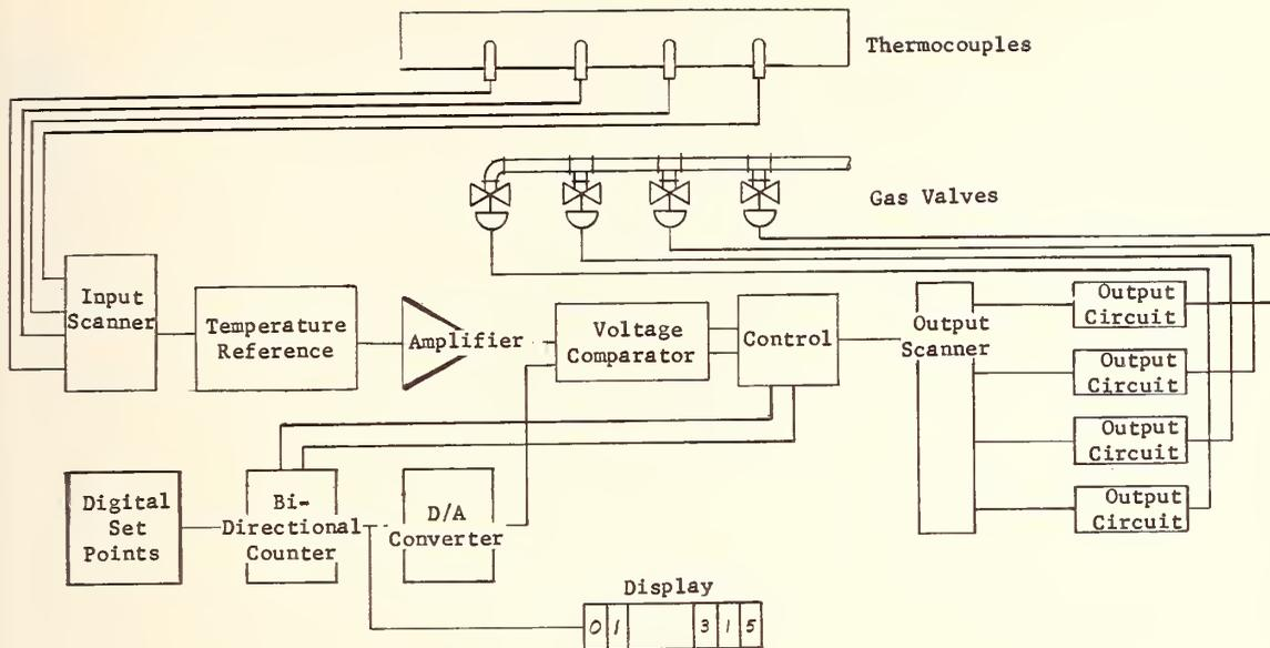
Figure 13. Temperature Control System with Digital Control
