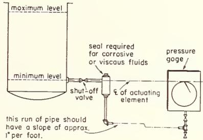
Fig. 35 Liquid Level Measurement by Pressure Gage Method
