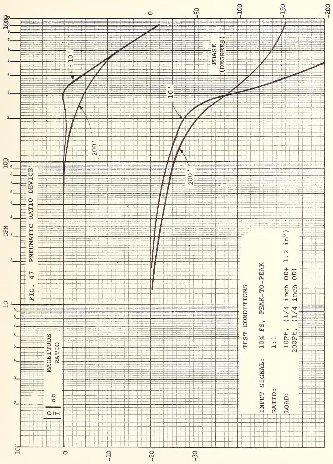
FIG. 47 PNEUMATIC RATIO DEVICE
