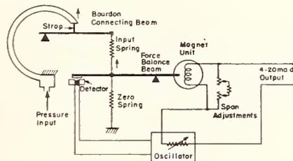
Fig. 44 Method of Operation, PP/1 transmitter
