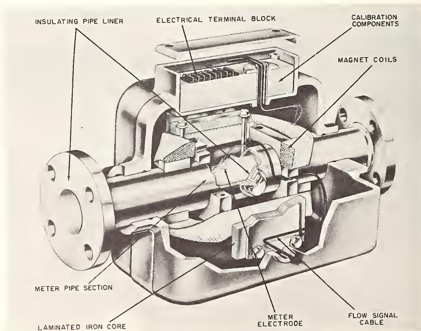
Figure 8. Magnetic Flow Meter (Courtesy Fischer & Porter Company)
