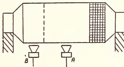
Fig. 40 Liquid Level Detection by Noise Level Measurement
