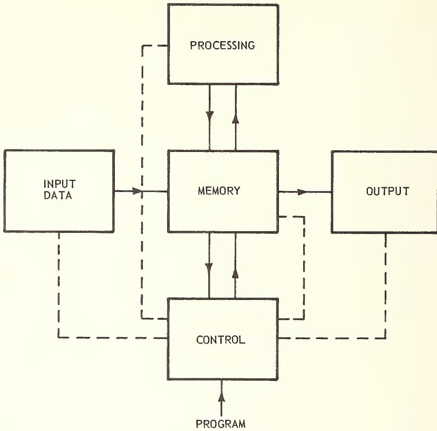
Figure 2. Basic Steps Performed by a Digital Computer.
