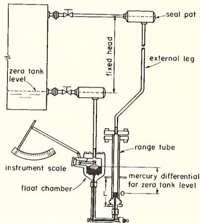
Fig. 38 Liquid Level Measurement in Closed Vessel
