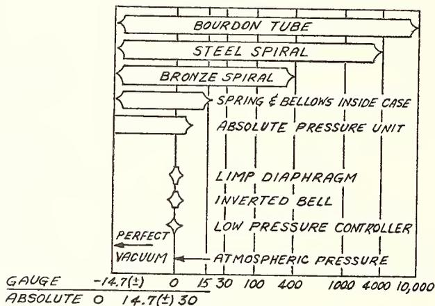
Fig. 11 Application Chart of Pressure Measuring Devices
