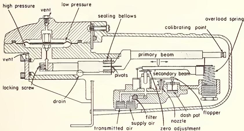
Fig. 29 Differential Pressure Converts, Force-Balance Type
