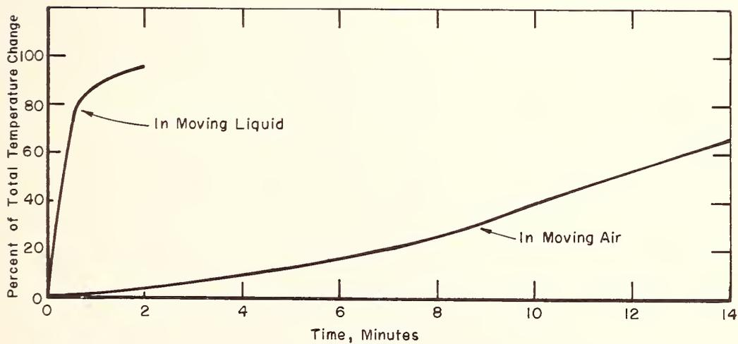
Fig. 7 Speed of Response of Resistance Thermometer Bulb
