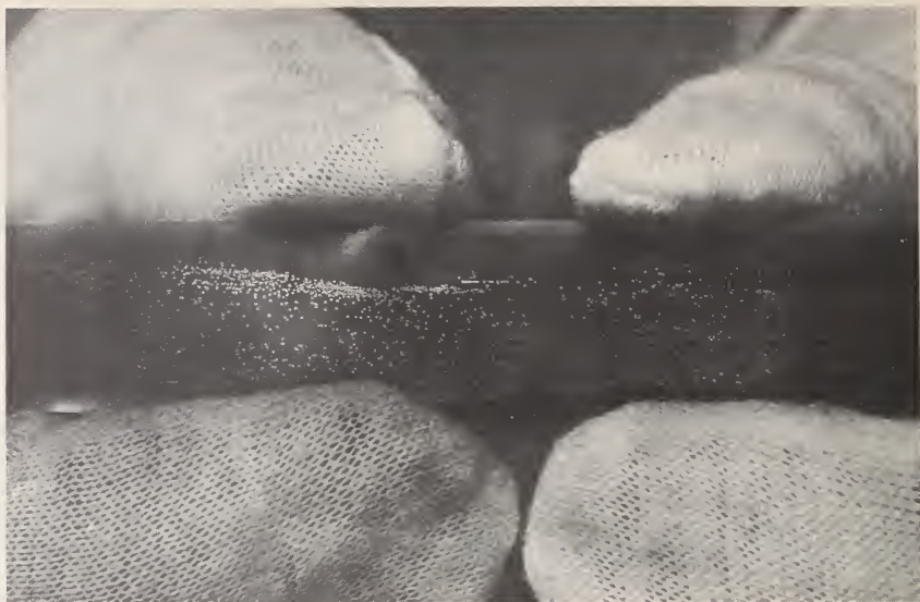
Aging blemishes on the leader of a 16 mm microfilm. The causes for the appearance of these spots on microfilm records, and possible corrective measures, are currently the subject of an intensive investigation. (See page 53)
