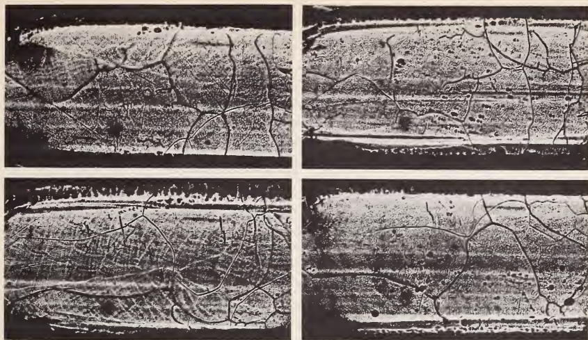
Four sides of a methane crystal at 87 °K seen through liquid argon. The heavy lines are grain boundaries on the back faces of the crystal and the lighter ones are grain boundaries on the front faces. These crystals provide excellent sources for spectroscopic, solid state, and surface physics studies at low temperatures. (See page 154)
