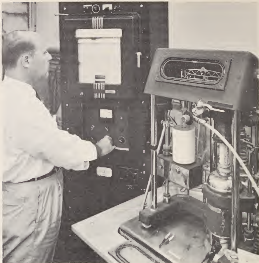
An electronic thermogravimetric balance used to detect changes in weight of coordination polymer samples as they are heated in a vacuum furnace (extreme right). The measurements obtained are an indication of polymer thermal stability. (See page 138)
