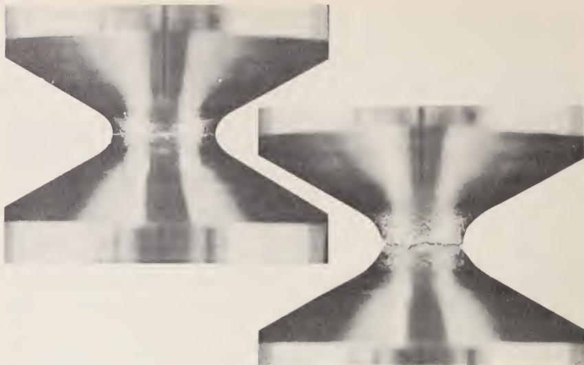
Notch geometry is extremely useful in studying the origin and propagation of metal fractures. Here, a tensile specimen of 310 stainless steel cracks under a true strain of 0.22 (left). Crack has grown under strain of 0.8 (right) just prior to the rapid final fracture of the specimen. (See page 140)
