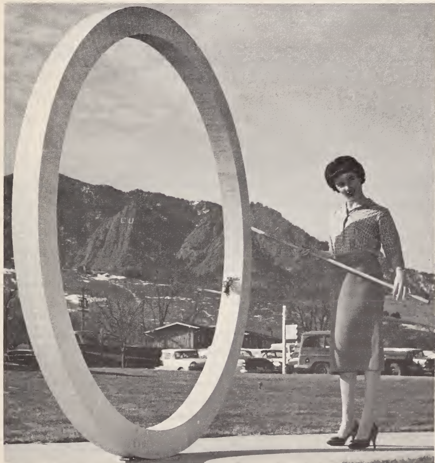
Two-meter diameter antenna of 16,000 turns used for ultra-low-frequency studies. This includes observations of the electromagnetic field environment, seeking its geophysical source, and understanding propagation from distant natural sources. (See page 202)
