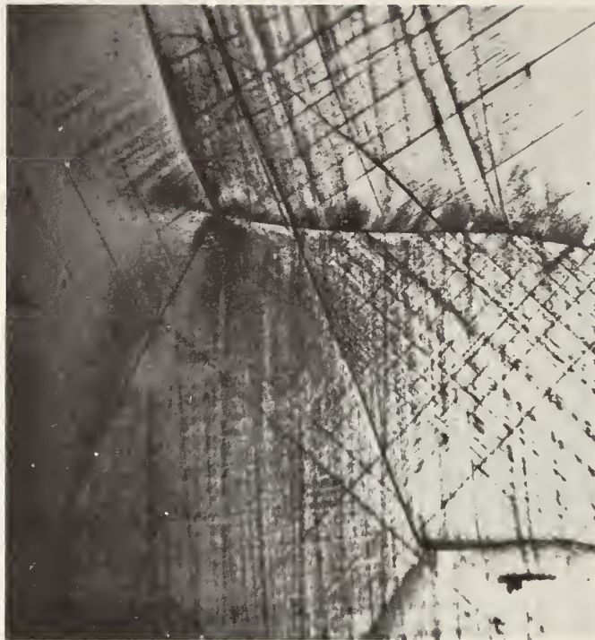
Figure 11. Slip distribution in the vicinity of grain boundaries in lithium fluoride deformed at room temperature. Note very local slip on {001} planes near triple point. Slip revealed by etch pit technique. (courtesy W. D. Scott and J. A. Pask).
