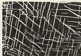
FIGURE 8. Widmanstätten structures. Example: \text{UC}_2 (bright) in \text{UC} (X281). [Chang, R., and C. G. Rhodes, "High-Pressure Hot-Pressing of Uranium Carbide Powders and Mechanism of Sintering of Refractory Bodies," J. Am. Ceram. Soc. 45 , 379 (1962)].
