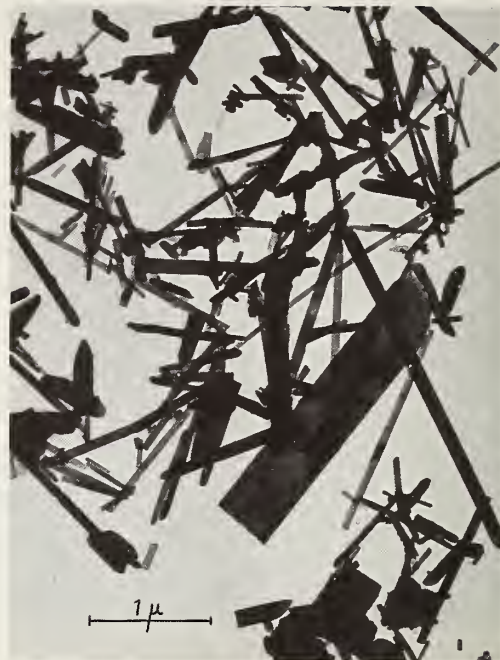
FIGURE 8. Isolated and dispersed mullite phase of an insulator porcelain.
