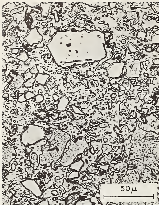
FIGURE 3. Vitreous sanitary ware (etched 10 sec, 0 °C, 40% HF, collodion replica).
