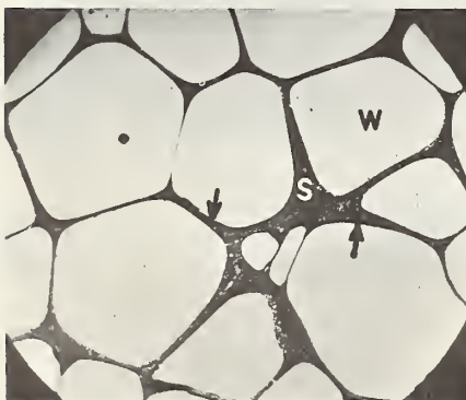
FIGURE 29. Microstructural-controlled behavior. Example: wüstite ( \text{FeO} ) and a silicate matrix. This matrix was liquid at the equilibrating temperature and subsequently has crystallized to fayalite ( \text{Fe}_2\text{SiO}_4 ) and more wüstite (approx. X84). The crack is in the silicate matrix, but is closely associated with the silicate-wüstite boundary. W - wüstite; S - silicate liquid; Arrow - crack.
