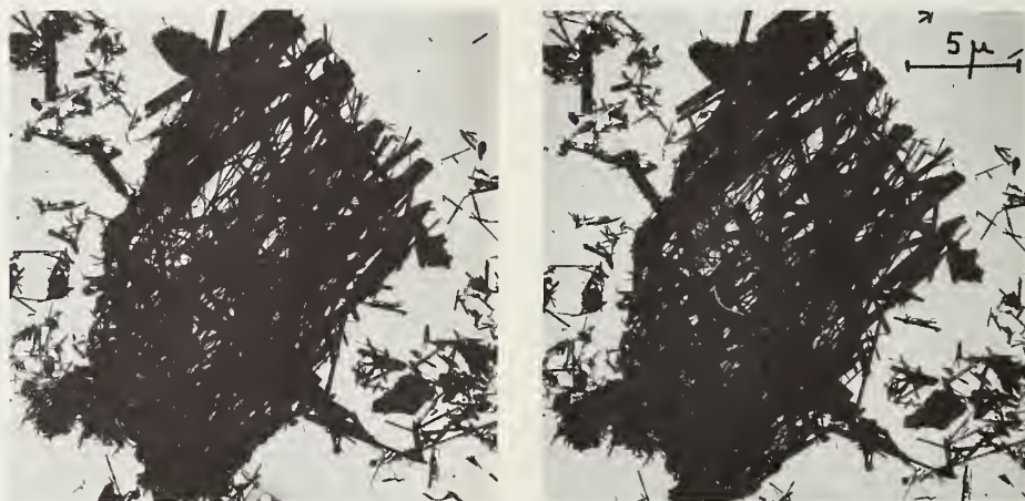
FIGURE 9. Stereoscopic views of a part (the large aggregate) of the mullite phase from a feldspar relict region showing the magnitude and relative position of the mullite crystals. To the left some smaller, more compact aggregates from clay relicts can be seen.
