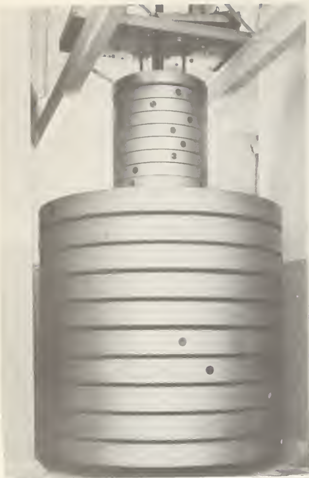
Figure 9. Weights and lower part of the 111,000-lb capacity dead-weight machine.
