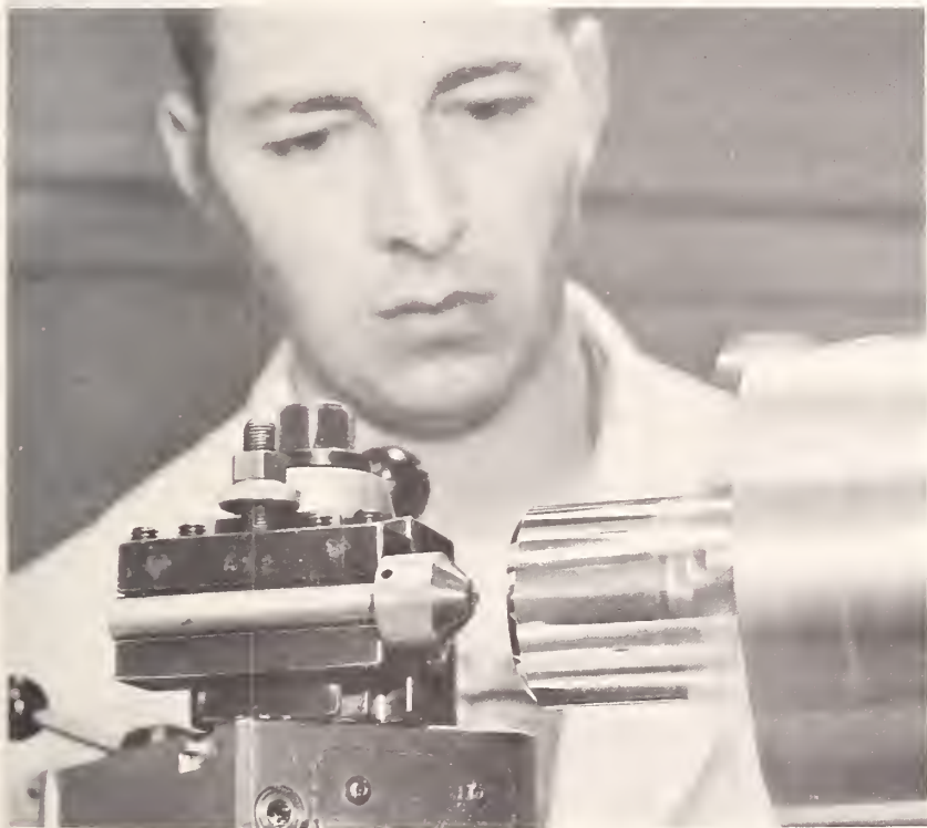
Diamond burnishing was shown to give the necessary high surface finish to standard weights. The process eliminates much of the time consuming and costly polishing previously necessary in production. (See p. 28.)
