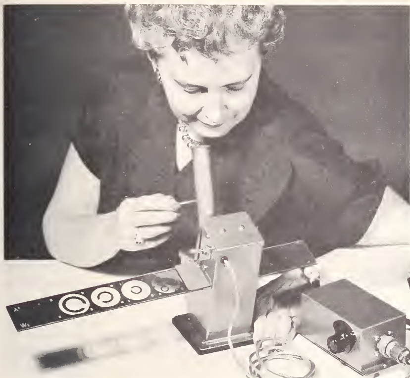
An image-glossmeter was developed to measure the image-forming properties of a surface. Image-gloss is an important attribute of some types of building exteriors. (See p. 167.)
