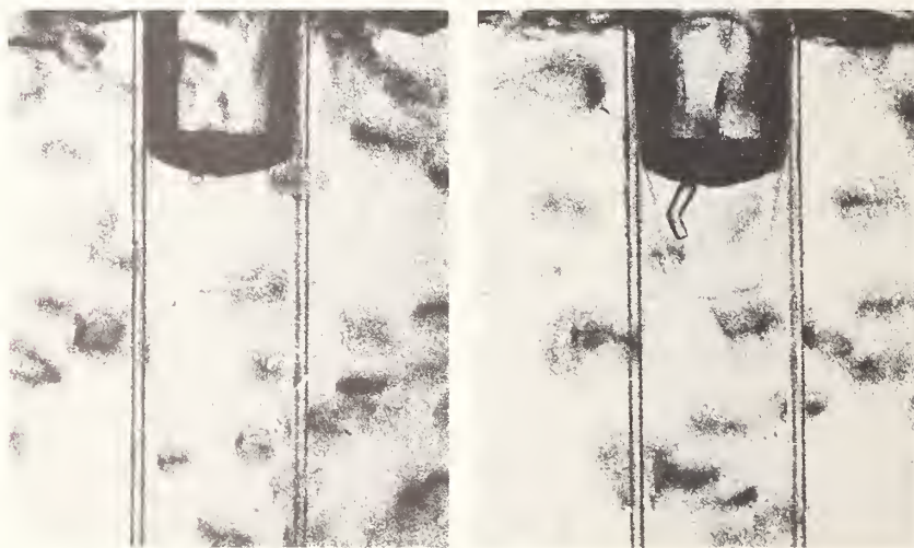
"Vapor snake" growing in crystallizing argon. Starting with a bubble at the surface of the melt (left) the snake grows downward as a vapor-filled solid sheath (right). This unusual phenomenon is shedding much light on the fundamental crystallization processes in the rare gases. (See p. 93.)
