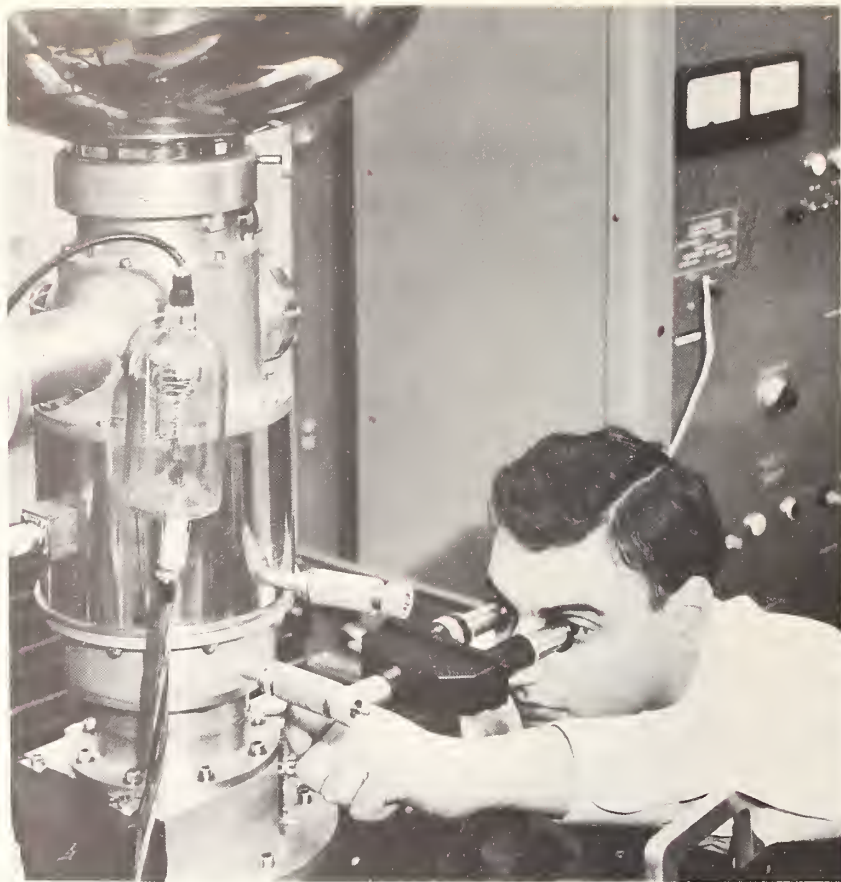
The NBS-developed electronprobe microanalyzer performs a nondestructive quantitative chemical analysis on a preselected, 1-micron diameter spot of a metal specimen. An optical system permits simultaneous visual observation of the spot being irradiated and analyzed. (See p. 98.)
