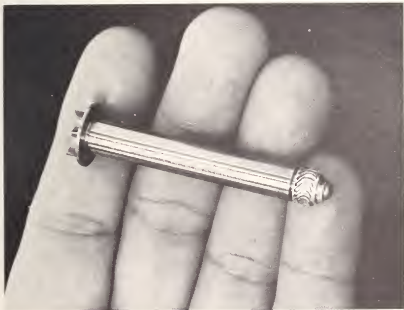
Miniature high-speed turbine expander is a vital component in a cryogenic refrigeration system. The turbine rotates at speeds up to 9000 revolutions per second. The shaft is supported by hydrostatic helium gas-lubricated bearings. (See p. 156.)
