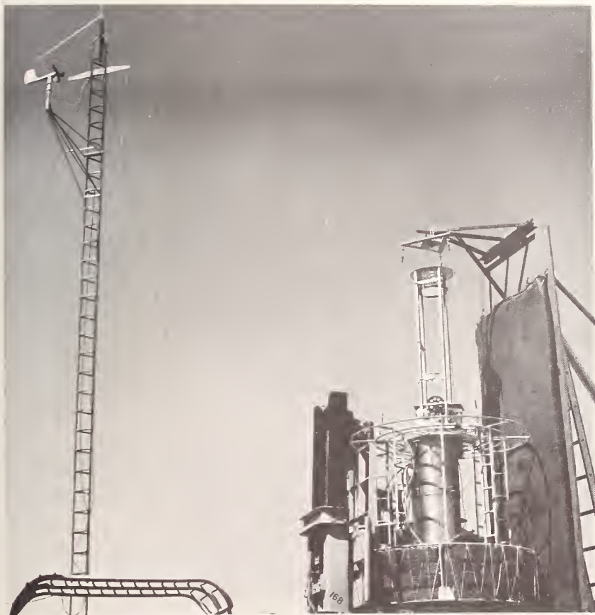
Balloon-borne spectrometer used to measure the composition of the atmosphere by means of its infrared absorption spectrum. The sun serves as the infrared source.
