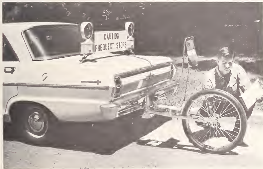
Checking the fifth wheel distance-measuring device used to obtain information regarding the accuracy of vehicle odometers. The investigation is designed to provide car-rental agencies with accuracy requirements, and to provide weights and measures officials with a performance code, testing equipment design, and test methods. (See p. 170.)
