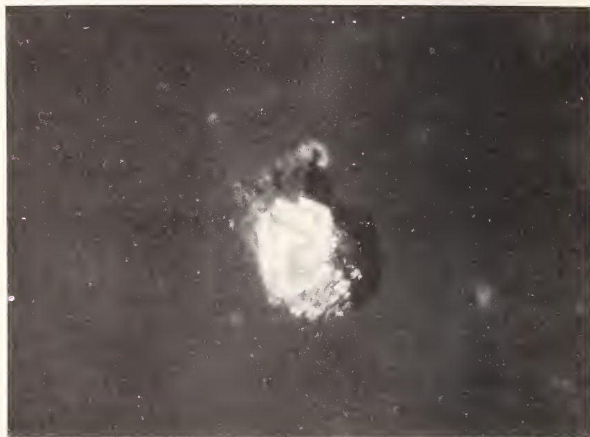
Diamond grown in multi-anvil (tetrahedral) apparatus at a temperature of 3000 °F and one million pounds per square inch pressure. This work is aimed at establishing fixed reference points on the pressure scale (page 30).
