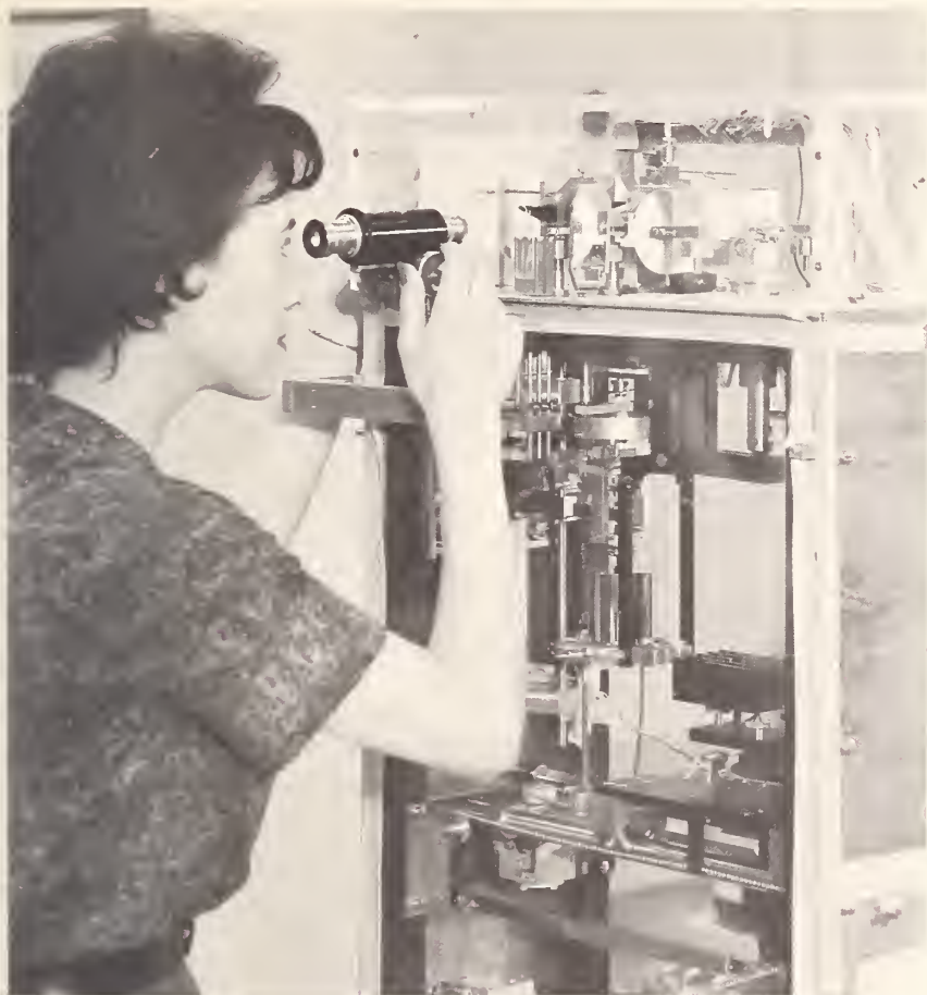
Experimental one-pan balance designed to investigate the limitations of such an apparatus in experiments where the maximum attainable level of precision is demanded—work with the National Standard Kilogram, for example (page 22).
