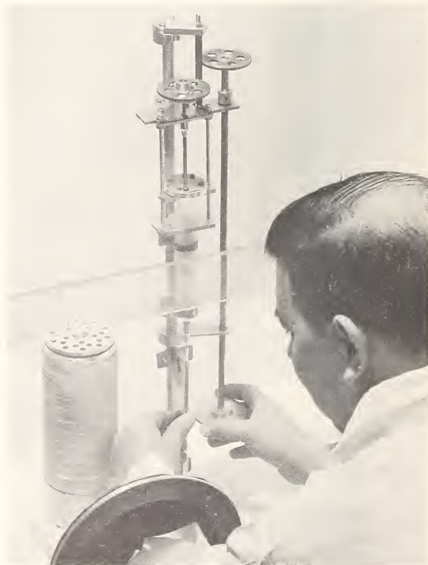
Eight new standard hydrocarbon blends were issued for calibrating instruments used to analyze gasoline and blending stocks. Ampoules are filled in a controlled atmosphere with sufficient blend for one calibration (page 75).
