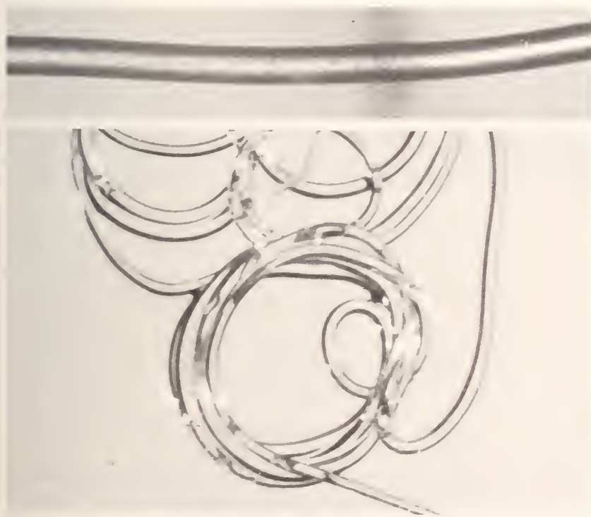
Nylon fiber (above) develops helical coils (below) after chemical treatment. Such artificially induced structural changes may lead to fibers which will resist extreme environmental conditions (page 102).
