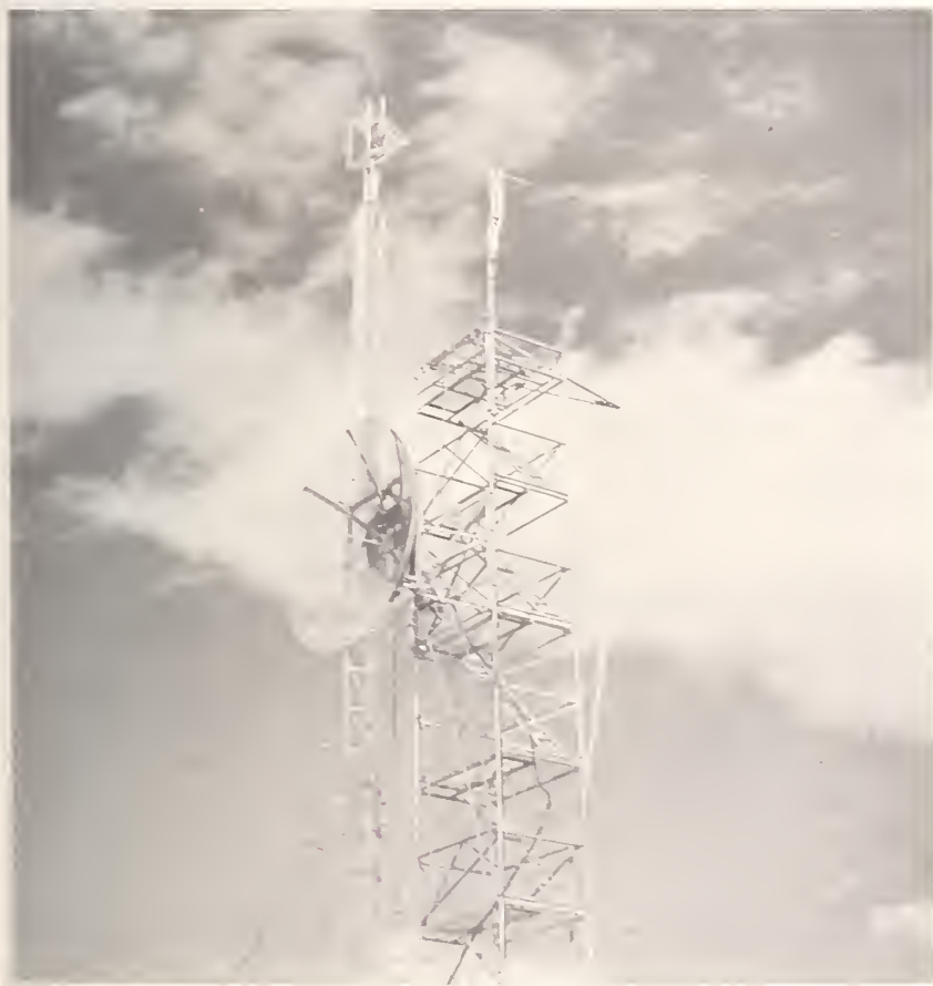
Receiving antennas used in studies of obstacle-gain propagation over Pikes Peak. Under certain conditions, signals propagated across mountain ridges are found to be far stronger than if the obstacle were not there (page 130).
