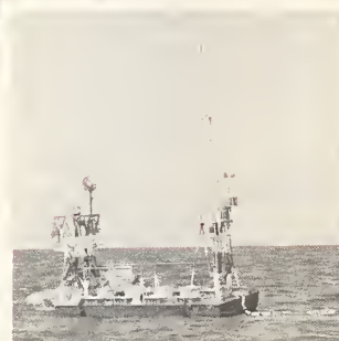
Right: The anchored, unmanned, automatic weather station, "Nomad," developed for the Navy, was the first automatic weather station to detect formation of a hurricane. Above: NBS engineers also helped the Navy to develop and set up a chain of automatic weather stations in the Antarctic (page 120).
