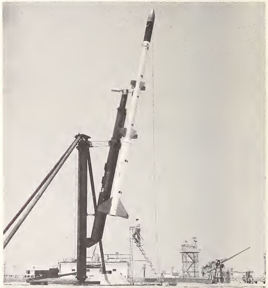
Javelin rocket which carried an ionosonde to an altitude of 1,000 kilometers. For thirteen minutes, the ionosonde made topside soundings of the ionosphere. The experiment was made to test the sounding system for the fixed-frequency satellite topside sounder to be orbited in 1962 (page 127).
