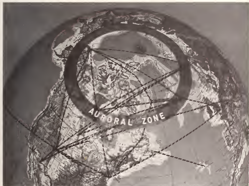
Radio propagation paths under study by the Bureau to provide information on factors affecting the design and use of radio systems. Ionospheric, ground-wave, and line-of-sight paths are investigated to define the limitations, disturbances, and capacity of the transmission medium as a channel (page 128).
