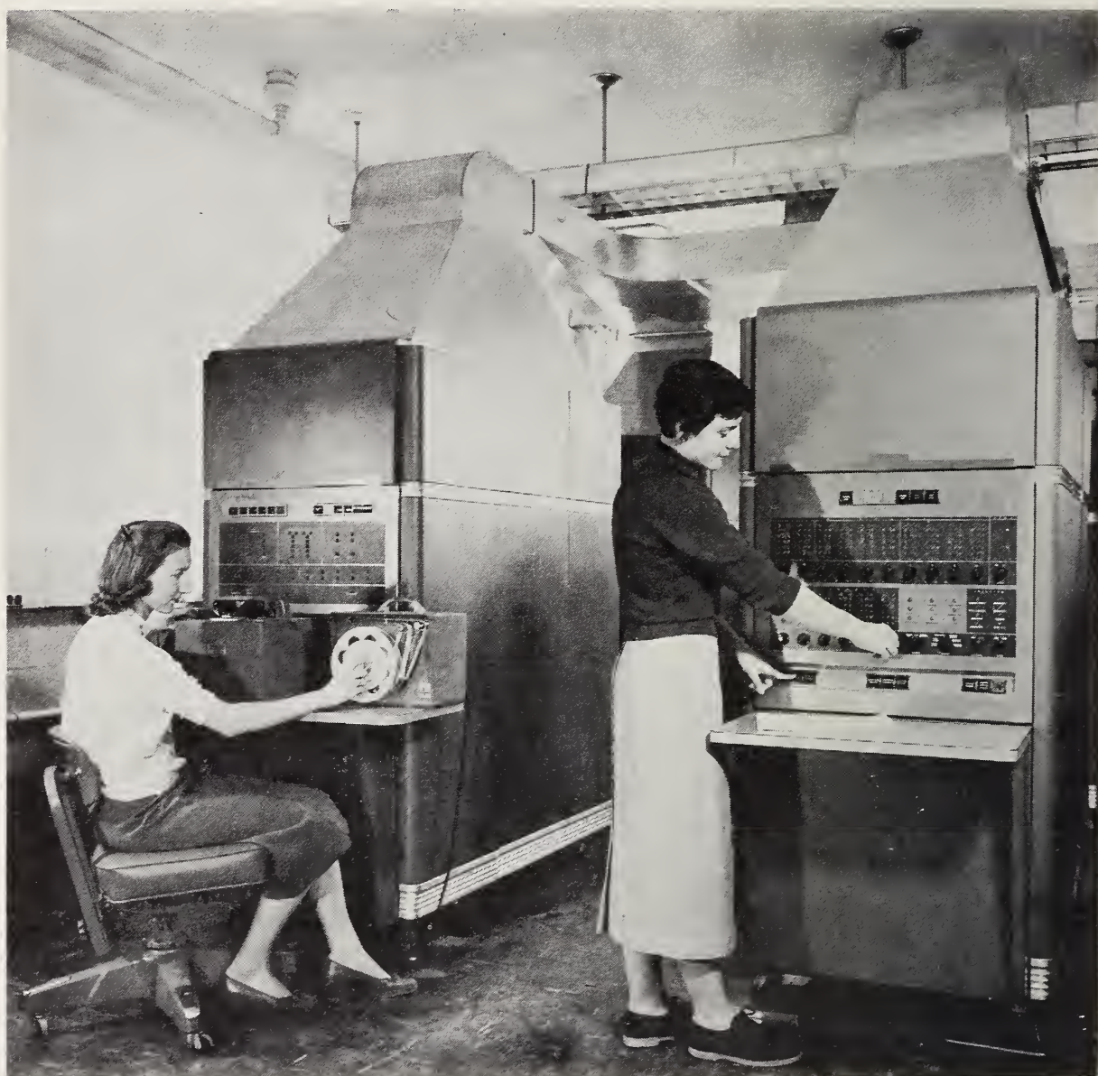
High-speed electronic computers improve speed and accuracy in the preparation of world-wide ionospheric maps (page 111).
