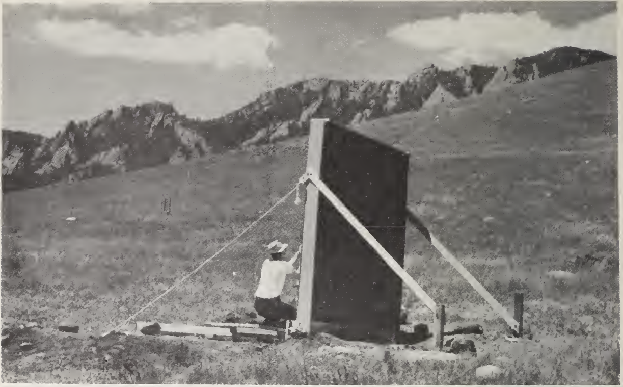
This masonry wall is typical of test structures constructed on the NBS r-f attenuation measurement range to study the transmission of radio waves through buildings and other structures (page 116).
