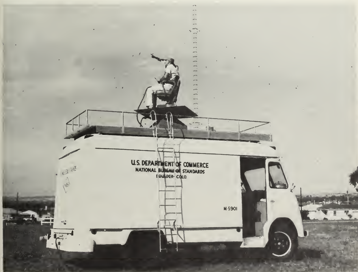
Mobile laboratory containing recording apparatus and roof turntable used to track aircraft in antenna evaluations for the U.S. Air Force (page 121).
