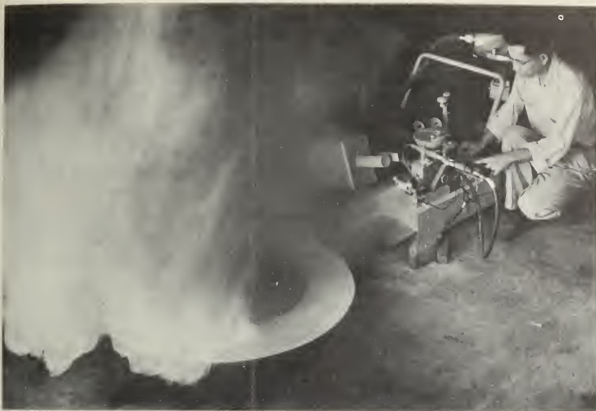
The effectiveness of dry powders in extinguishing fires of flammable liquids was studied (page 89).
