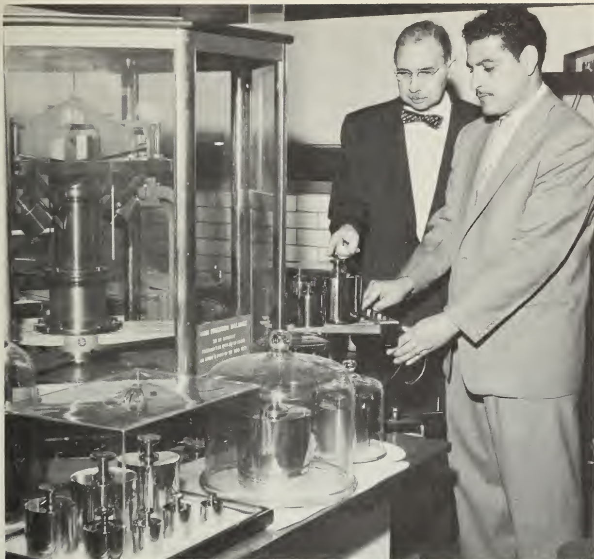
An engineer with the Department of Weights and Measures, National Laboratory of Metrology, Mexico, is instructed in the operation of a large precision balance used for weights up to 25 kg. During the year, approximately 900 foreign scientists and technicians, representing 50 countries, visited the Bureau (page 13).
