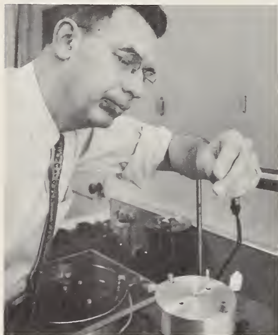
Improvements were made in standards of radioactivity (page 44). Left: A radiation balance is used to measure the rate of energy emission from a radium source used in preparing the new 10^{-9} and 10^{-11} g radium solution standards. Right: Tank of manganese sulfate used as a moderator in calibrations of the National Standard Photoneutron Source.
