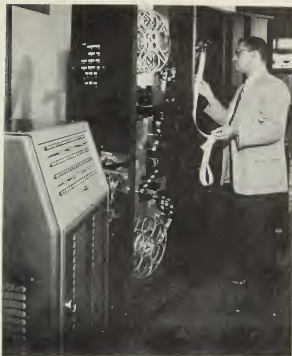
Left: Analog-digital simulator used to study air traffic problems. An airways map of the Washington, D.C., airport appears on the screen. Right: Prototype high-speed document retrieval device handles microfilm at the rate of 2,400 pages of documents per minute (pages 98, 100).
