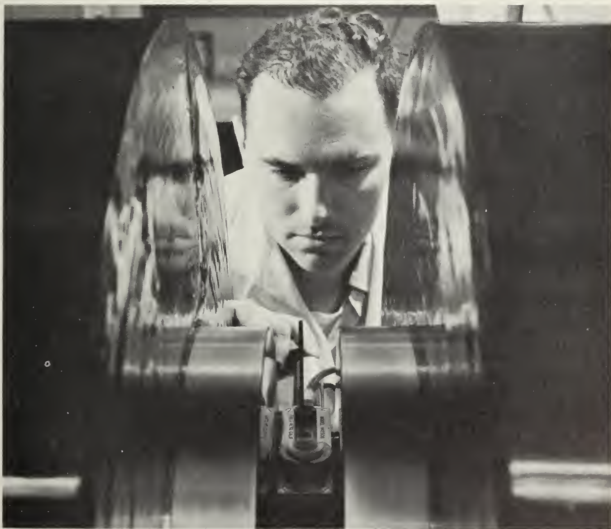
Tuning in on the atomic nucleus. The nuclear magnetic resonance of metals and alloys is studied with the aid of a tuned radio transmitter and receiver. The metal sample is in the probe between the poles of an electromagnet (see page 73).
