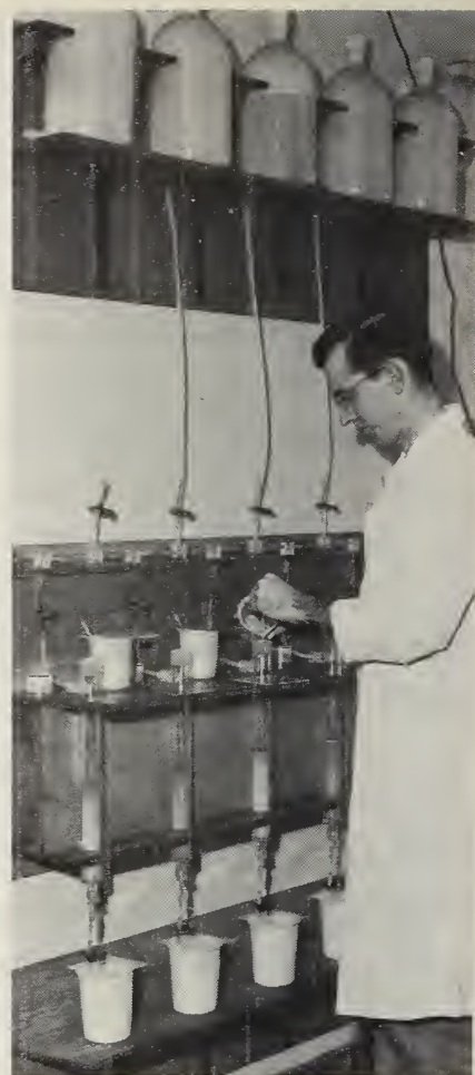
Left: Samples of benzene with controlled amounts of impurity are packaged in a vacuum system. The vacuum transfer system assured the identity of the 42 samples distributed for an international comparison analysis. Right: Analyzing alloys containing minute amounts of titanium, zirconium, niobium, and tantalum. A relatively simple method based on the formation of metal-fluoride complexes was developed for this analysis (pages 51, 49).
