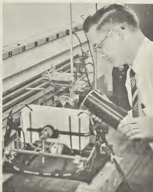
Atomic beam principle (left) used by the Bureau to produce narrow emission lines in research on improved wavelength standards of lengths. A collimated beam of mercury atoms emerging from the oven (below white box in photo) is bombarded by electrons. The atoms thus excited emit light which is then viewed at right angles to the motion of the atoms in order to reduce Doppler broadening (page 25).
