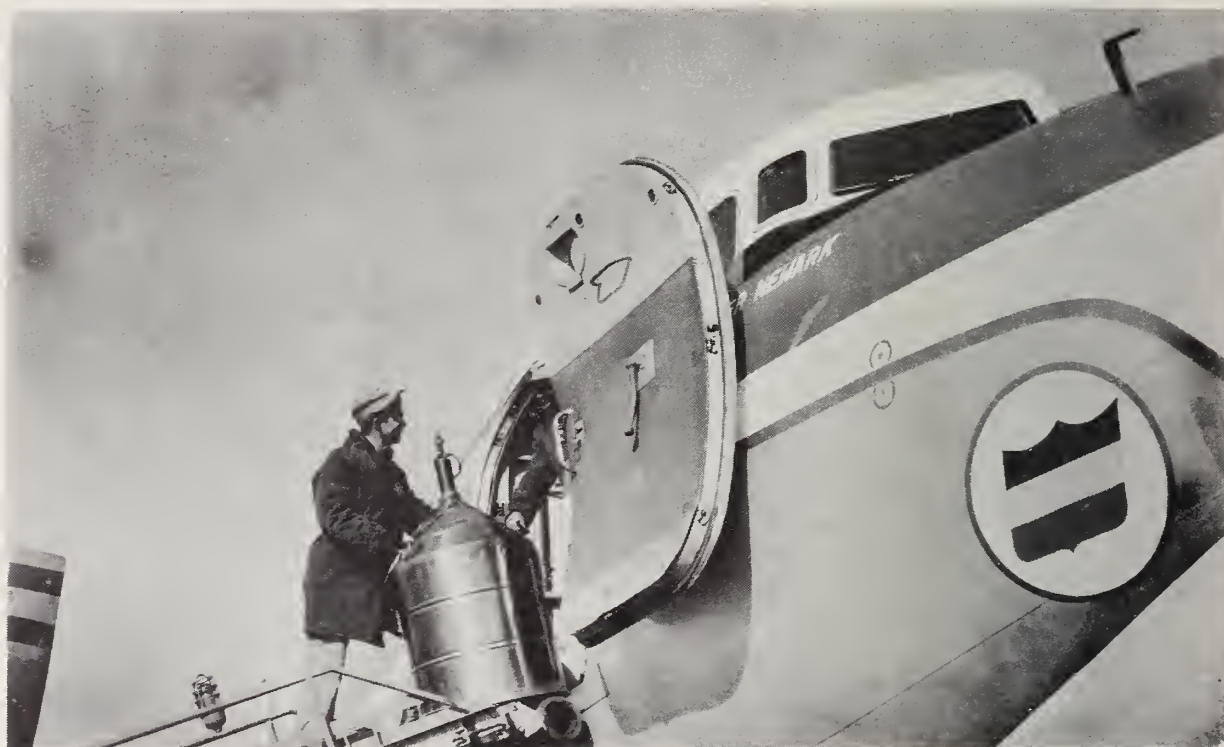
Unloading liquid helium flown 1,700 miles from Denver to Washington. Over 90 air trips have been made to supply the Bureau's Washington laboratories with helium liquefied at the Boulder (Colo.) Laboratories (page 108).
