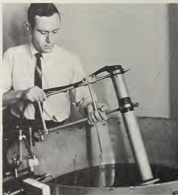
Improvements were made in standards of radioactivity (page 44). Left: A radiation balance is used to measure the rate of energy emission from a radium source used in preparing the new 10^{-9} and 10^{-11} g radium solution standards. Right: Tank of manganese sulfate used as a moderator in calibrations of the National Standard Photoneutron Source.
