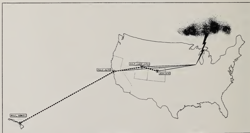
Chain of stations used in a study of the radio waves originating in lightning flashes. Broadband receiving equipment is used to record the signals in a study of the attenuation of low- and very-low-frequency radio waves (page 83).
