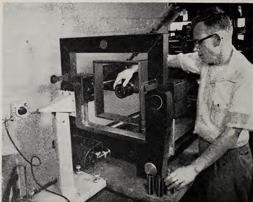
Model of millimeter-wave interferometer being used to investigate applications to the measurement of the velocity of light, to metrology, and to dielectrometry (page 94).
