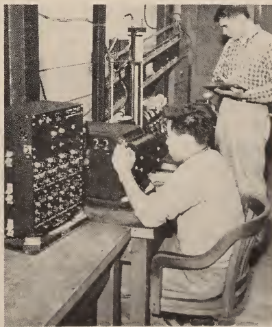
Experimental setup (left) for studying natural wind vibration of telephone wires, which causes a majority of the line failures in the country's wind belt. Right: Instruments for making wind-velocity measurements in wind-tunnel tests of the same phenomena (page 43).
