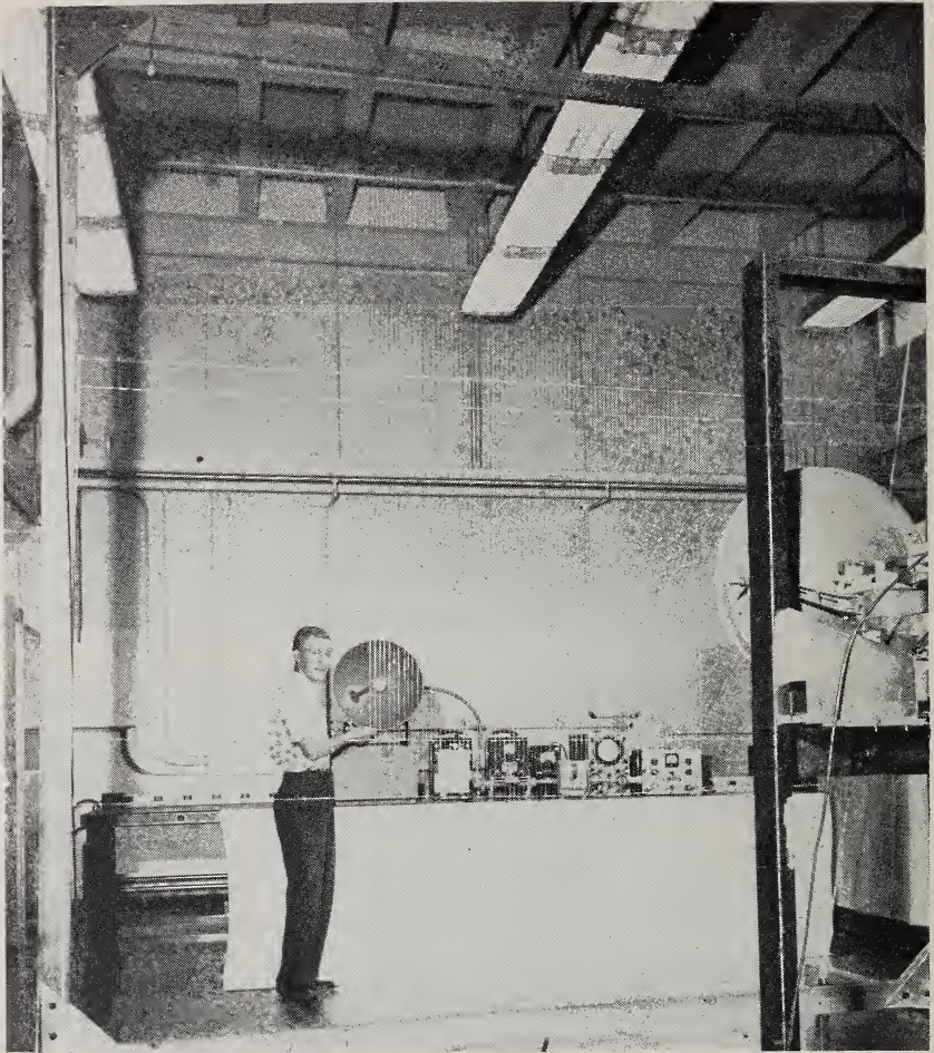
Equipment for measuring microwave energy transmitted through a parallel-wire grid. The known properties of the grid provide a reference for use in studying radio attenuation in various materials (page 89).
