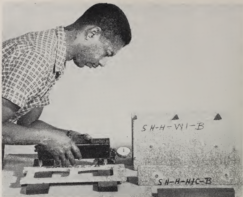
An improved method for determining the drying shrinkage of concrete masonry is being studied. The shrinkage of a thin lamina (left) was found to correlate well at a relative humidity of 30 percent with that of the full-sized blocks (right), and can be measured in a much shorter time (page 67).
