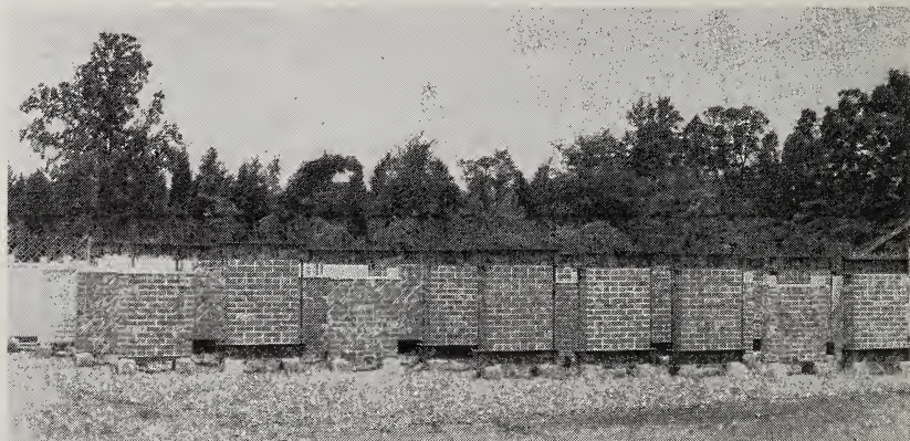
Field test of the dimensional stability of brick walls constructed with mortars containing various dolomitic limes. The results are being correlated with those of a laboratory autoclave expansion test of the lime constituent to determine the suitability of the autoclave test for masonry lime specifications. This program is carried on in cooperation with the National Lime Association, (page 110).
