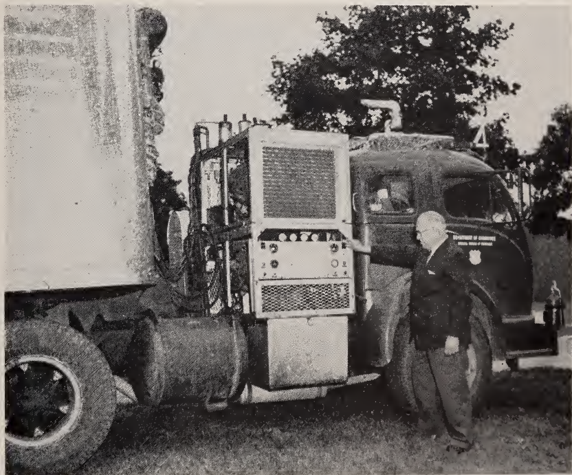
Specially equipped tractor used to develop standard test methods for determining the heat transfer and air-moisture leakage of refrigerated trailers (page 65).
