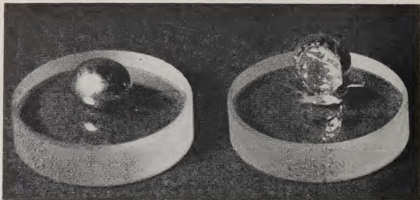
Gold pellets fused on silica plaques in a high-temperature furnace are used to study the strength of ceramic-metal bonds. When the pellet was sheared from the silica surface (right), fracture occurred in the glass rather than at the interface, showing good bond strength (page 61).
