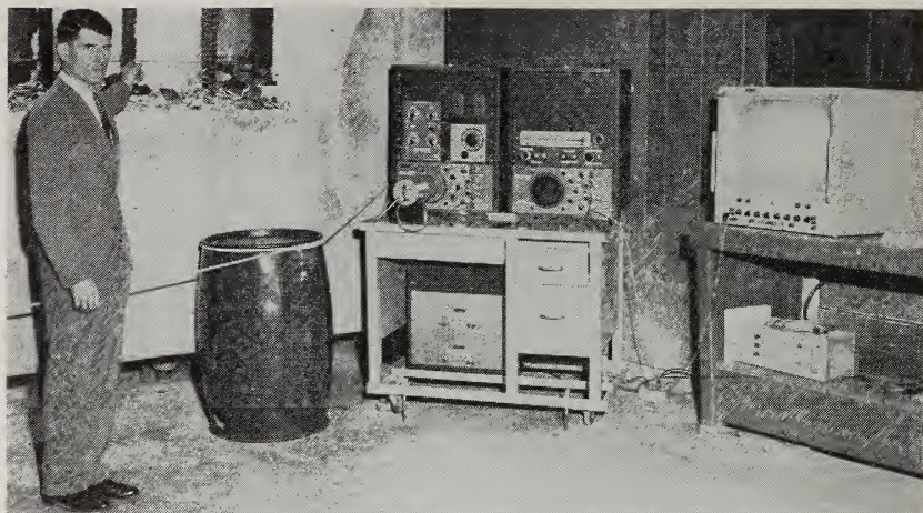
Transient heat-flow analyzer designed to eliminate costly large-scale fire tests by analyzing data about thermal properties of materials (p. 65).
