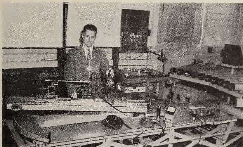
Precision equipment for making exacting determinations of the optical characteristics of aerial camera lenses (p. 20). These factors are very important in photogrammetry, the science of making maps from airplane photographs.
