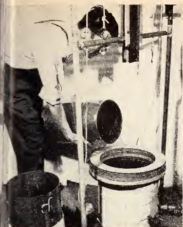
Left: sheet of aircraft glazing, stretch-formed in the shape of a hat, is removed from vacuum forming vessel (p. 38). Right: apparatus used for determining the bursting strength of leather (p. 37). Plungers used in the tests are on the machine panel.
