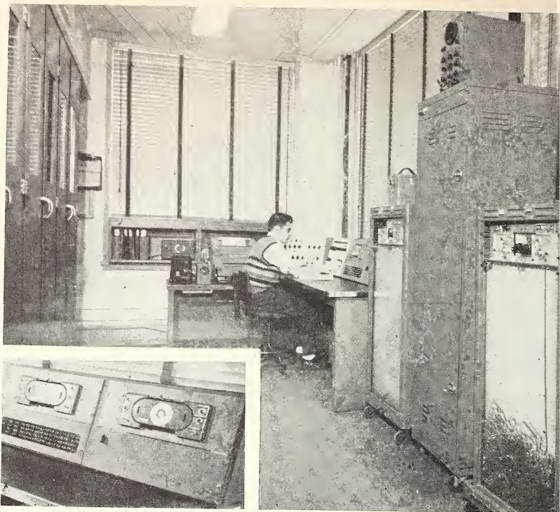
SEAC operates on a 24-hour day, 7 days a week (p. 64). New reel-less magnetic tape external memory devices (right and center) which have unusually fast access time (p. 64). Insert: for loading and unloading the computer very rapid magnetic wire cartridges were installed (p. 64).
