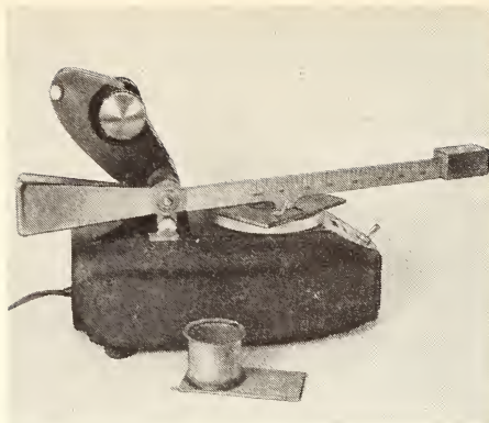
Left: resistance of various floor coverings to effects of grease, oils, alkalis, and other reagents is determined by scratching exposed specimens with sharp tool (under the gram mark). Width of the scratch gives measure of resistance of various coverings to different reagents (p. 48). Right: concrete cylinder (bottom center) set up for impact testing with drop hammer (p. 48).
