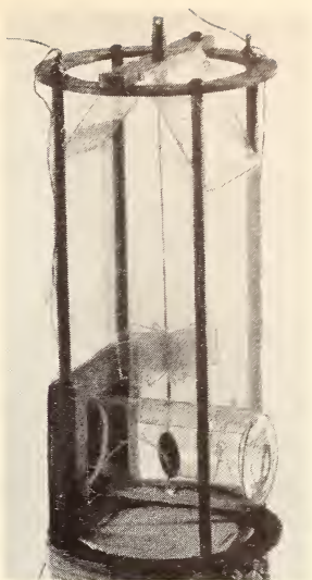
Left: Thermal Raleigh disk apparatus developed by NBS for the study of second sound and the properties of liquid helium II near absolute zero (p. 26). The new technique measures the torque exerted on a light disk (right) by standing waves of second sound set up within a resonant cavity.
