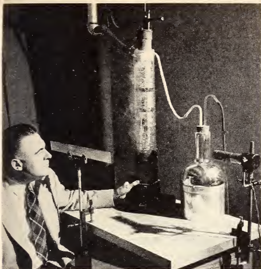
Left: Thermal Raleigh disk apparatus developed by NBS for the study of second sound and the properties of liquid helium II near absolute zero (p. 26). The new technique measures the torque exerted on a light disk (right) by standing waves of second sound set up within a resonant cavity.
