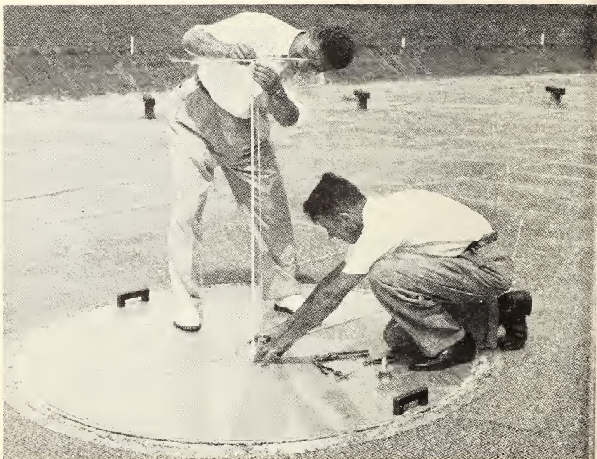
Above: A new model antenna range to facilitate the measurement of antenna radiation patterns in the vertical plane has recently been completed by NBS. Below: Adjusting a test antenna on the new range.
