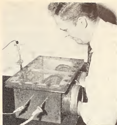
Left: A simple, rapid method was developed for determining the percentage of rubber hydrocarbon in crude natural rubber by measuring the refractive index of a rubber solution (p. 53). Right: For stress-corrosion studies, metal specimens are abraded in an argon atmosphere to remove the film due to atmospheric exposure.
