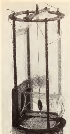
Left: Thermal Raleigh disk apparatus developed by NBS for the study of second sound and the properties of liquid helium II near absolute zero (p. 26). The new technique measures the torque exerted on a light disk (right) by standing waves of second sound set up within a resonant cavity.
