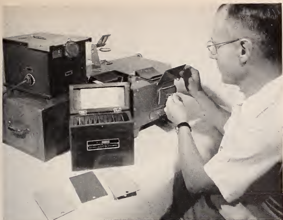
Calibrated chromatic reflectance standards (foreground), covering 10 important commercial colors, are now available from the Bureau for use with photoelectric reflectometers.
