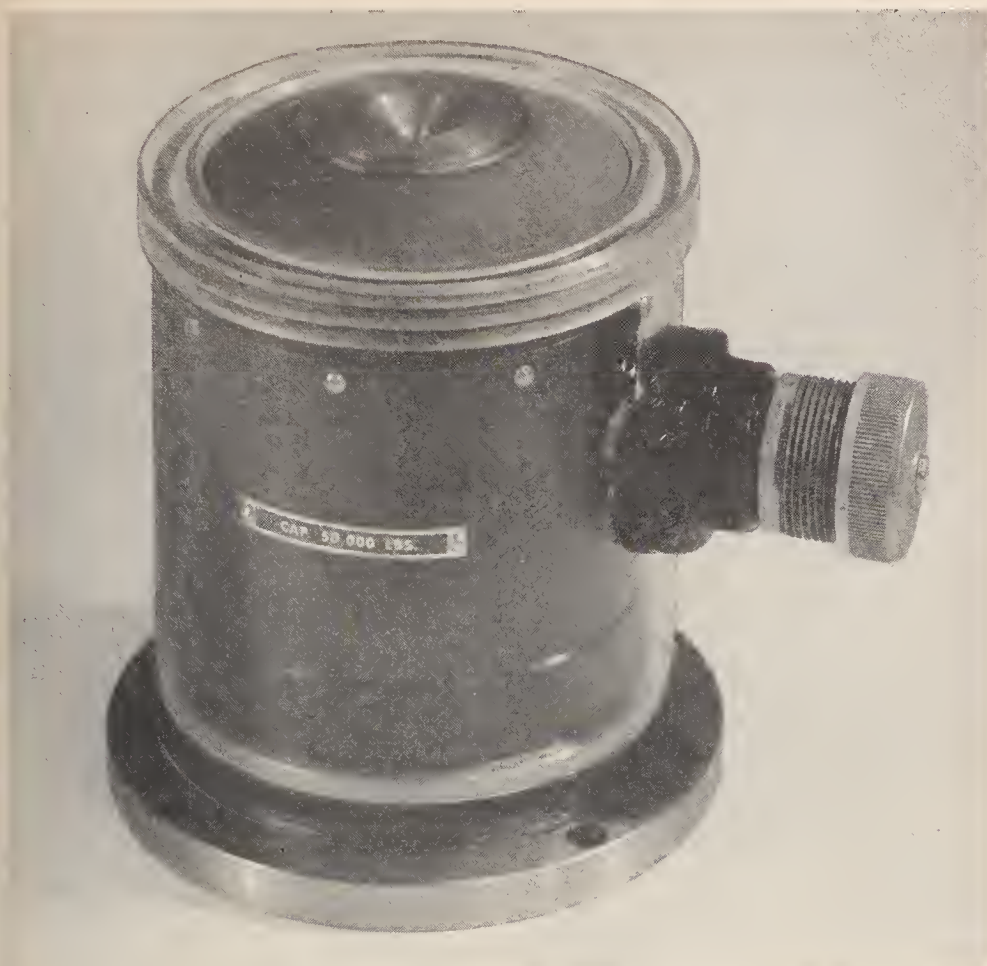
FIGURE 2. Cell used in electronic scale.
