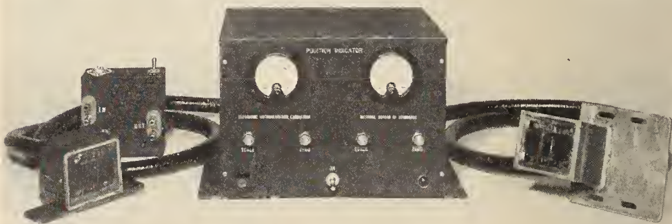
NBS Electronic Position Indicator. This instrument was designed at the Bureau to determine the clearance between rotor and stator blades of propulsion turbines in the USS Coral Sea during actual operating conditions. At left is the channel-selector switch and one of the pick-ups; the other pick-up is shown at right.
