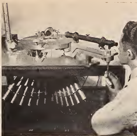
Left: this high-precision spectrometer determines the refractive index of transparent materials used by the Bureau in standardizing industrial refractometers. Right: a new precision camera calibrator recently developed by the Bureau is tested for accuracy (p. 8).
