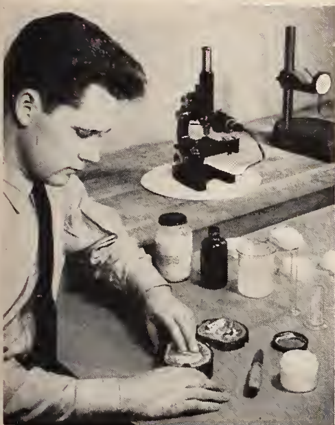
Laboratory studies of the fundamental physical and clinical properties of dental materials are conducted at the Bureau (p. 13). Top: tendencies toward shrinkage in dental amalgam are determined by means of the dental interferometer. Lower left: to obtain data on materials and techniques, experimental dentures are processed under controlled conditions. Lower right: measurement of shrinkage in a plastic denture.
