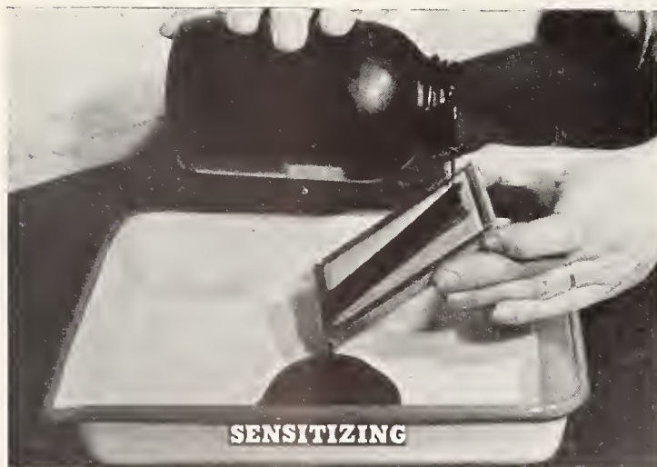
FIGURE 2.4. Steps used in preparing a screen stencil.
