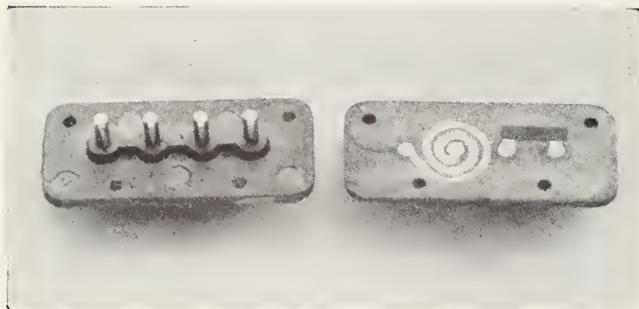
FIGURE 17.4. Printed plug-in unit on a molded Mycalex base plate.
