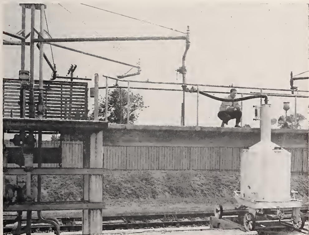
FIGURE 8. Semiportable prover tank, capacity, 500 gallons.
