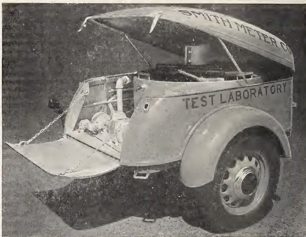
FIGURE 6. Portable test laboratory equipped for recalibration and accuracy tests in customers' plants.
