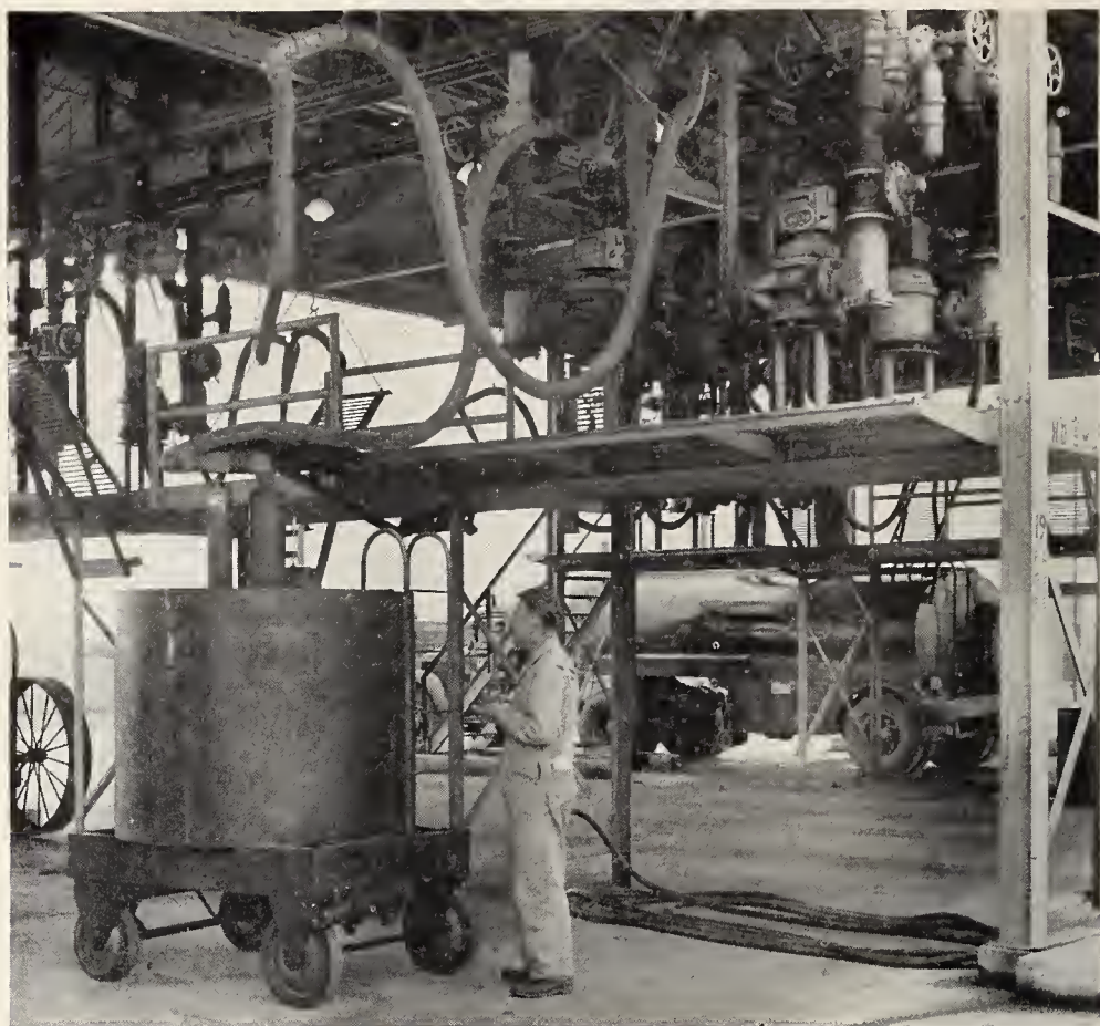
FIGURE 9. 400-gallon prover tank receiving a test delivery.
