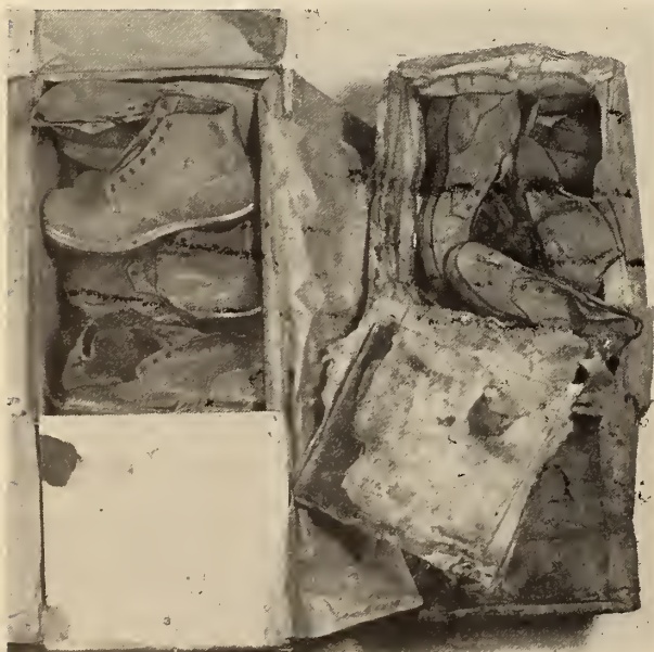
FIGURE 4. Two cases of Army shoes received from storage on the island of Saipan illustrate the importance of packaging.
