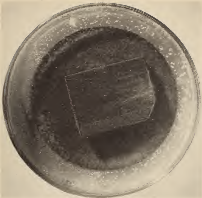
FIGURE 8. Wood treated with inferior fungicide showing growth of Chaetomium globosum when tested by the mycelial mat method.
