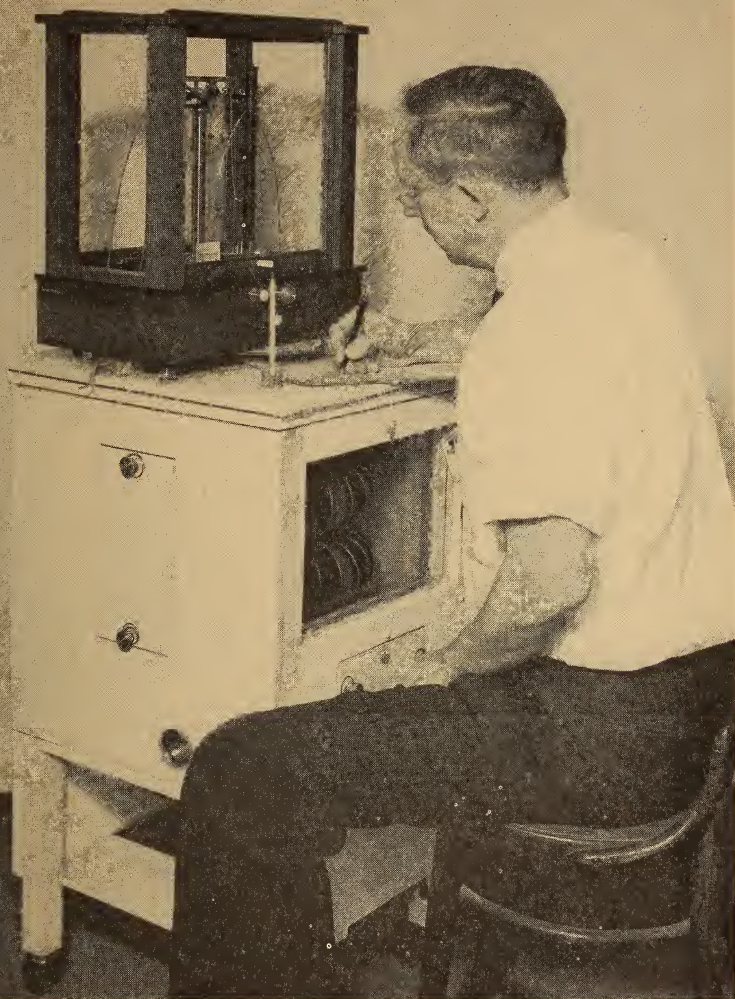
FIGURE 5.— Cabinet for testing for permeability to water and water vapor under tropical conditions.
