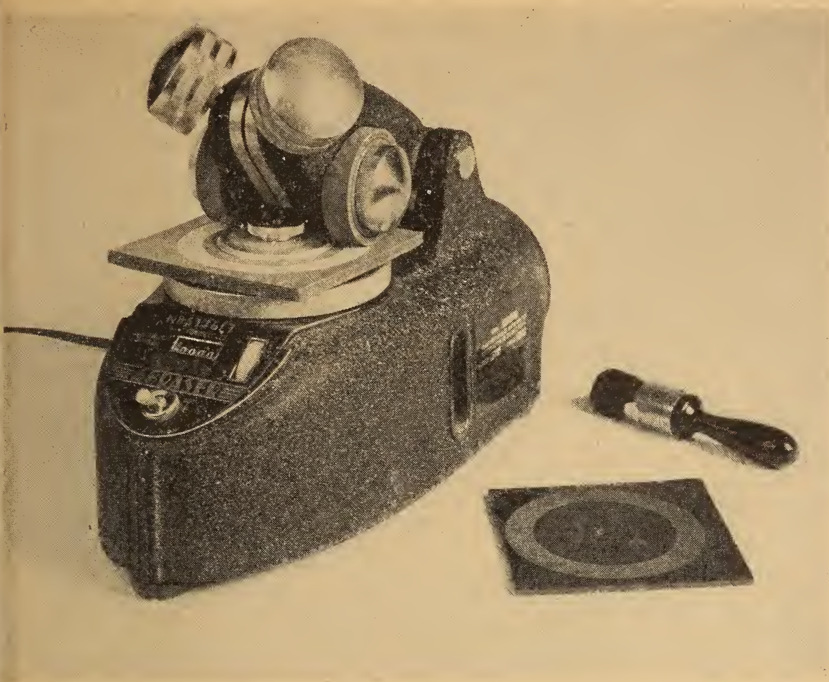
FIGURE 2.—Apparatus used for determining resistance to scuffing of caselining materials when dry.
