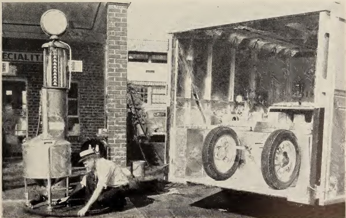
FIGURE 35.— Oregon vehicle-scale testing equipment, showing auxiliary volumetric apparatus.
