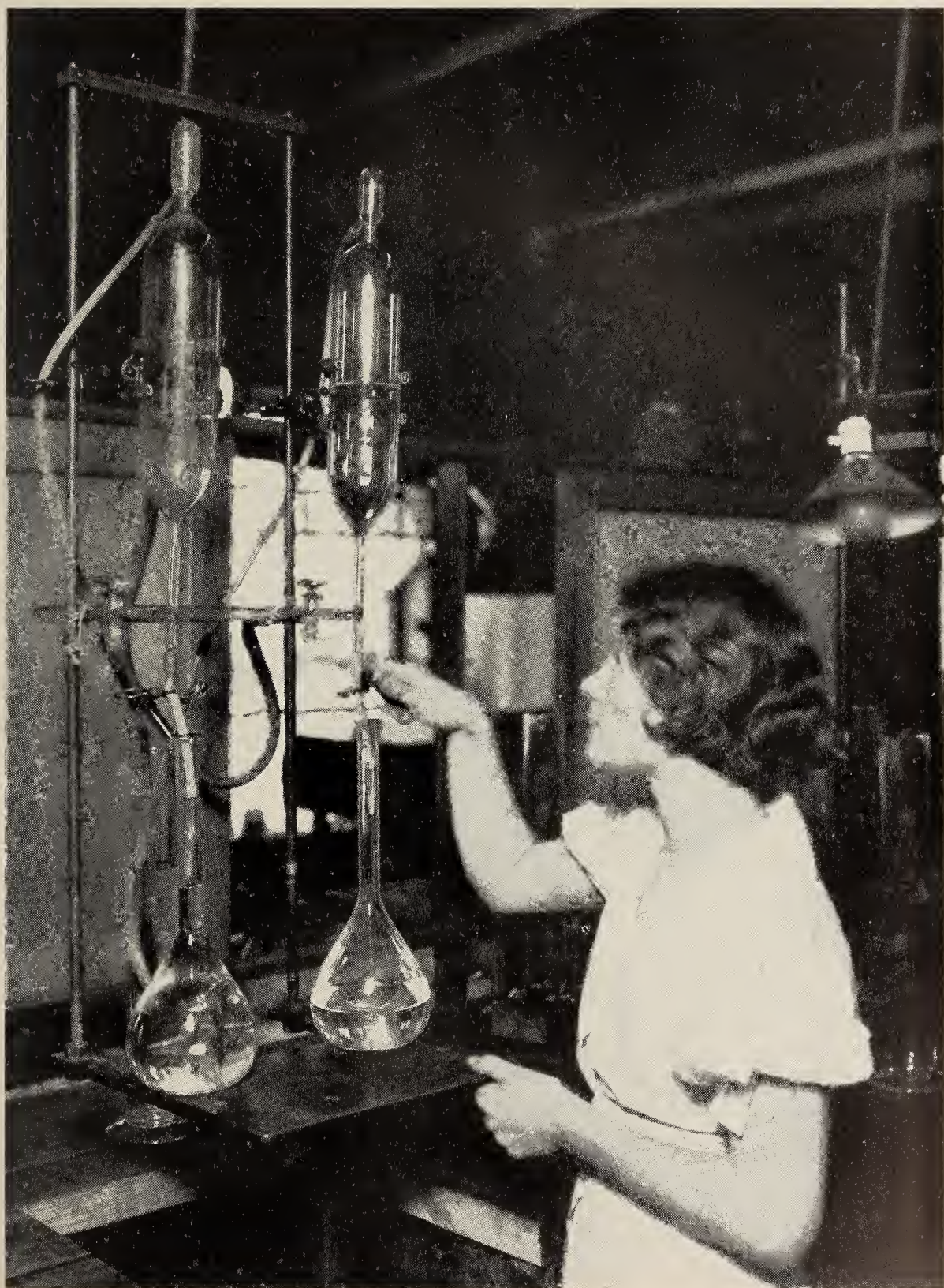
FIGURE 21.— Calibration of measuring flask.
