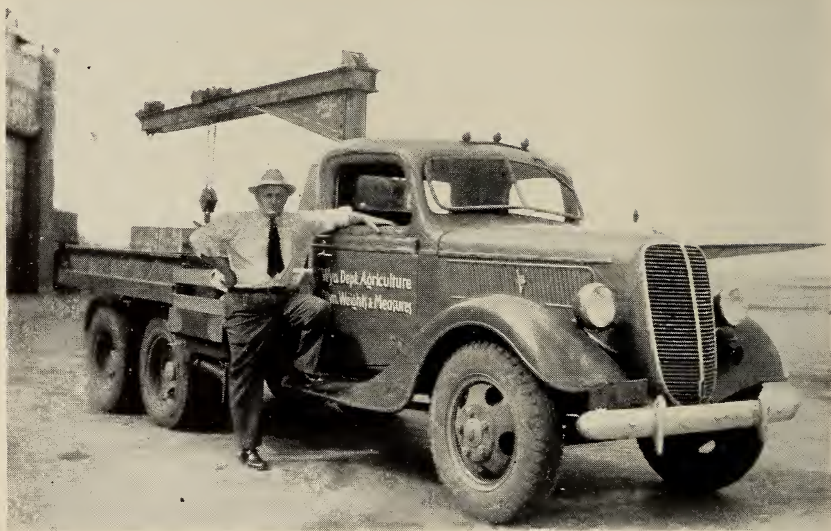
FIGURE 36.— Vehicle-scale testing equipment, State of Wyoming.
