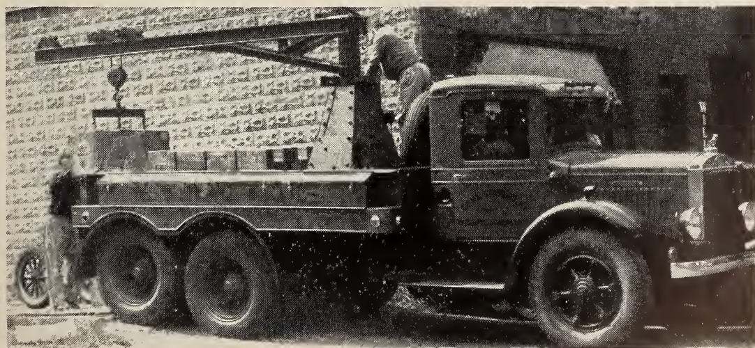
FIGURE 27.— Vehicle-scale testing equipment, State of Connecticut.
